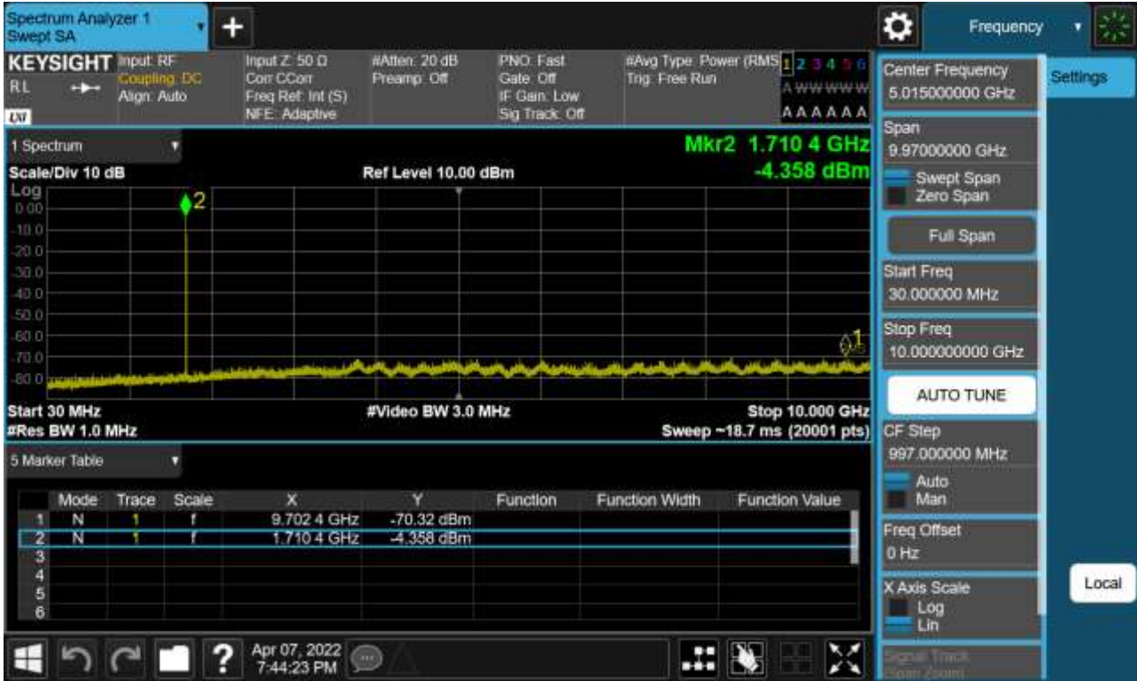
Sub6 n66. Conducted Spurious Plot_1 (342500ch_5 MHz_BPSK_RB 1_1)
