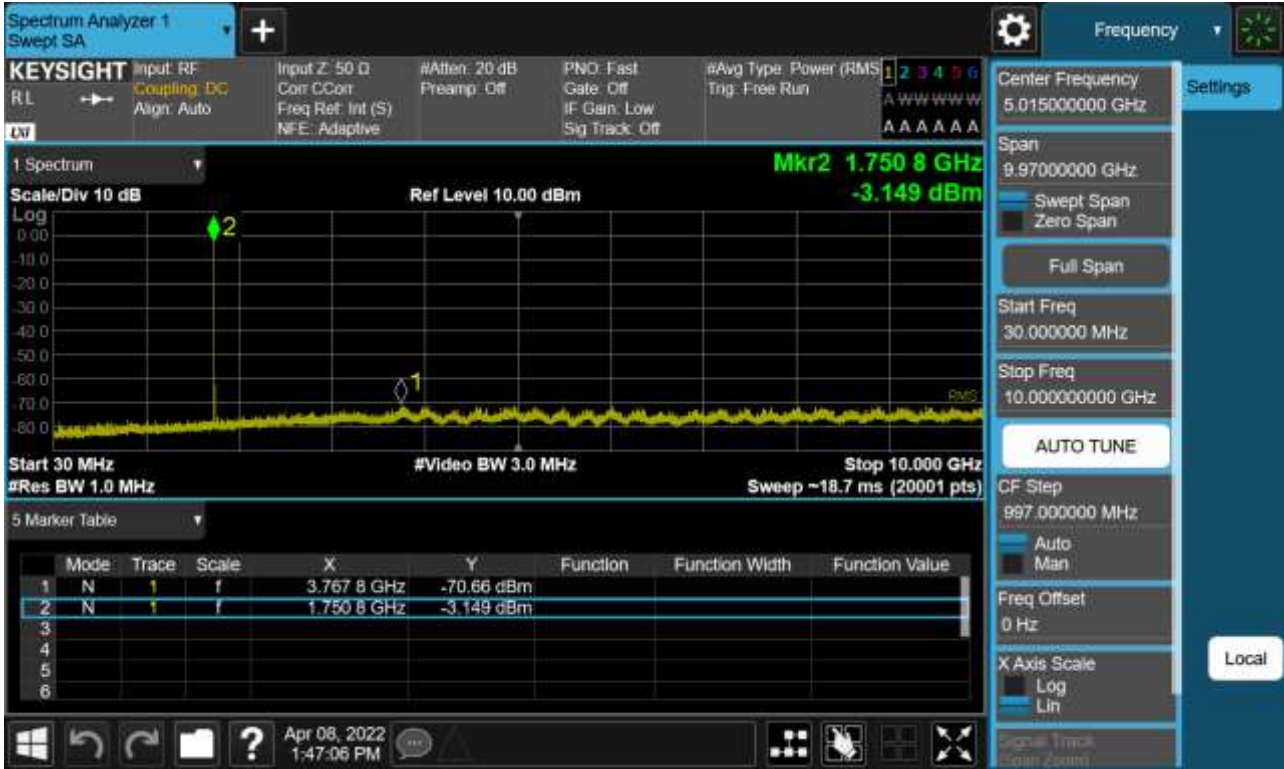
Sub6 n66. Conducted Spurious Plot_1 (353000ch_30 MHz_BPSK_RB 1_1)
