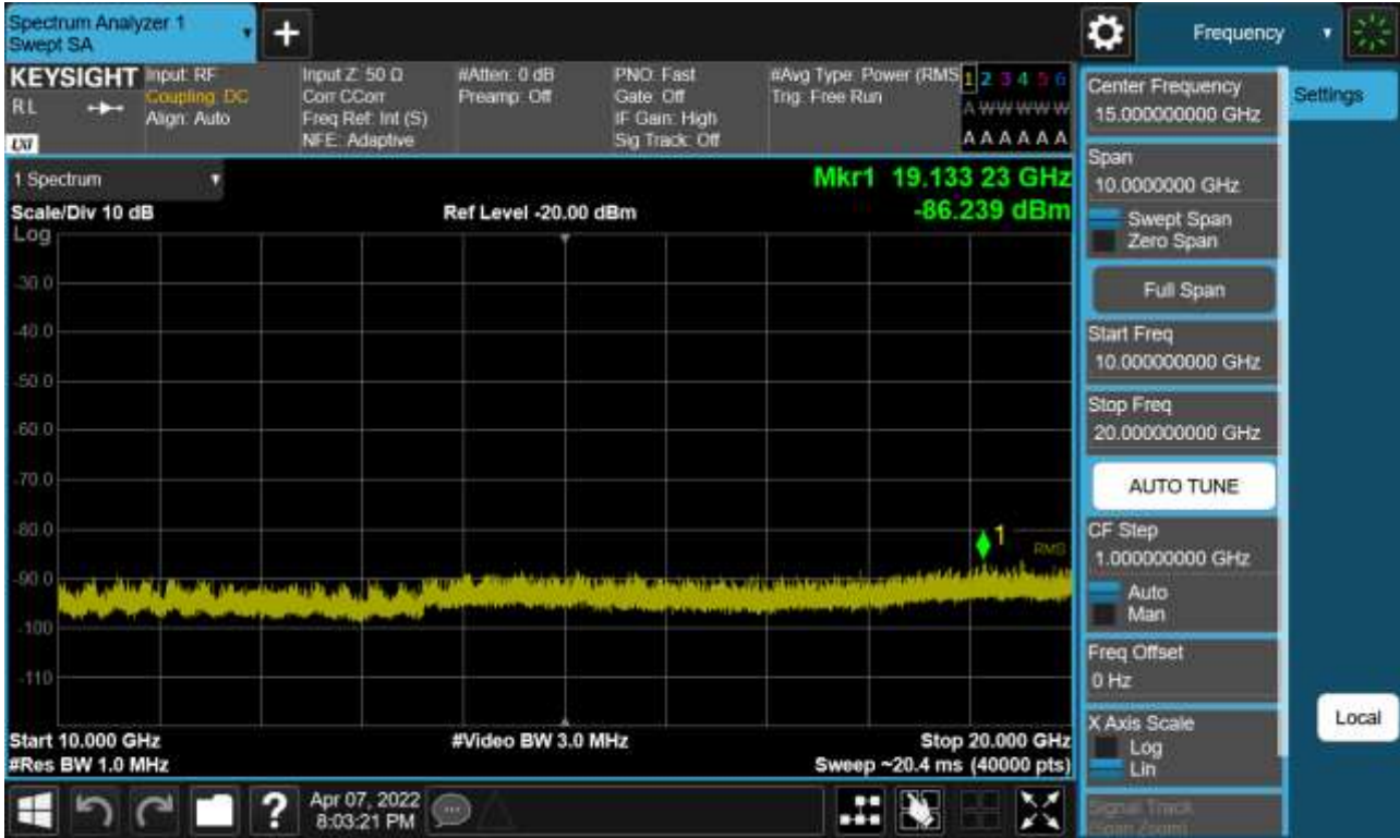
Sub6 n66. Conducted Spurious Plot_2 (355000ch_10 MHz_BPSK_RB 1_1)
