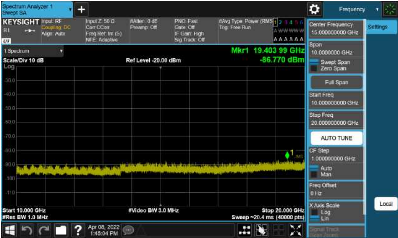
Sub6 n66. Conducted Spurious Plot_2 (349000ch_30 MHz_BPSK_RB 1_1)
