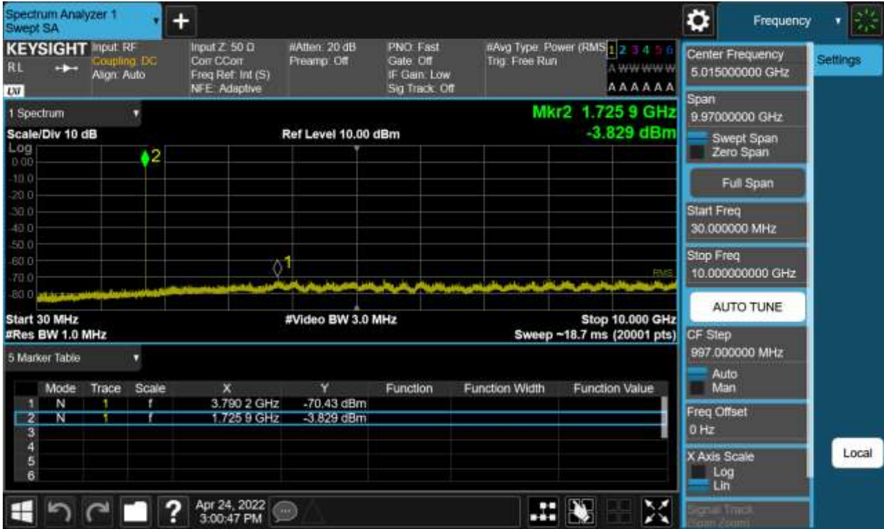
Sub6 n66. Conducted Spurious Plot_1 (349000ch_40 MHz_BPSK_RB 1_1)
