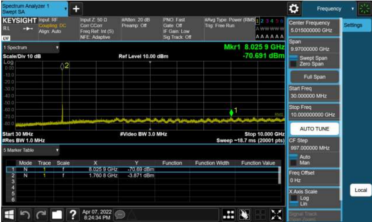
Sub6 n66. Conducted Spurious Plot_1 (354000ch_20 MHz_BPSK_RB 1_1)
