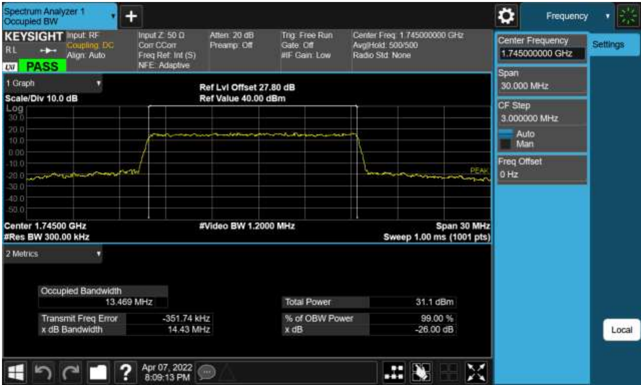
Sub6 n66. Occupied Bandwidth Plot (15 M BW Ch.349000 16QAM Full RB)
