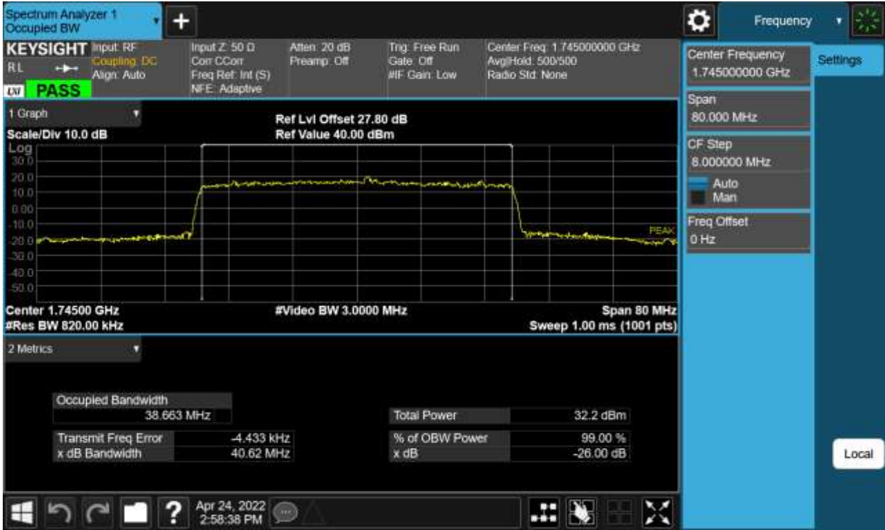
Sub6 n66. Occupied Bandwidth Plot (40 M BW Ch.349000 QPSK Full RB)
