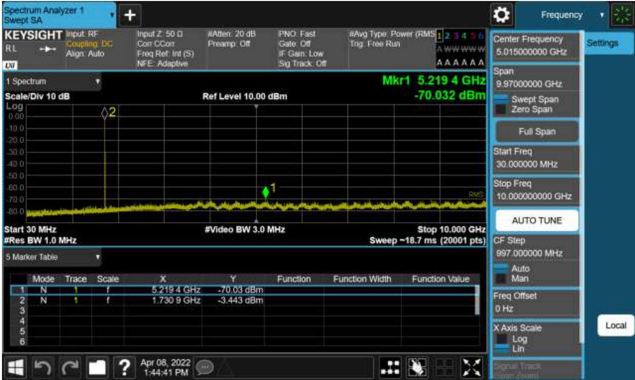
Sub6 n66. Conducted Spurious Plot_1 (349000ch_30 MHz_BPSK_RB 1_1)
