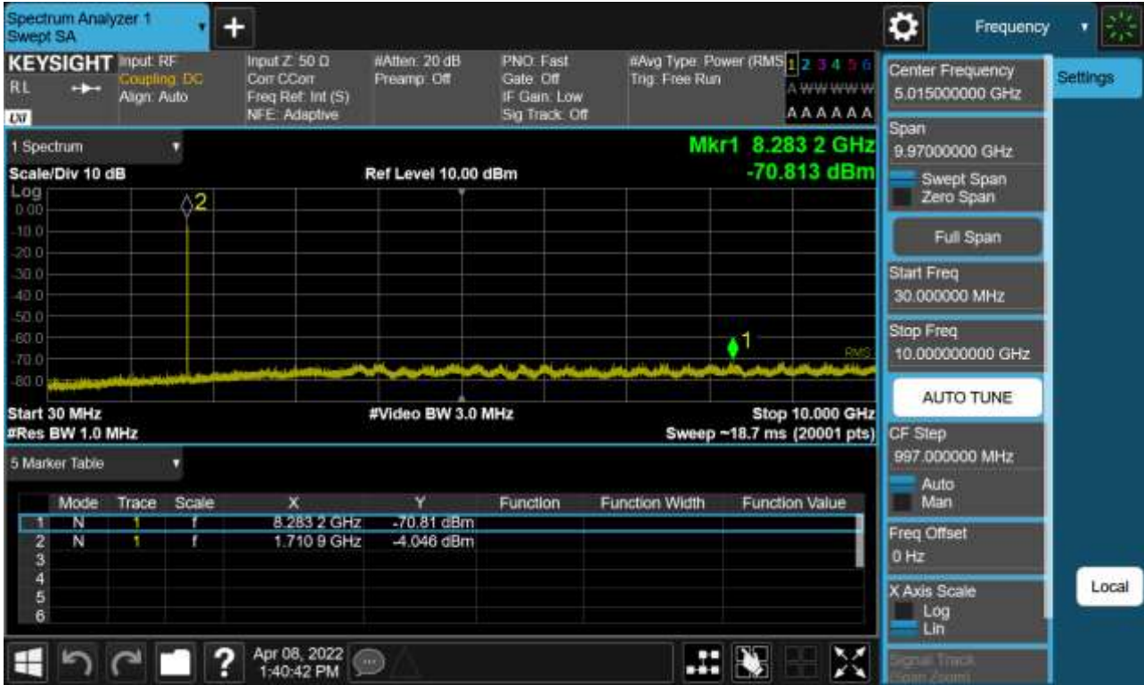
Sub6 n66. Conducted Spurious Plot_1 (345000ch_30 MHz_BPSK_RB 1_1)
