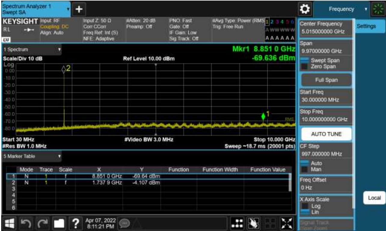
Sub6 n66. Conducted Spurious Plot_1 (349000ch_15 MHz_BPSK_RB 1_1)
