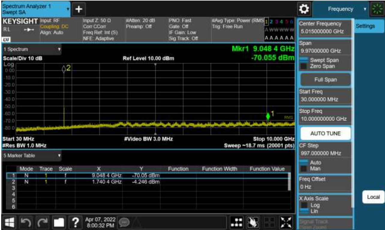
Sub6 n66. Conducted Spurious Plot_1 (349000ch_10 MHz_BPSK_RB 1_1)
