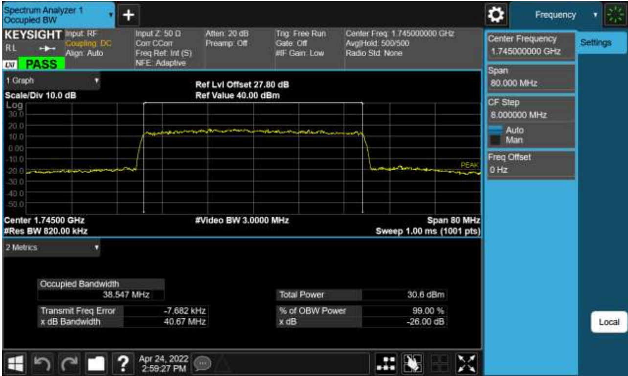
Sub6 n66. Occupied Bandwidth Plot (40 M BW Ch.349000 64QAM Full RB)
