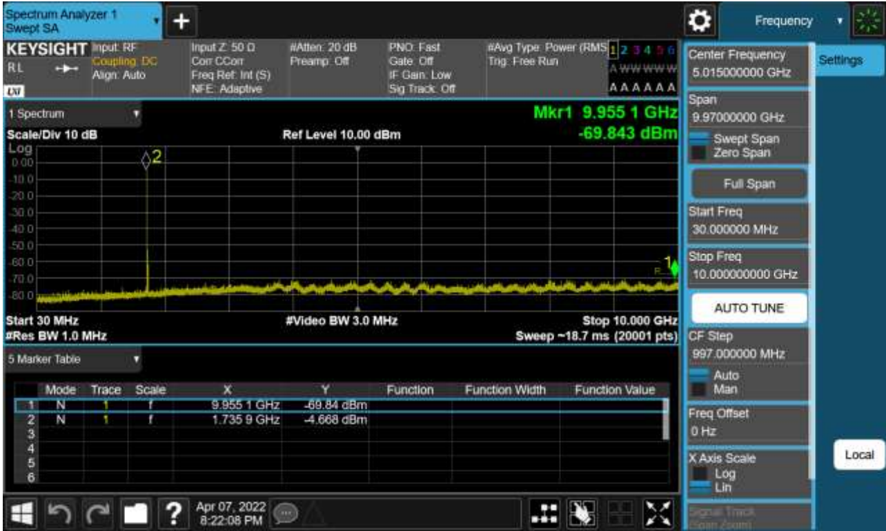
Sub6 n66. Conducted Spurious Plot_1 (349000ch_20 MHz_BPSK_RB 1_1)
