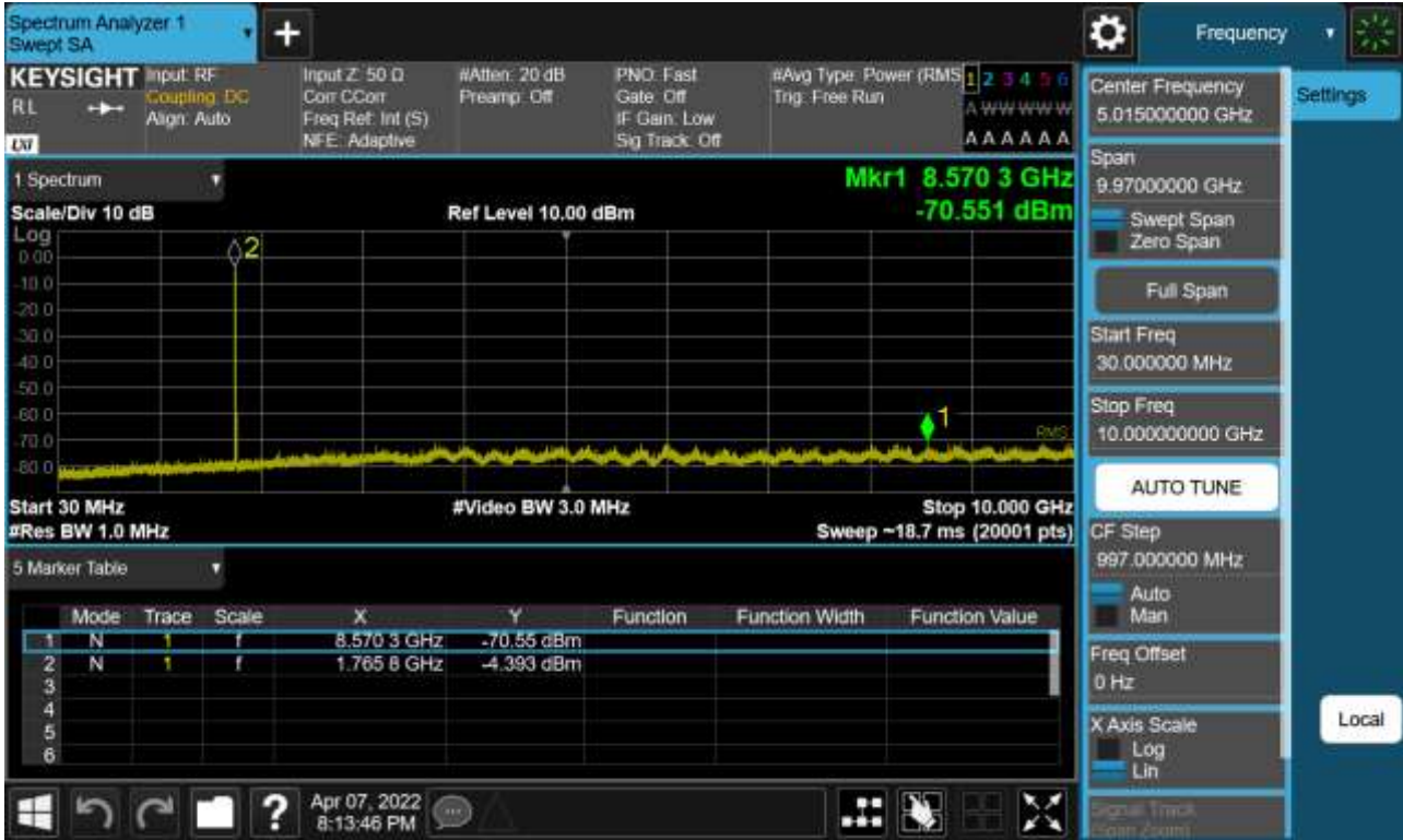
Sub6 n66. Conducted Spurious Plot_1 (354500ch_15 MHz_BPSK_RB 1_1)
