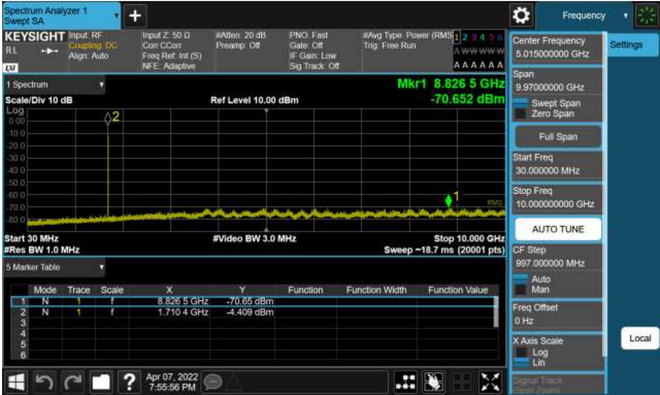
Sub6 n66. Conducted Spurious Plot_1 (343000ch_10 MHz_BPSK_RB 1_1)
