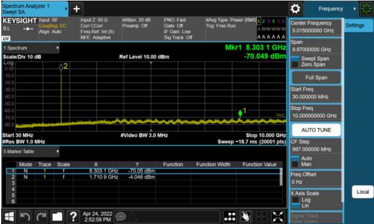
Sub6 n66. Conducted Spurious Plot_1 (346000ch_40 MHz_BPSK_RB 1_1)
