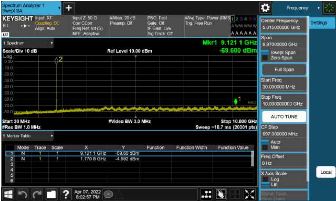
Sub6 n66. Conducted Spurious Plot_1 (355000ch_10 MHz_BPSK_RB 1_1)
