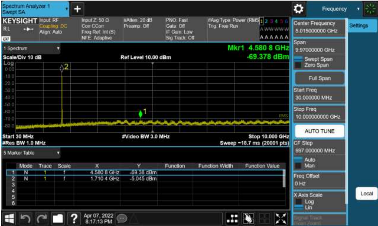
Sub6 n66. Conducted Spurious Plot_1 (344000ch_20 MHz_BPSK_RB 1_1)
