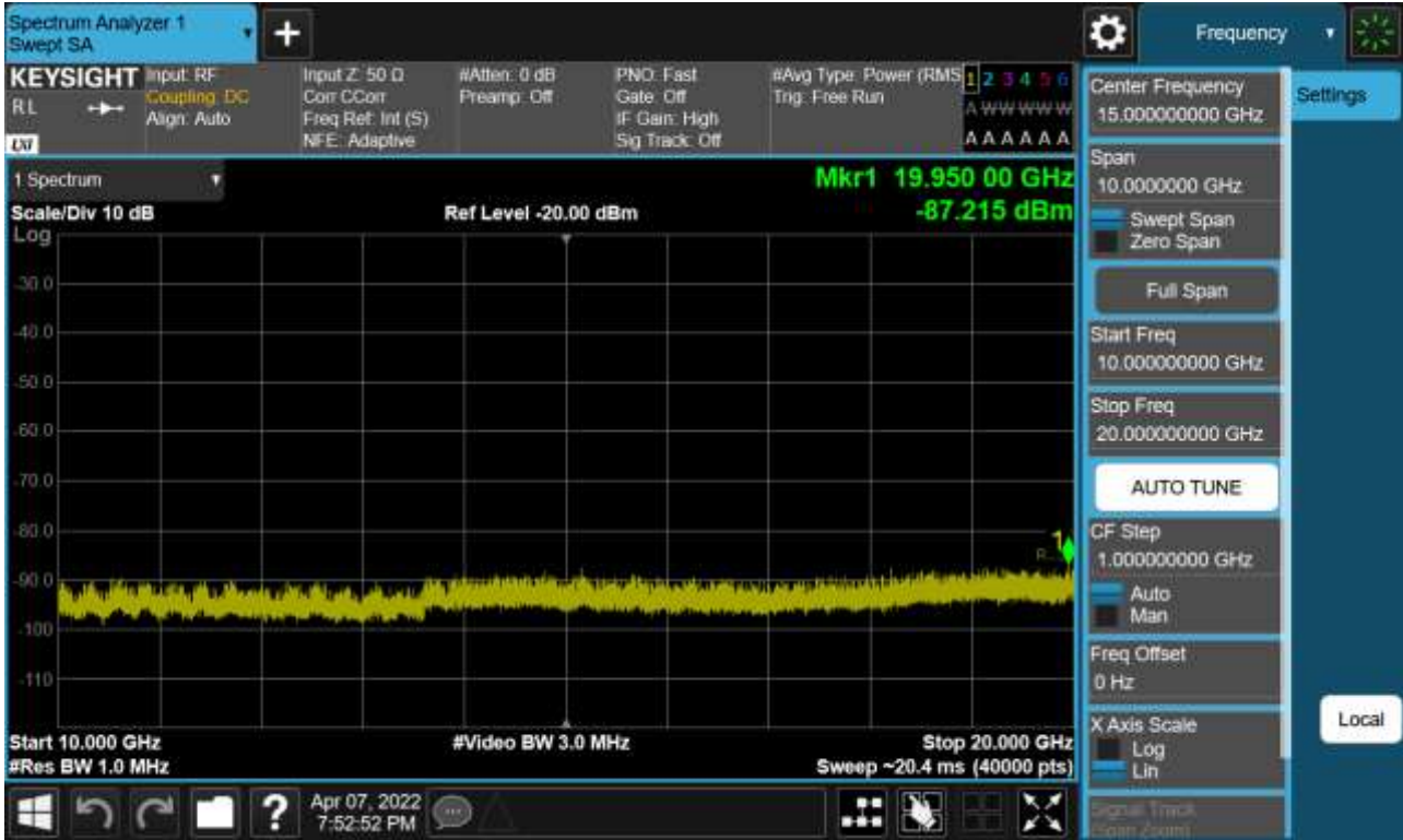
Sub6 n66. Conducted Spurious Plot_2 (355500ch_5 MHz_BPSK_RB 1_1)
