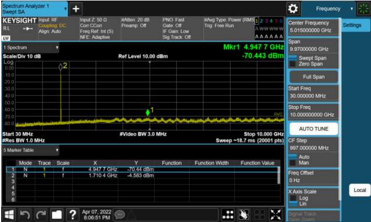
Sub6 n66. Conducted Spurious Plot_1 (343500ch_15 MHz_BPSK_RB 1_1)
