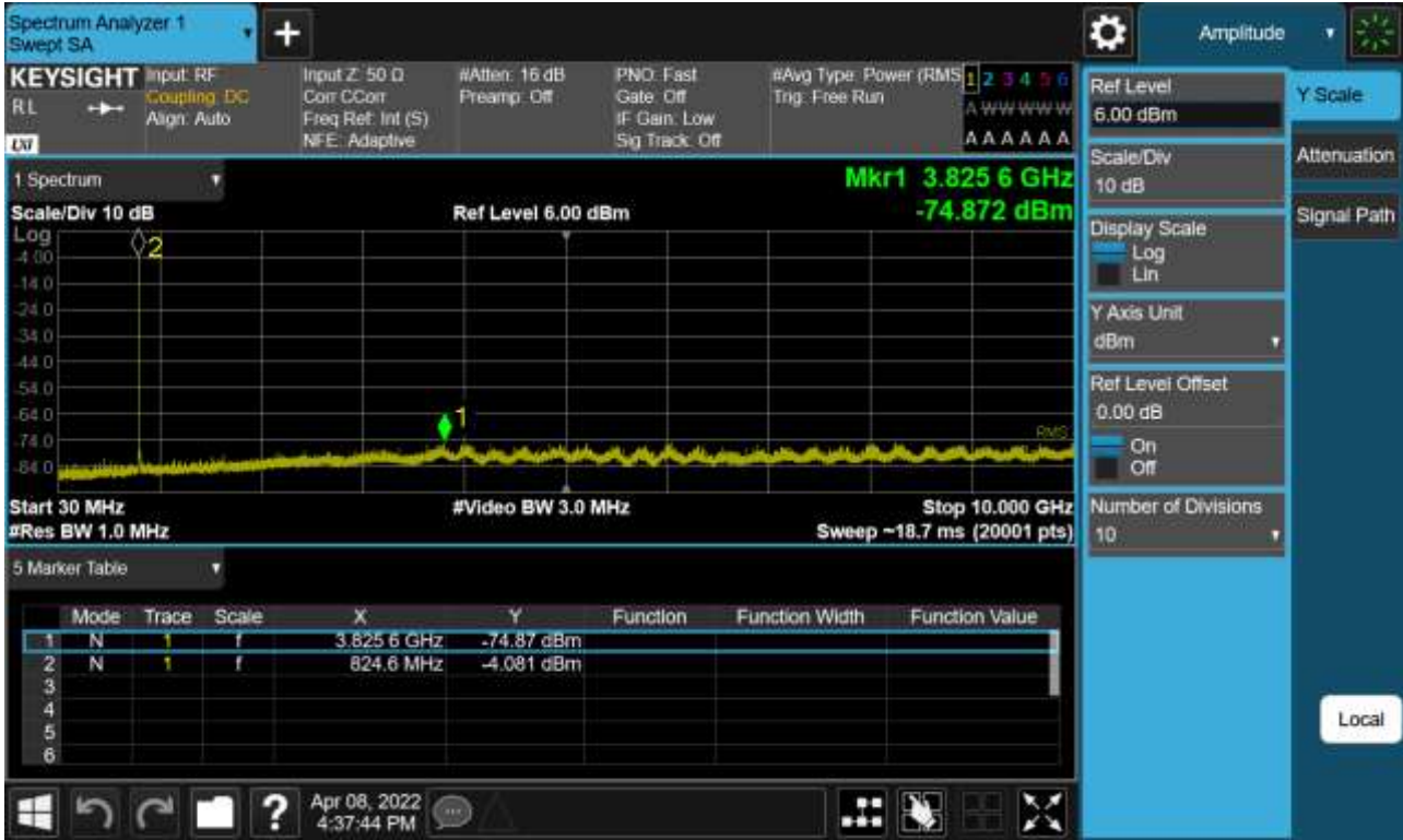
Sub6 n5. Conducted Spurious Plot (166300ch_15 MHz_BPSK_RB 1_1)
