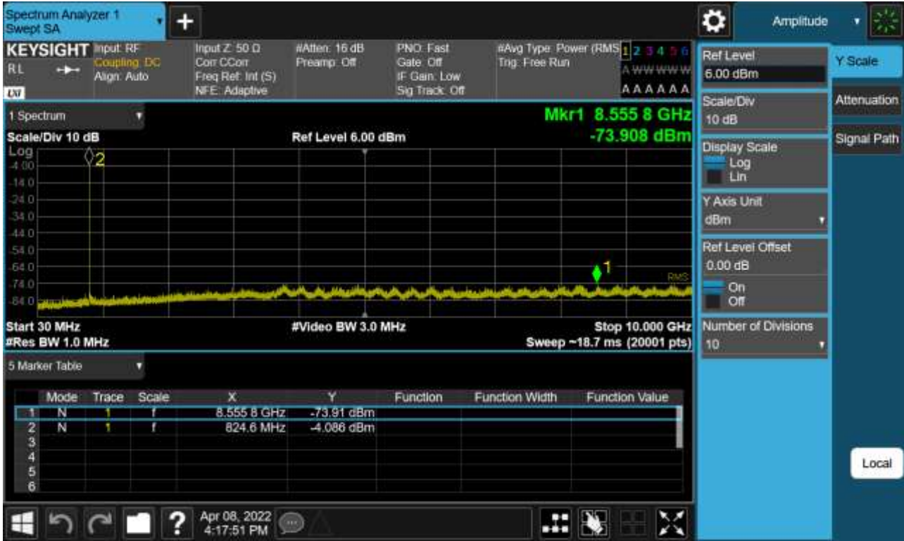
Sub6 n5. Conducted Spurious Plot (165800ch_10 MHz_BPSK_RB 1_1)
