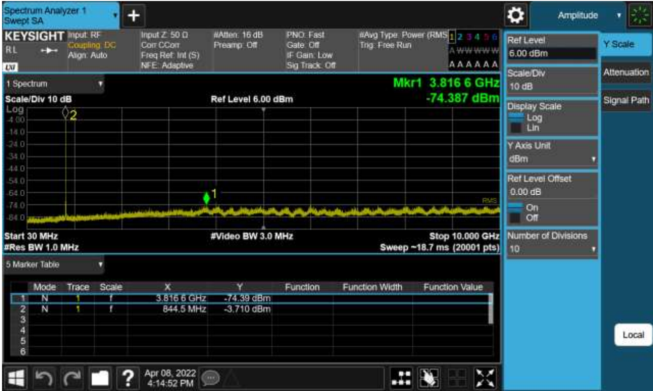
Sub6 n5. Conducted Spurious Plot (169300ch_5 MHz_BPSK_RB 1_1)
