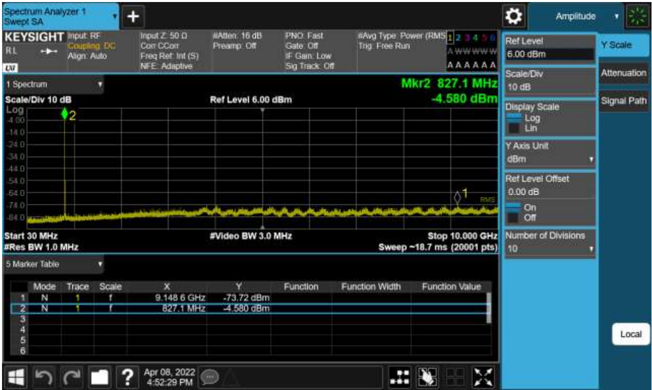
Sub6 n5. Conducted Spurious Plot (167300ch_20 MHz_BPSK_RB 1_1)
