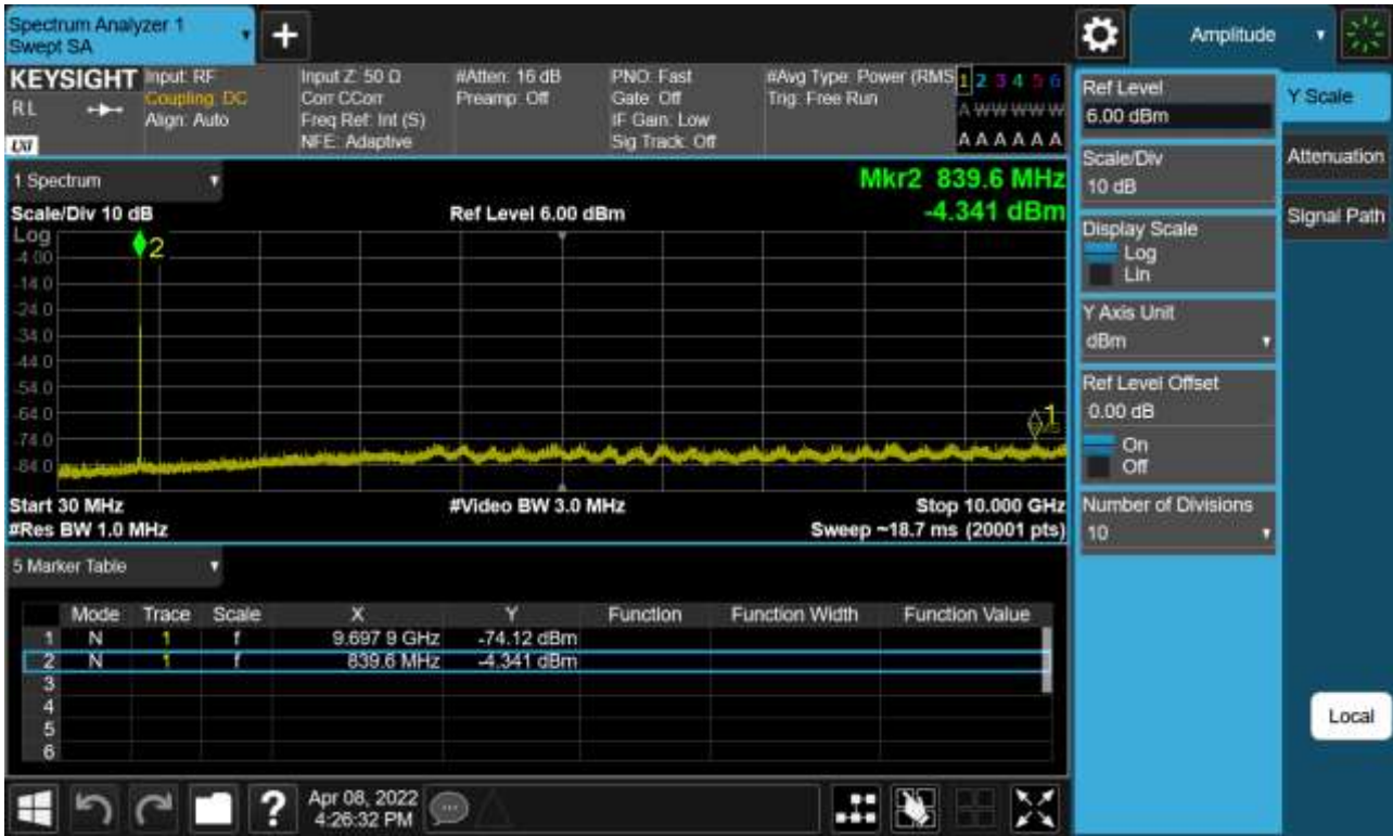
Sub6 n5. Conducted Spurious Plot (168800ch_10 MHz_BPSK_RB 1_1)
