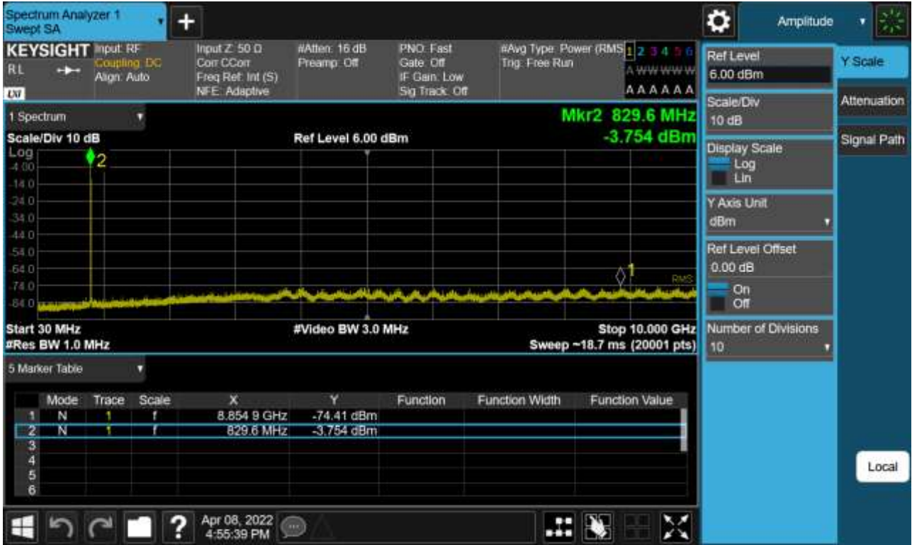
Sub6 n5. Conducted Spurious Plot (167800ch_20 MHz_BPSK_RB 1_1)
