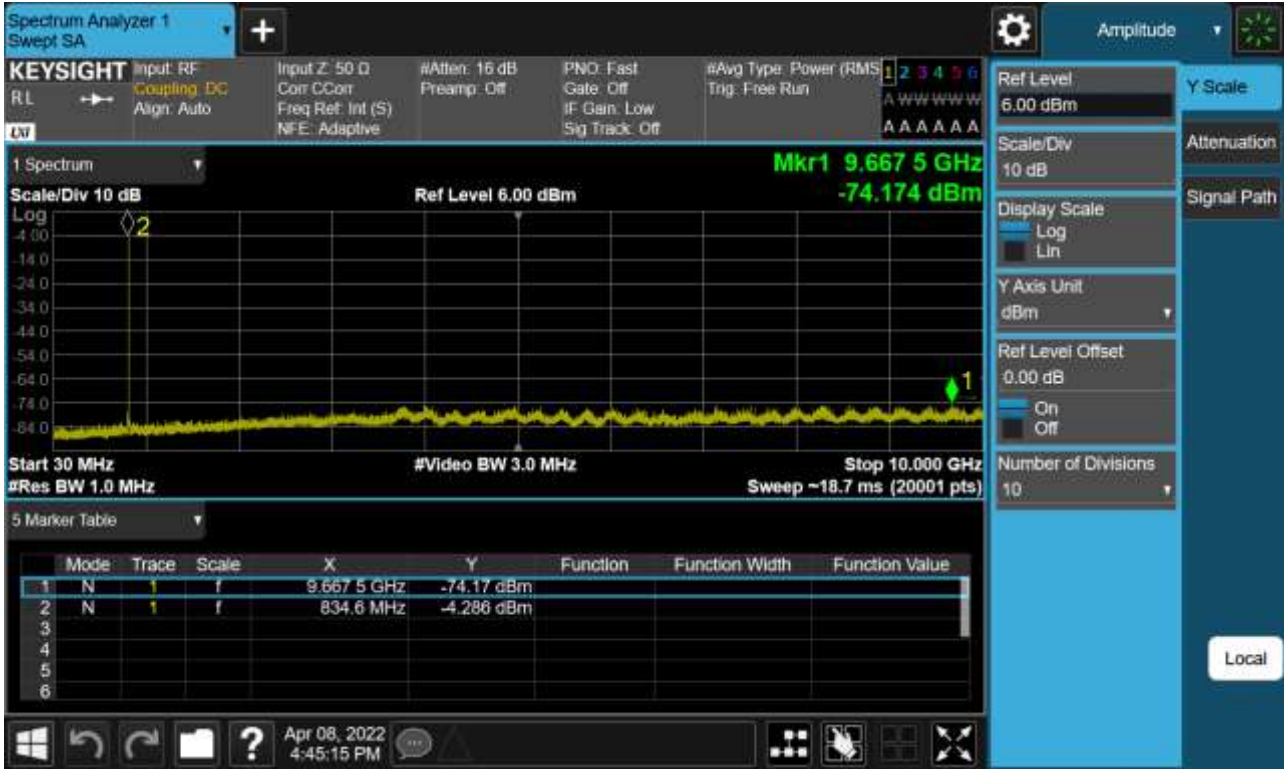
Sub6 n5. Conducted Spurious Plot (168300ch_15 MHz_BPSK_RB 1_1)
