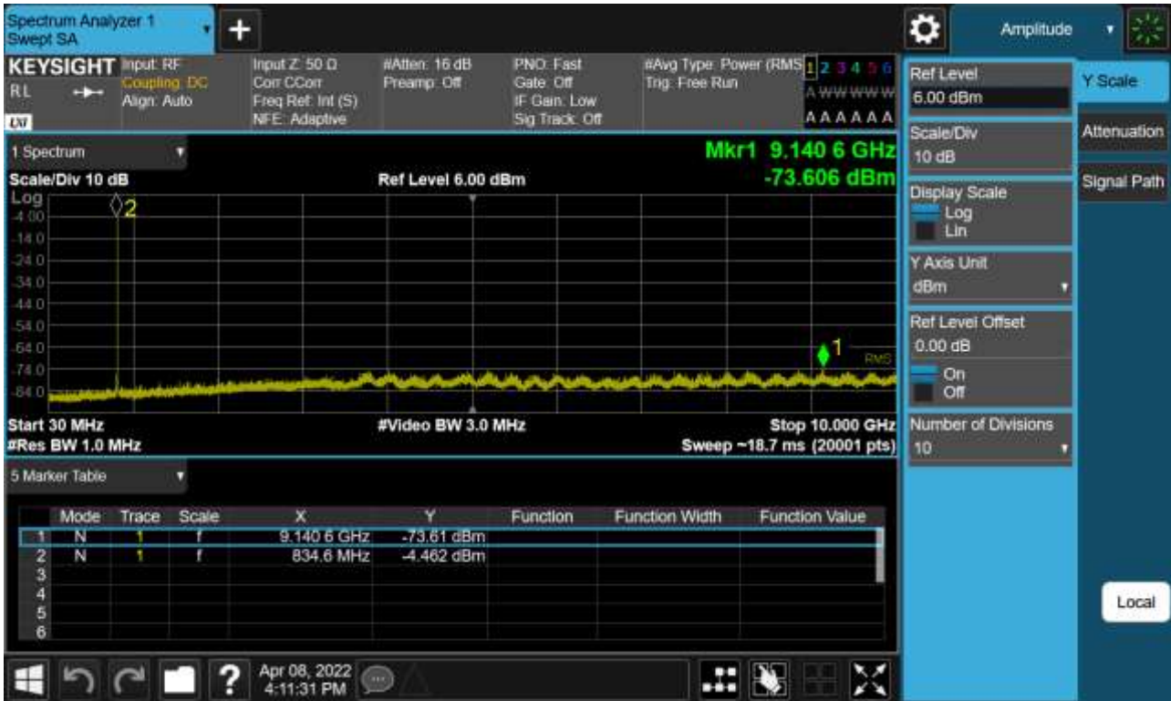
Sub6 n5. Conducted Spurious Plot (167300ch_5 MHz_BPSK_RB 1_1)
