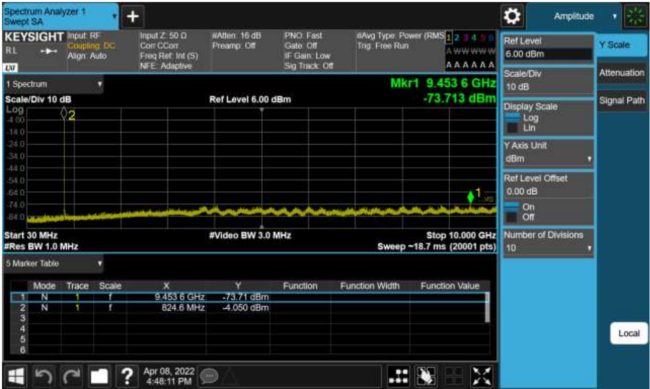
Sub6 n5. Conducted Spurious Plot (166800ch_20 MHz_BPSK_RB 1_1)
