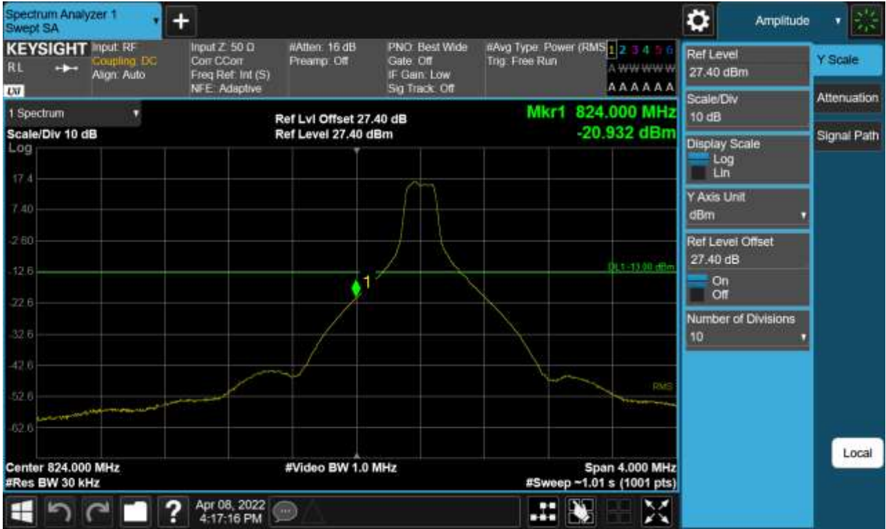
Sub6 n5. Lower Band Edge Plot (10 M BW Ch.165800 BPSK_RB1_Offset 0)
