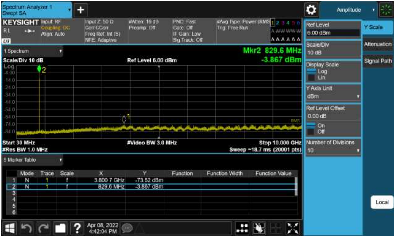
Sub6 n5. Conducted Spurious Plot (167300ch_15 MHz_BPSK_RB 1_1)
