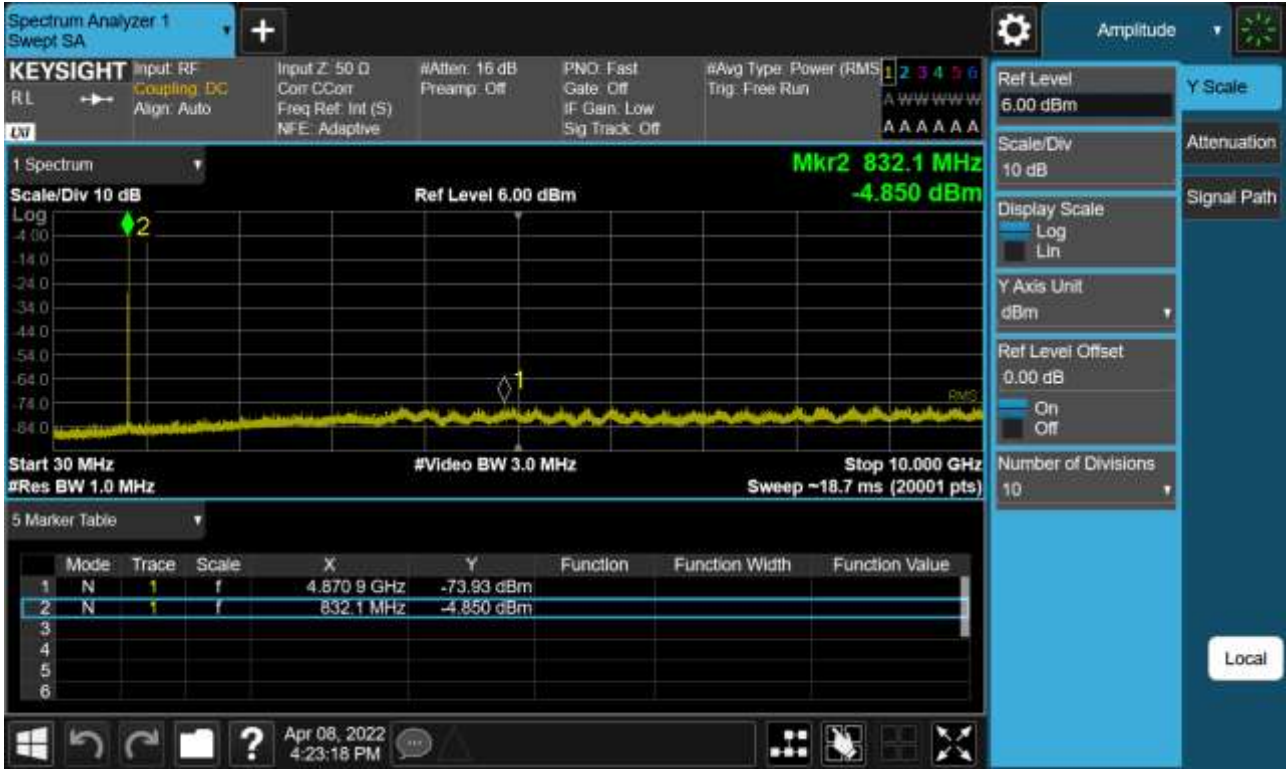
Sub6 n5. Conducted Spurious Plot (167300ch_10 MHz_BPSK_RB 1_1)
