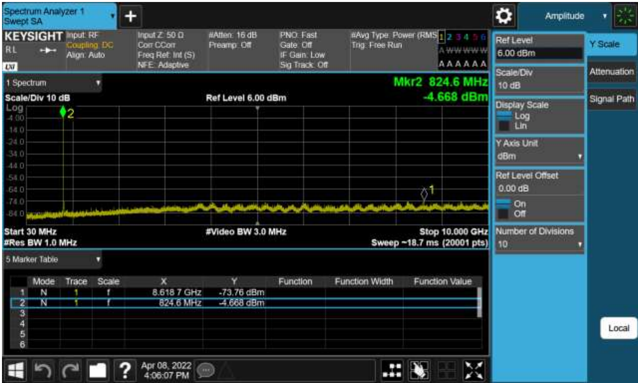
Sub6 n5. Conducted Spurious Plot (165300ch_5 MHz_BPSK_RB 1_1)
