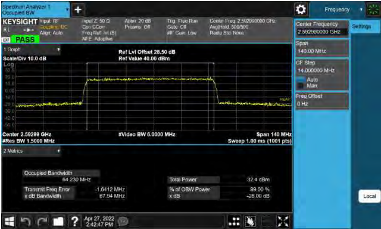
Sub6 n41. Occupied Bandwidth Plot (70 MHz Ch.518598 16-QAM )
