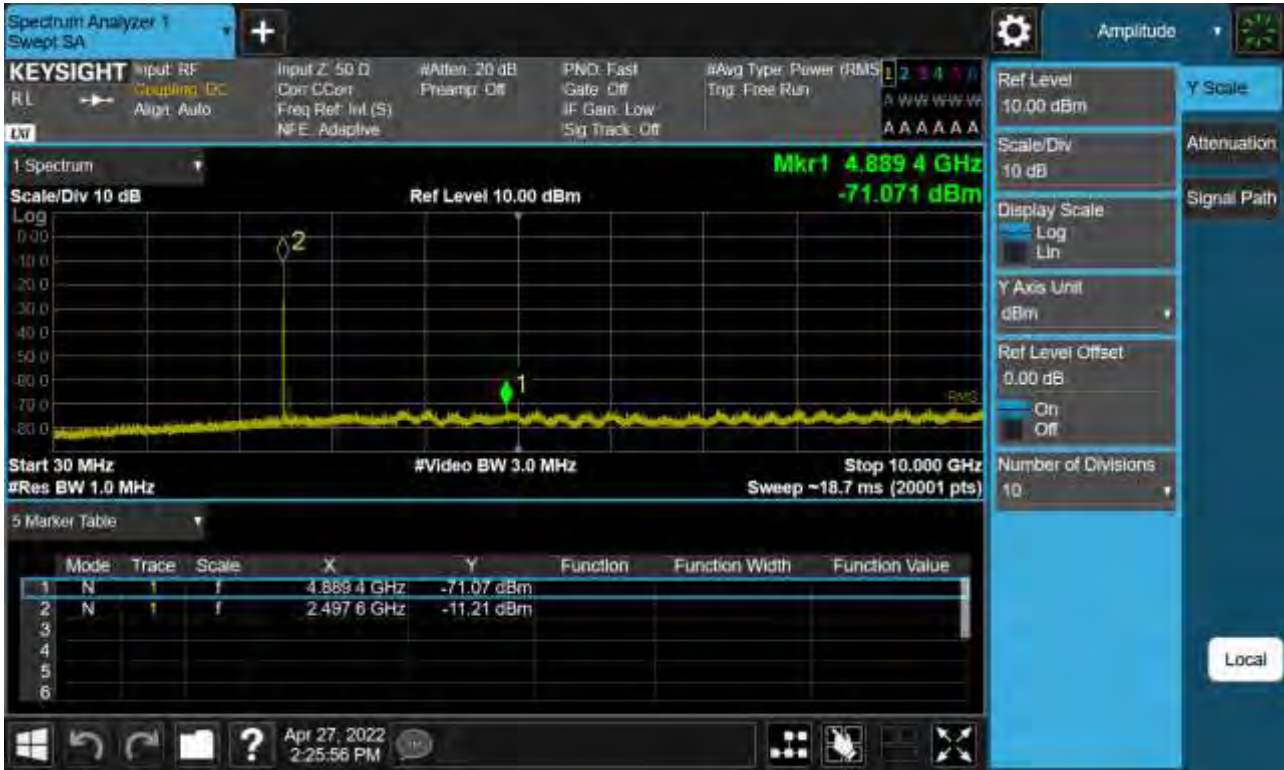
Sub6 n41. Conducted Spurious Plot 1 (60 MHz Ch.505200 BPSK RB 1)
