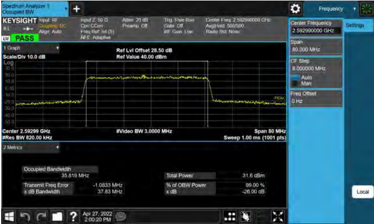
Sub6 n41. Occupied Bandwidth Plot (40 MHz Ch.518598 64-QAM )
