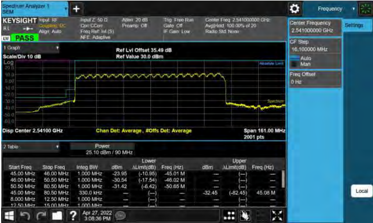
Sub6 n41. Low Channel Edge Plot (90 MHz Ch.508200 BPSK )-1
