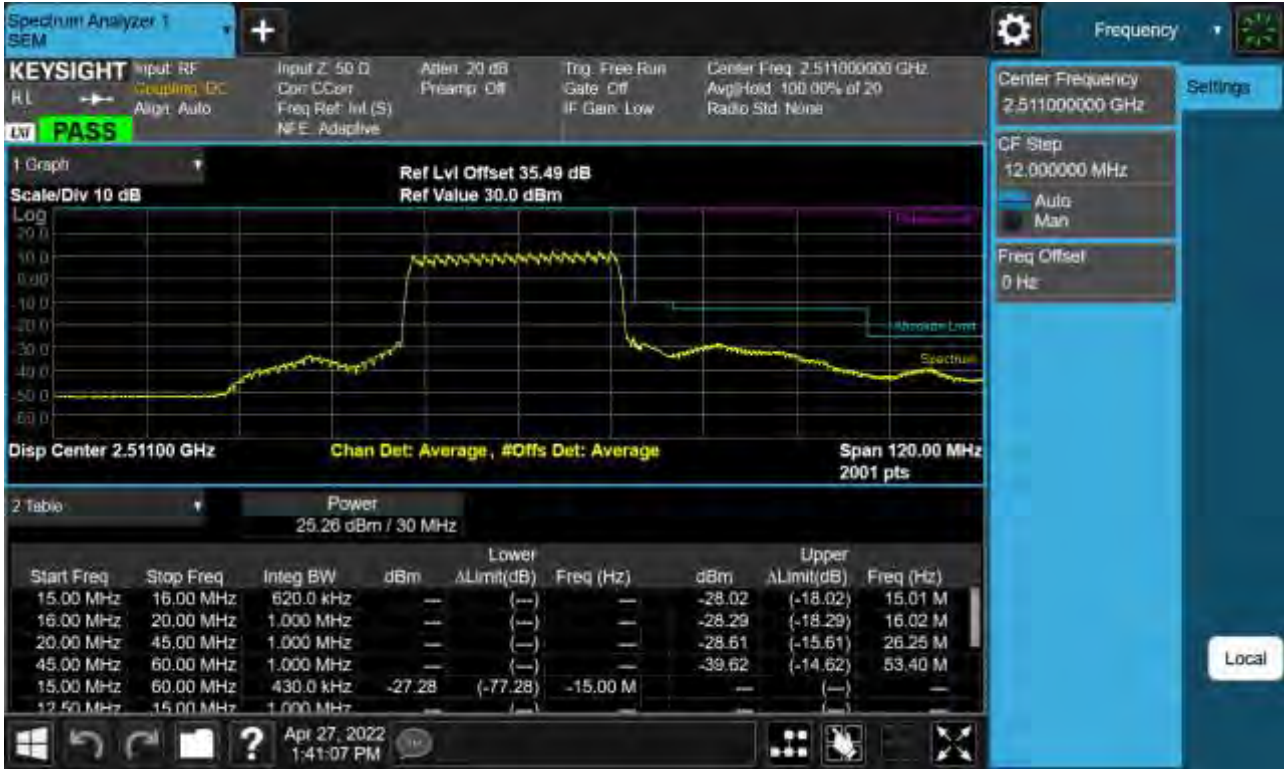
Sub6 n41. Low Channel Edge Plot (30 MHz Ch.502200 BPSK)-2
