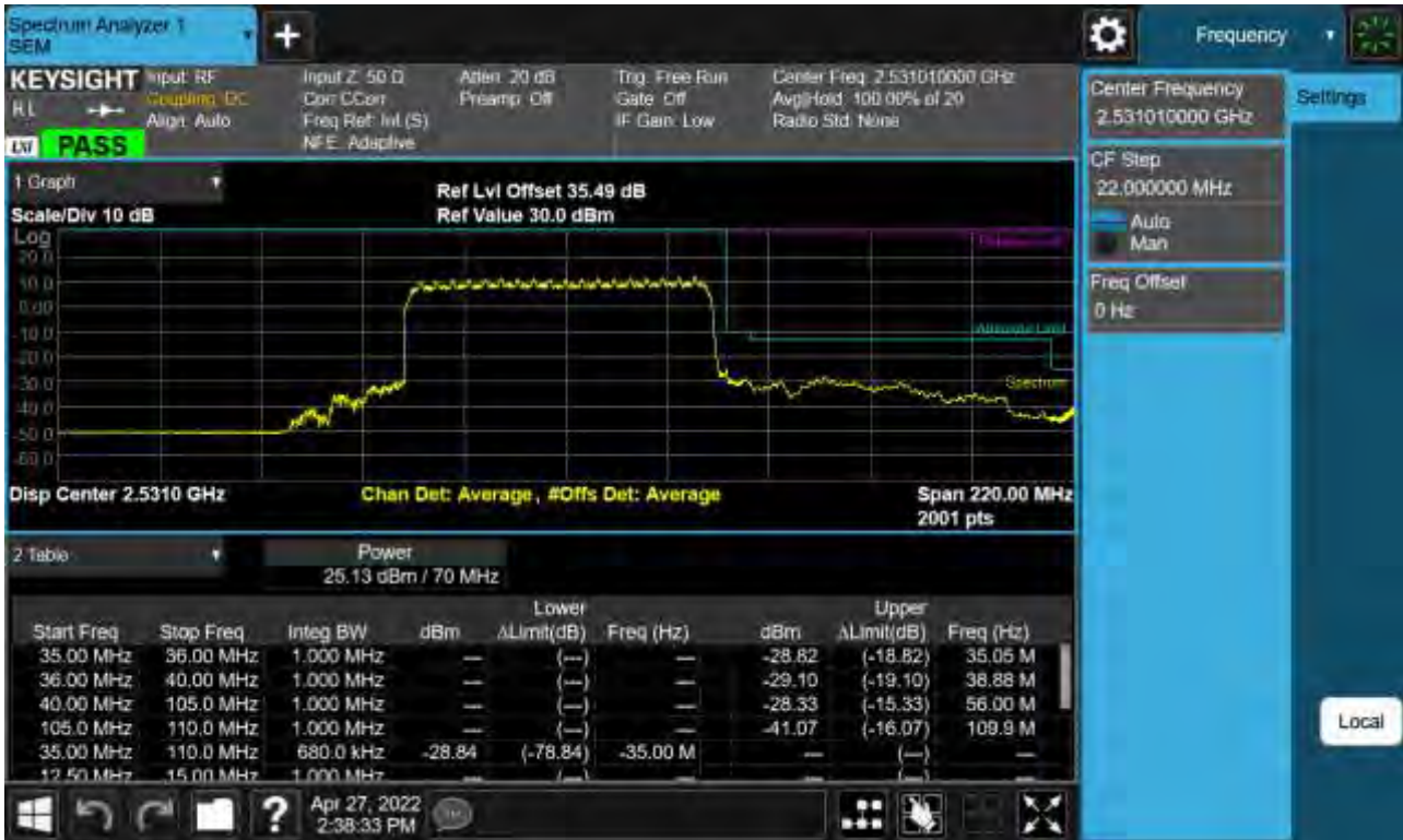
Sub6 n41. Low Channel Edge Plot (70 MHz Ch.506202 BPSK)-2
