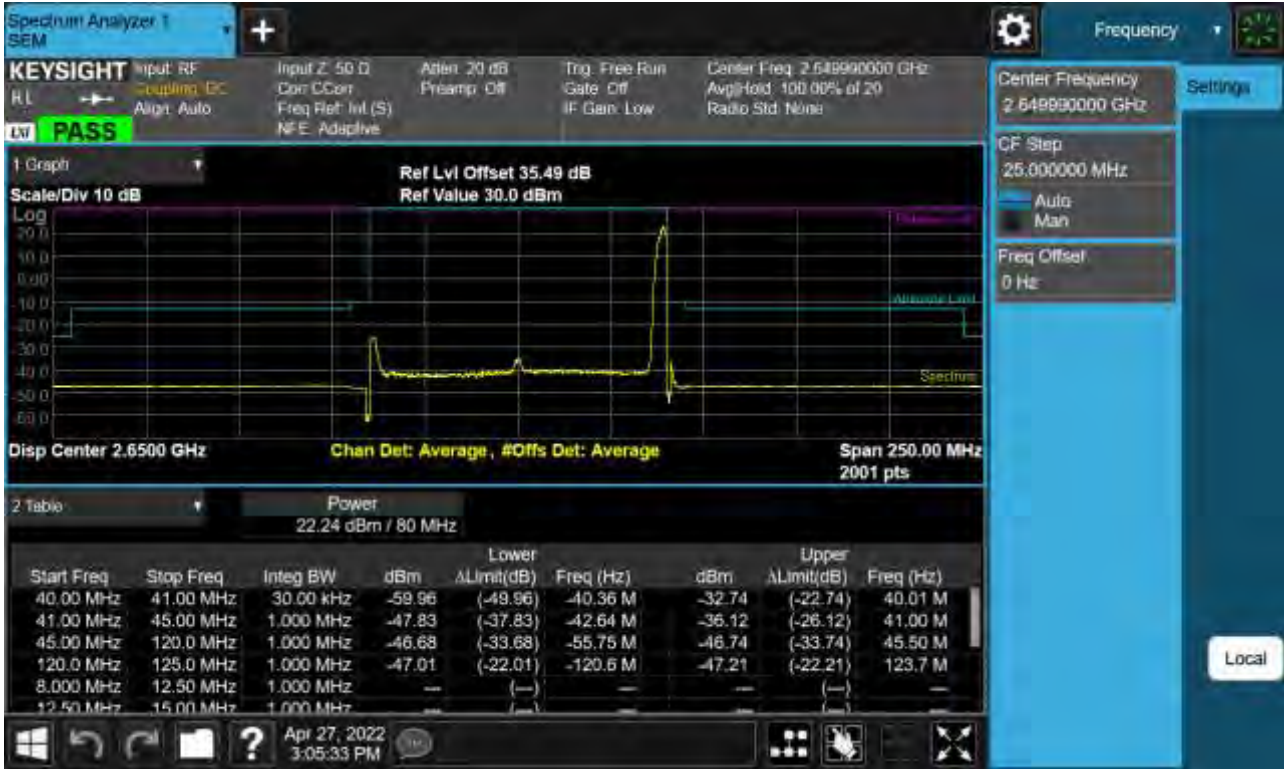
Sub6 n41. High Channel Edge Plot (80 MHz Ch.52998 BPSK RB 1)
