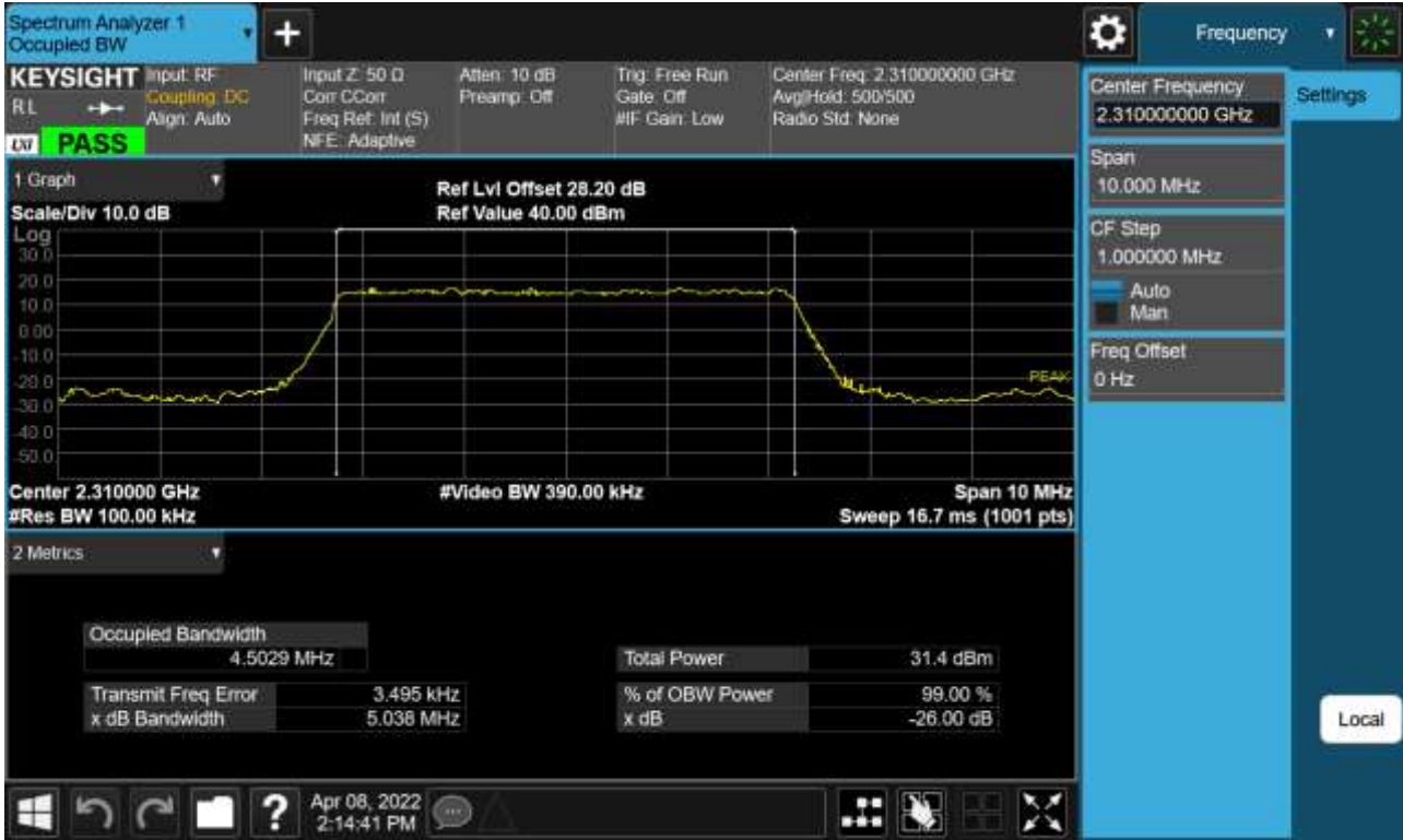
Sub6 n30. Occupied Bandwidth Plot (5 MHz Ch.462000 BPSK RB 25)
