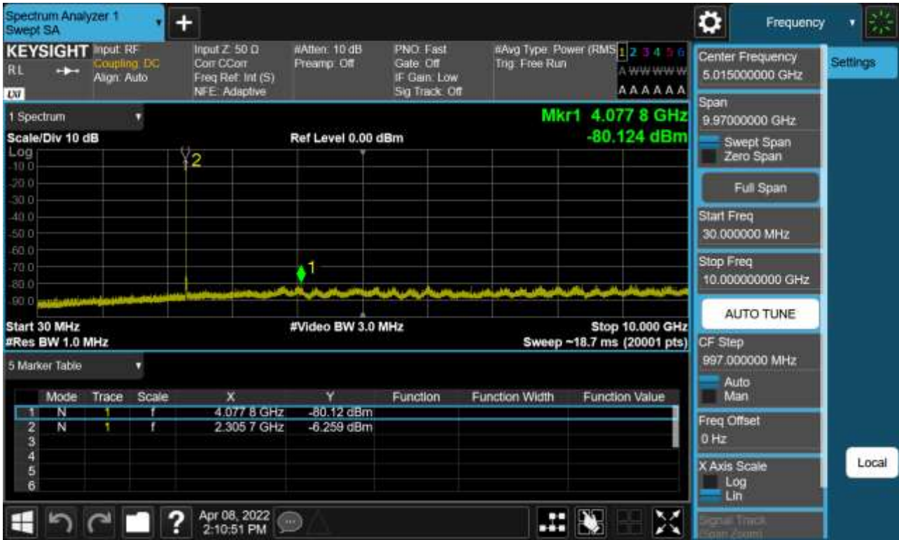
Sub6 n30. Conducted Spurious Plot 1 (5 MHz Ch.461500 BPSK RB 1, Offset 1)
