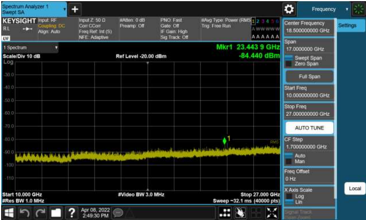
Sub6 n30. Conducted Spurious Plot 2 (10 MHz Ch. 462000 BPSK RB 1, Offset 1)
