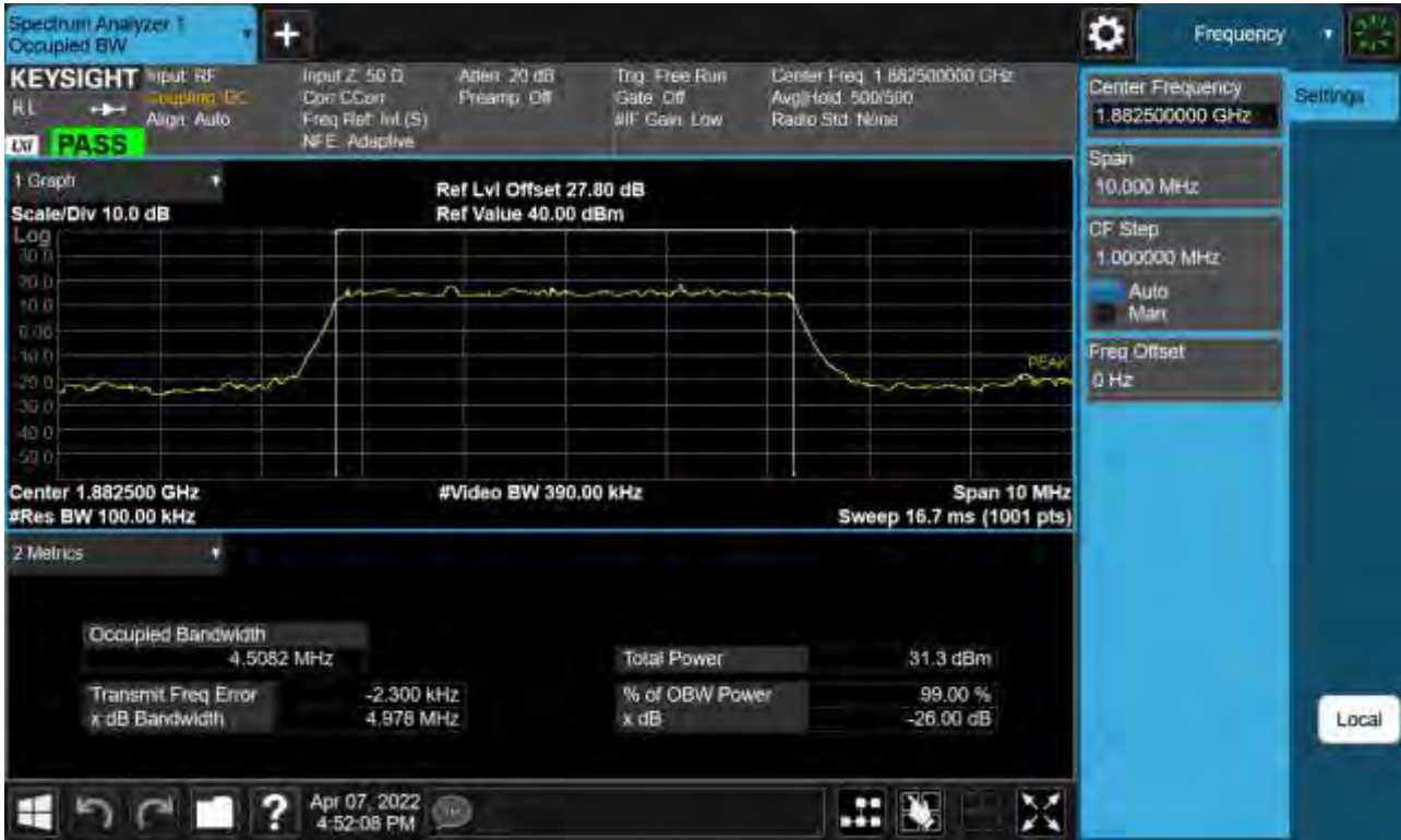
Sub6 n25(2). Occupied Bandwidth Plot (5 M BW Ch.376500 BPSK_ Full RB_0 )
