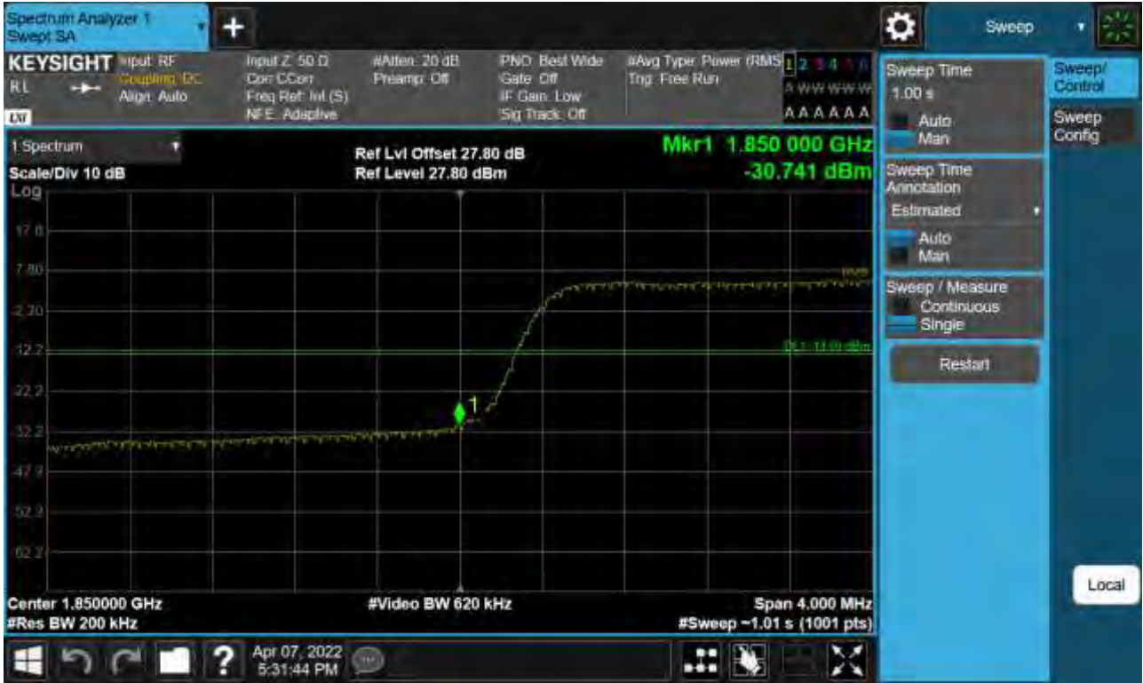
Sub6 n25(2). Lower Band Edge Plot (20 M BW Ch.372000 BPSK_RB100_Offset 0) -1
