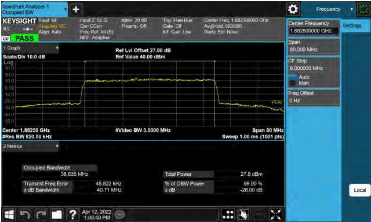
Sub6 n25. Occupied Bandwidth Plot (40 M BW Ch.376500 256QAM_ Full RB _0)
