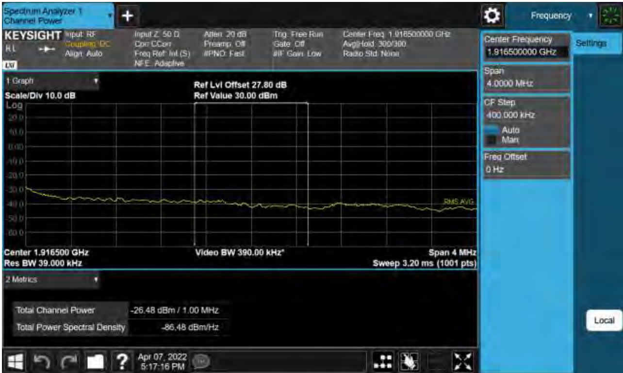
Sub6 n25(2). Upper Extended Band Edge Plot (10 M BW Ch.382000 BPSK_RB50_0) -2
