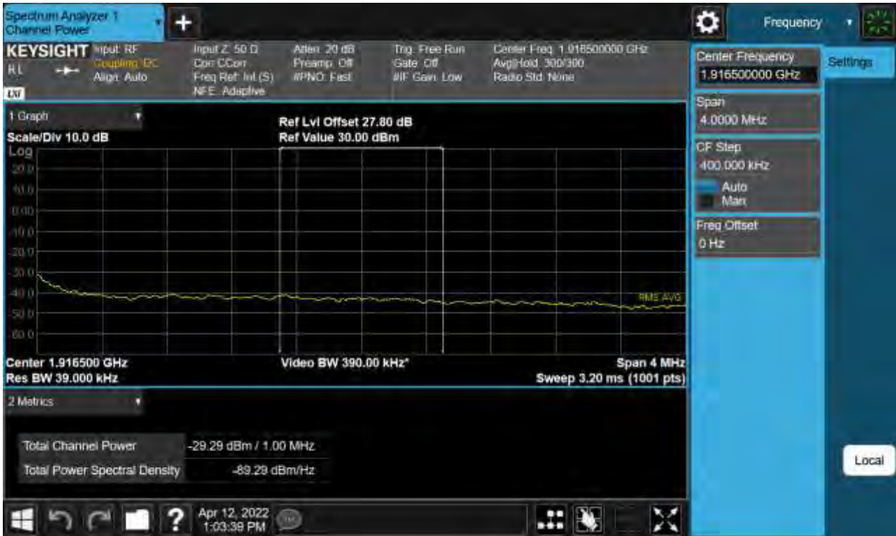
Sub6 n25. Upper Extended Band Edge Plot (40 M BW Ch.379000 BPSK_RB216_0) -2
