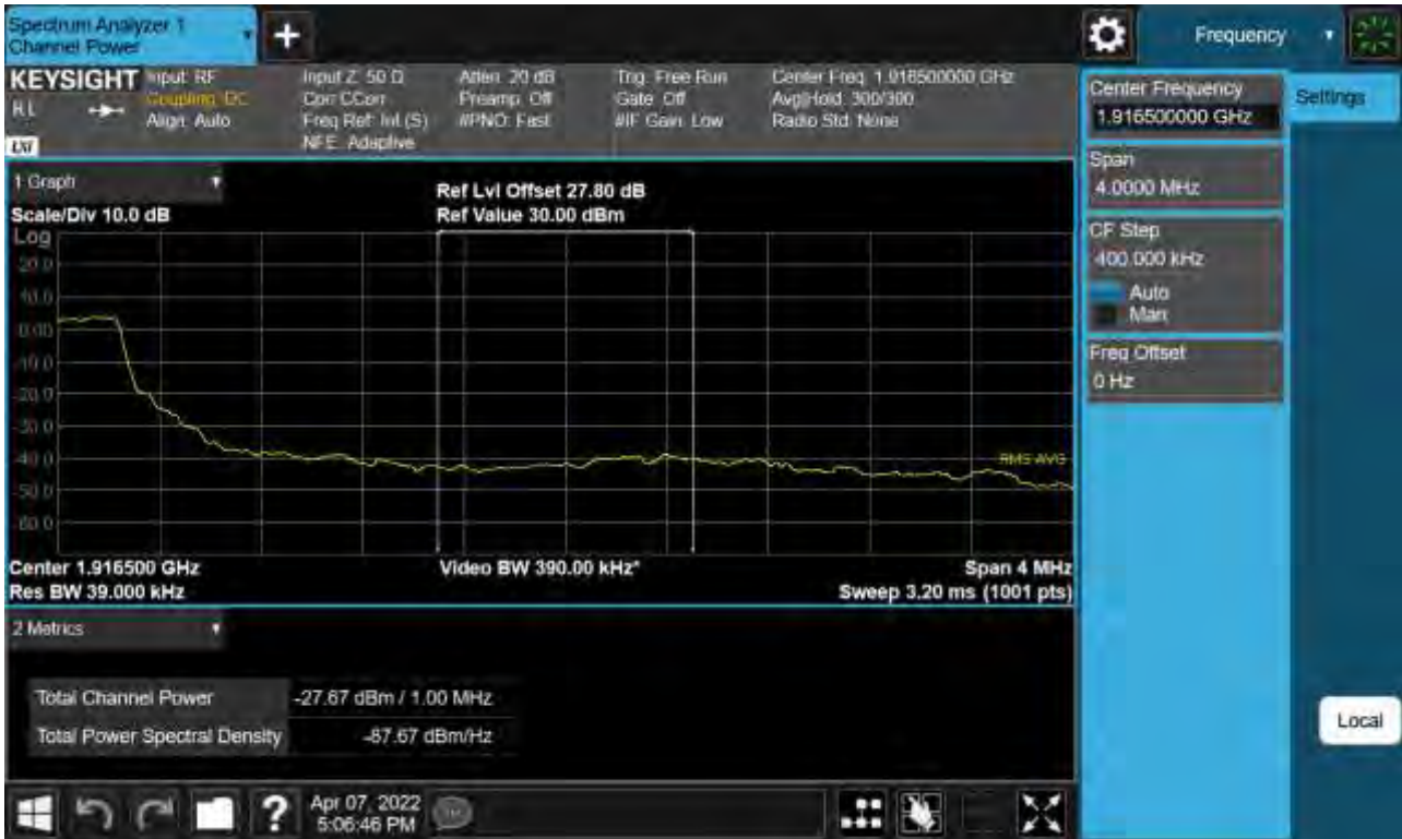
Sub6 n25(2). Upper Extended Band Edge Plot (5 M BW Ch.382500 BPSK_RB25_0) -2
