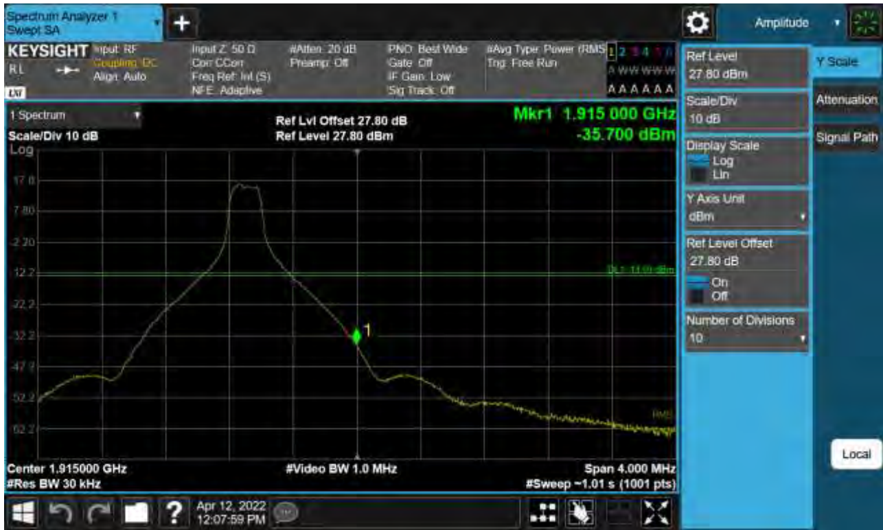
Sub6 n25. Upper Band Edge Plot (30 M BW Ch.380000 BPSK_RB1_Offset 159)
