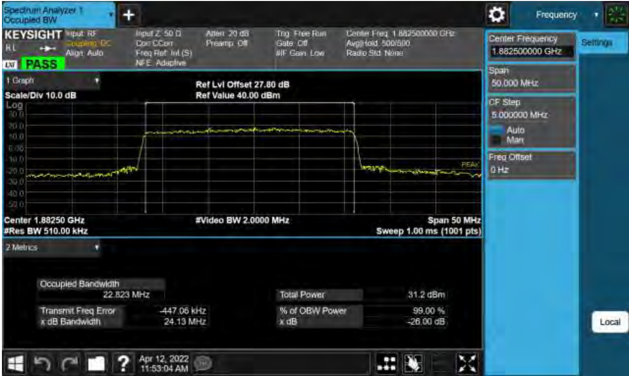
Sub6 n25. Occupied Bandwidth Plot (25 M BW Ch.376500 QPSK _ Full RB _0)
