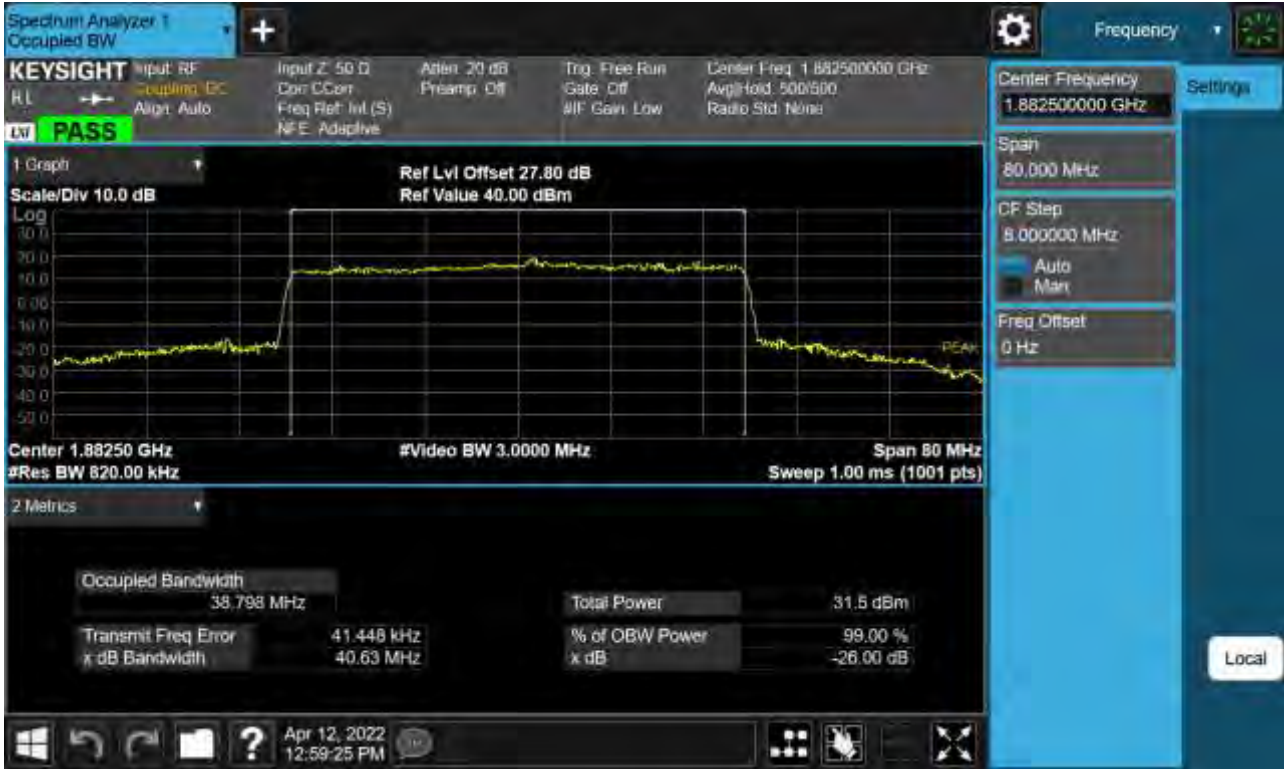
Sub6 n25. Occupied Bandwidth Plot (40 M BW Ch.376500 QPSK_ Full RB_0)
