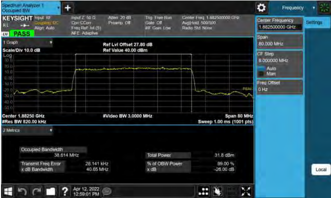
Sub6 n25. Occupied Bandwidth Plot (40 M BW Ch.376500 BPSK_ Full RB_0)
