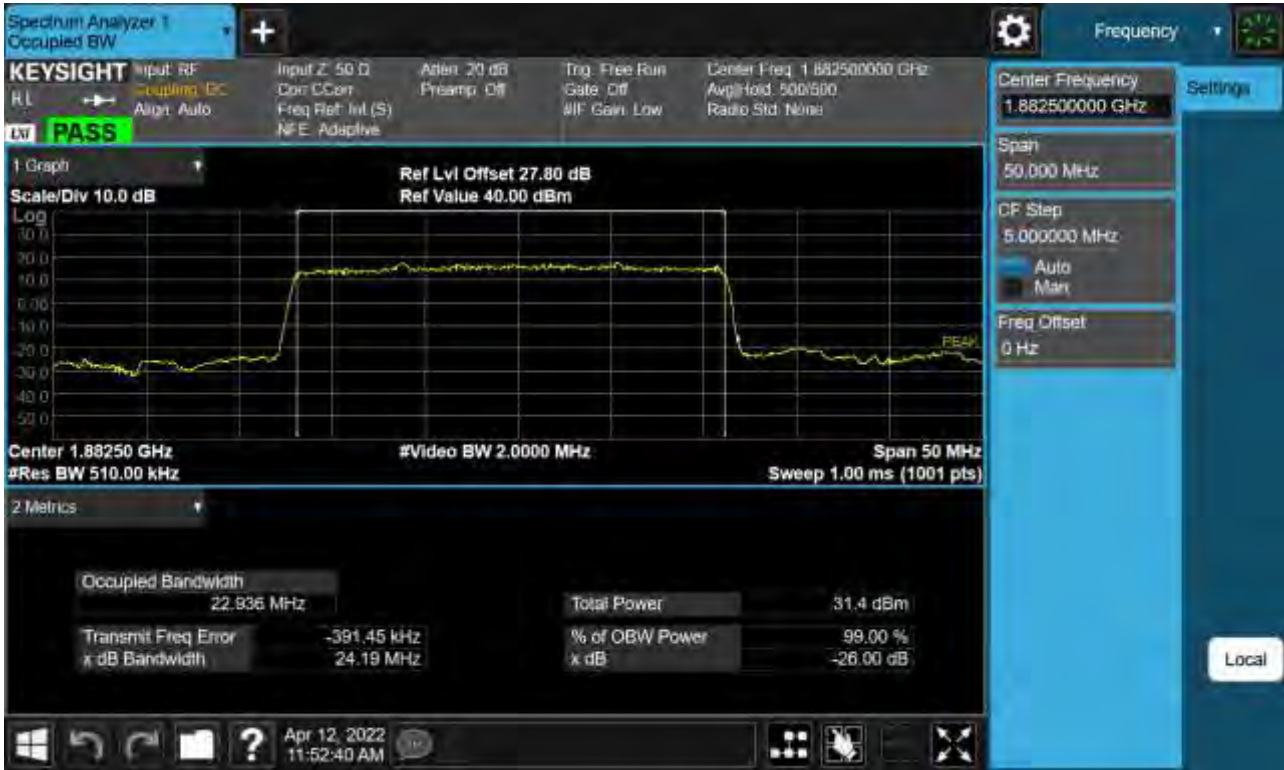
Sub6 n25. Occupied Bandwidth Plot (25 M BW Ch.376500 BPSK _ Full RB _0)
