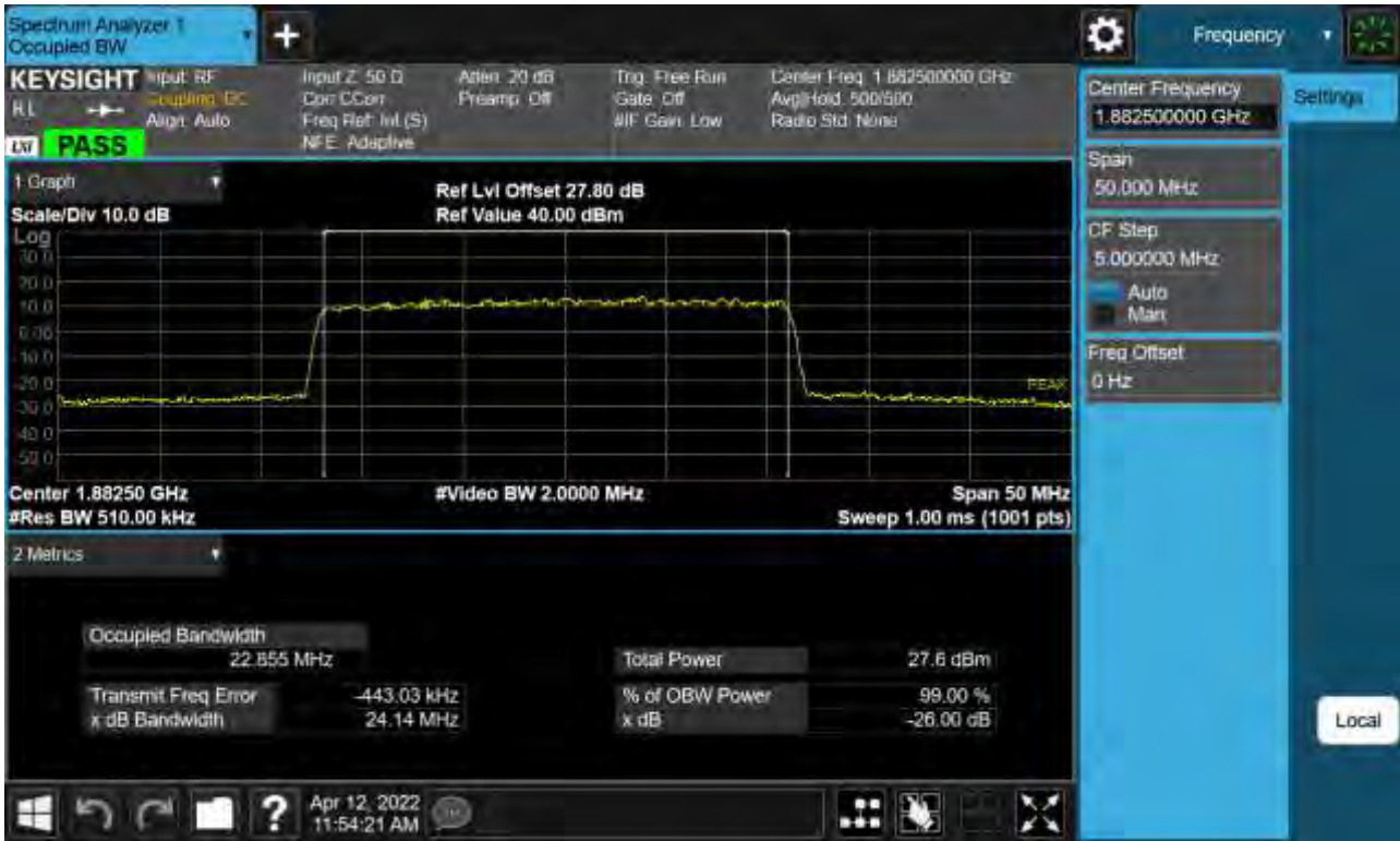
Sub6 n25. Occupied Bandwidth Plot (25 M BW Ch.376500 256QAM _ Full RB _0)
