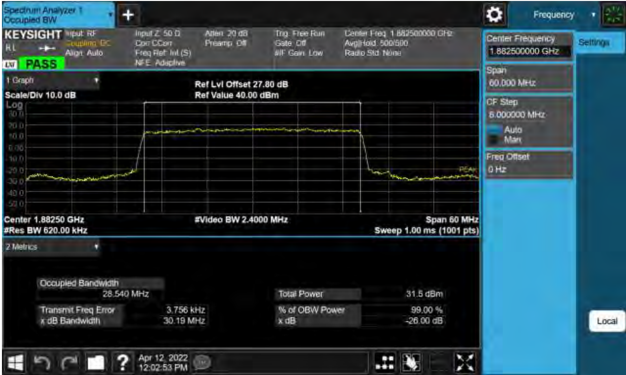
Sub6 n25. Occupied Bandwidth Plot (30 M BW Ch.376500 BPSK_ Full RB_0)
