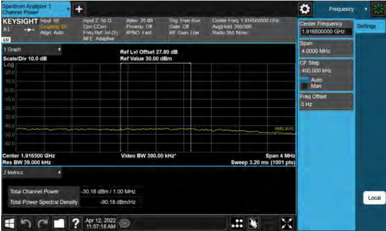
Sub6 n25. Upper Extended Band Edge Plot (25 M BW Ch.380500 BPSK_RB100_0) -2
