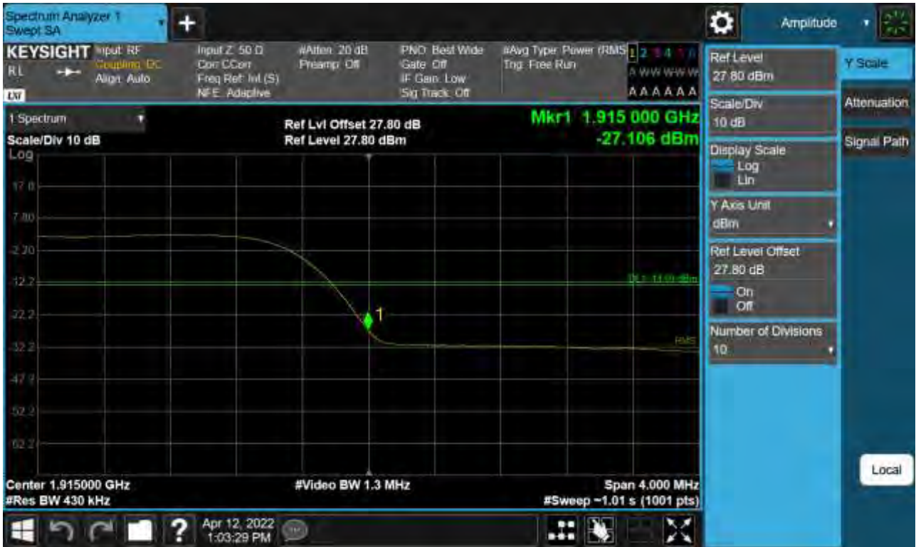
Sub6 n25. Upper Band Edge Plot (40 M BW Ch.379000 BPSK_RB216_Offset 0) -1
