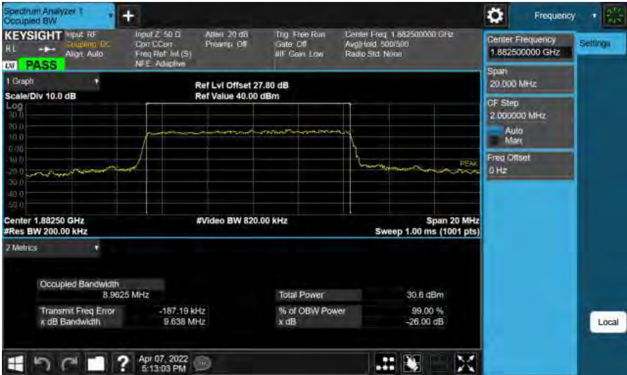
Sub6 n25(2). Occupied Bandwidth Plot (10 M BW Ch.376500 QPSK _ Full RB _0)
