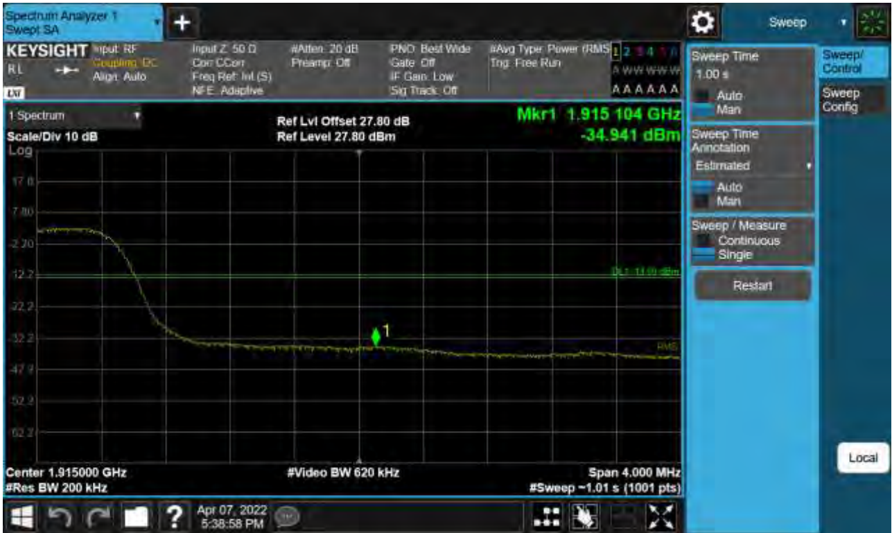
Sub6 n25(2). Upper Band Edge Plot (20 M BW Ch.381000 BPSK_RB100_Offset 0) -1
