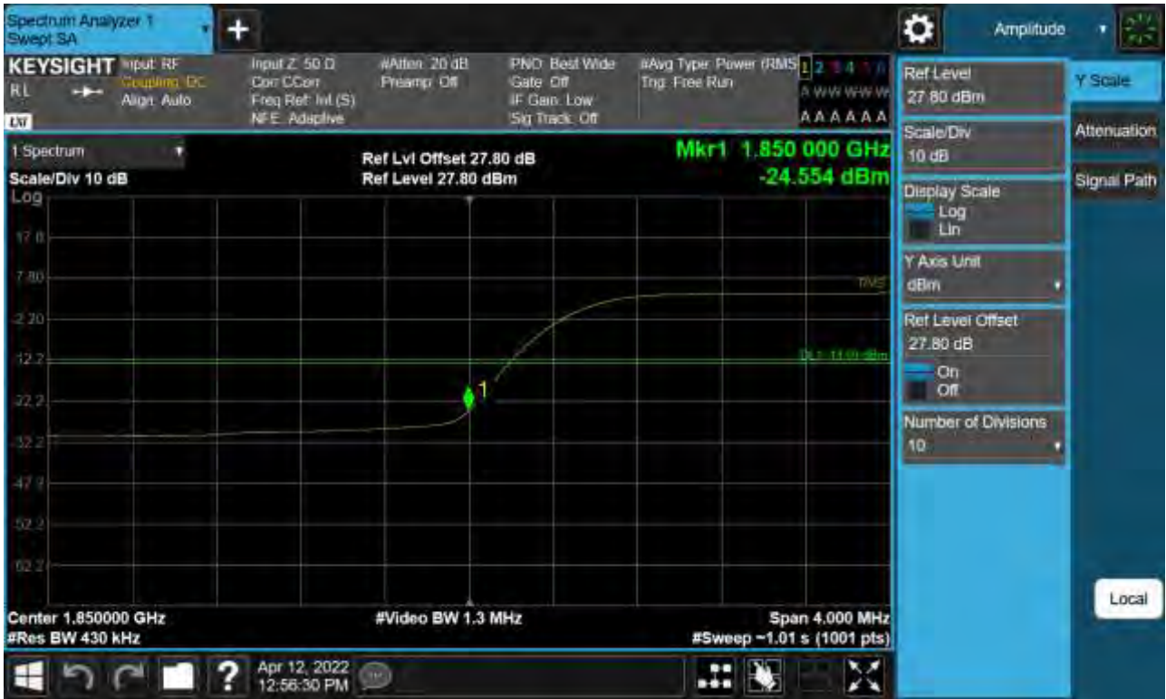
Sub6 n25. Lower Band Edge Plot (40 M BW Ch.374000 BPSK_RB216_Offset 0) -1
