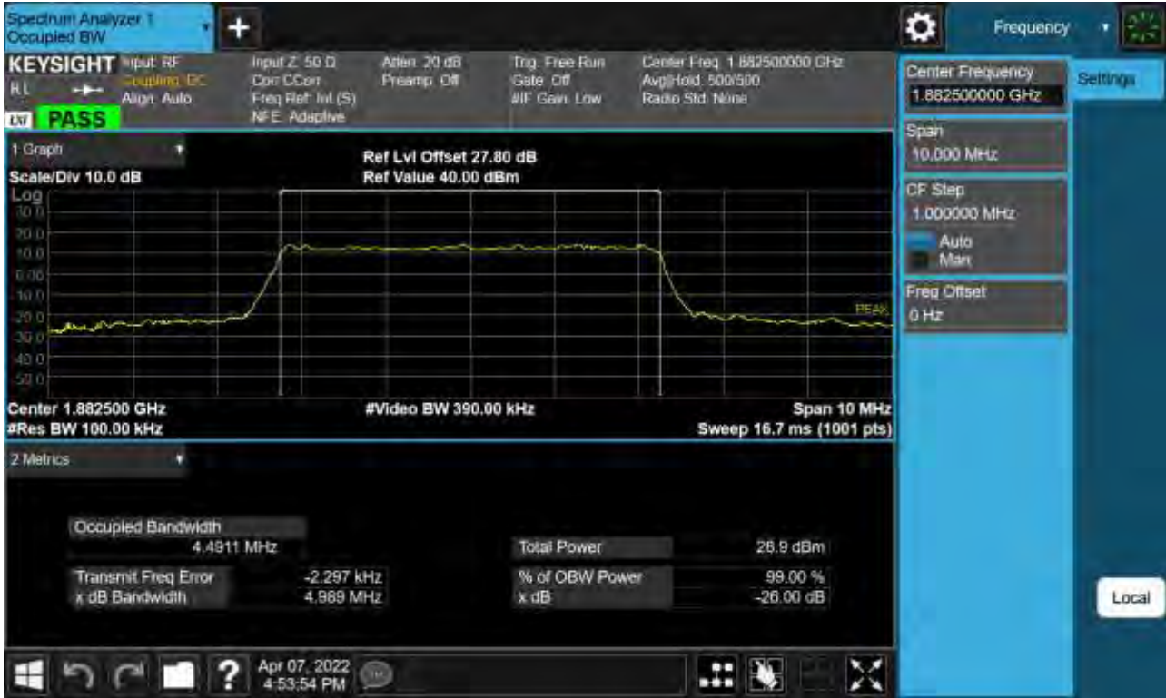
Sub6 n25(2). Occupied Bandwidth Plot (5 M BW Ch.376500 64QAM_ Full RB_0)
