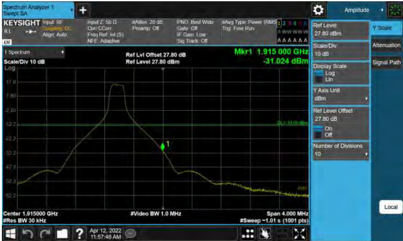
Sub6 n25. Upper Band Edge Plot (25 M BW Ch.380500 BPSK_RB1_Offset 99)
