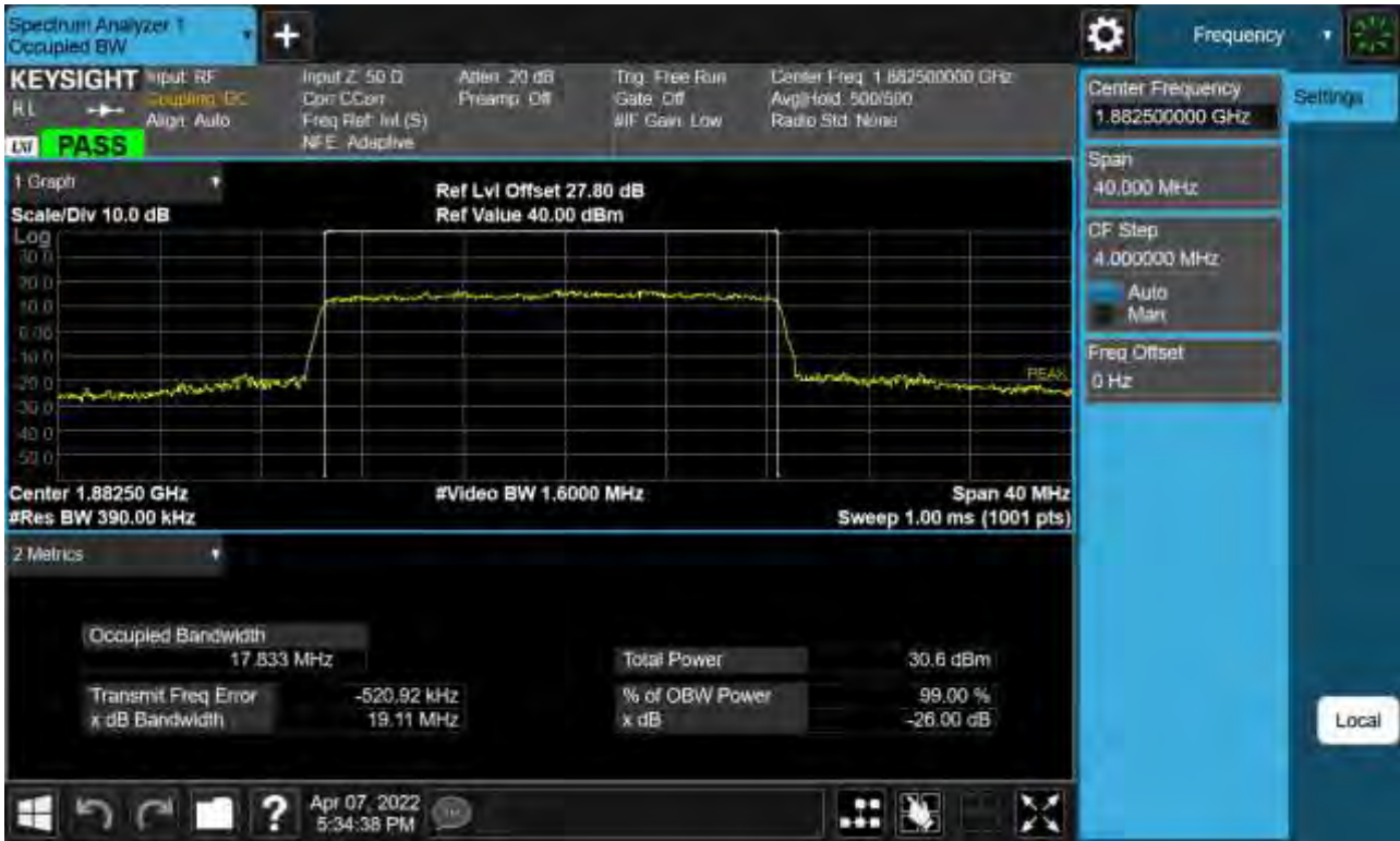
Sub6 n25(2). Occupied Bandwidth Plot (20 M BW Ch.376500 QPSK _ Full RB _0)
