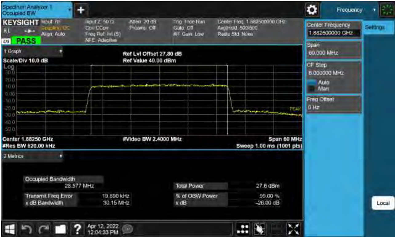
Sub6 n25. Occupied Bandwidth Plot (30 M BW Ch.376500 256QAM_ Full RB _0)
