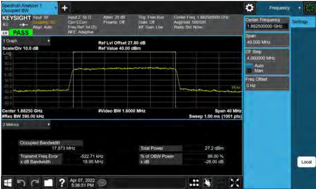
Sub6 n25(2). Occupied Bandwidth Plot (20 M BW Ch.376500 256QAM _ Full RB _0)
