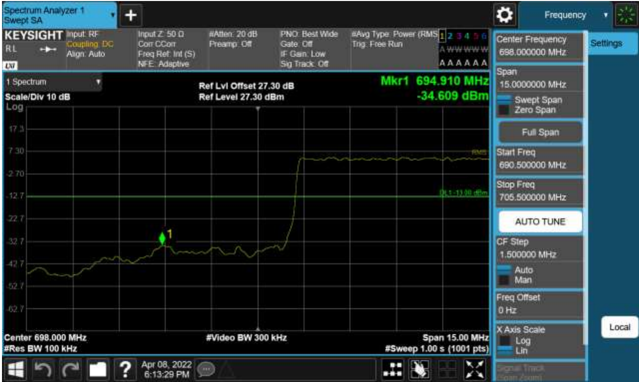
Sub6 n12. Lower Band Edge Plot (10M BW Ch.140800 BPSK_RB50_Offset 0)
