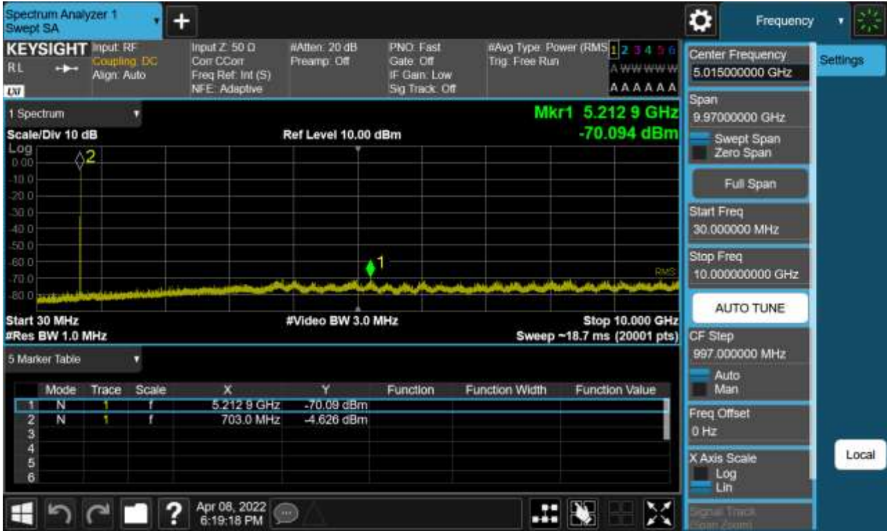
Sub6 n12. Conducted Spurious Plot _ (141500ch_10MHz_BPSK_RB 1_1)
