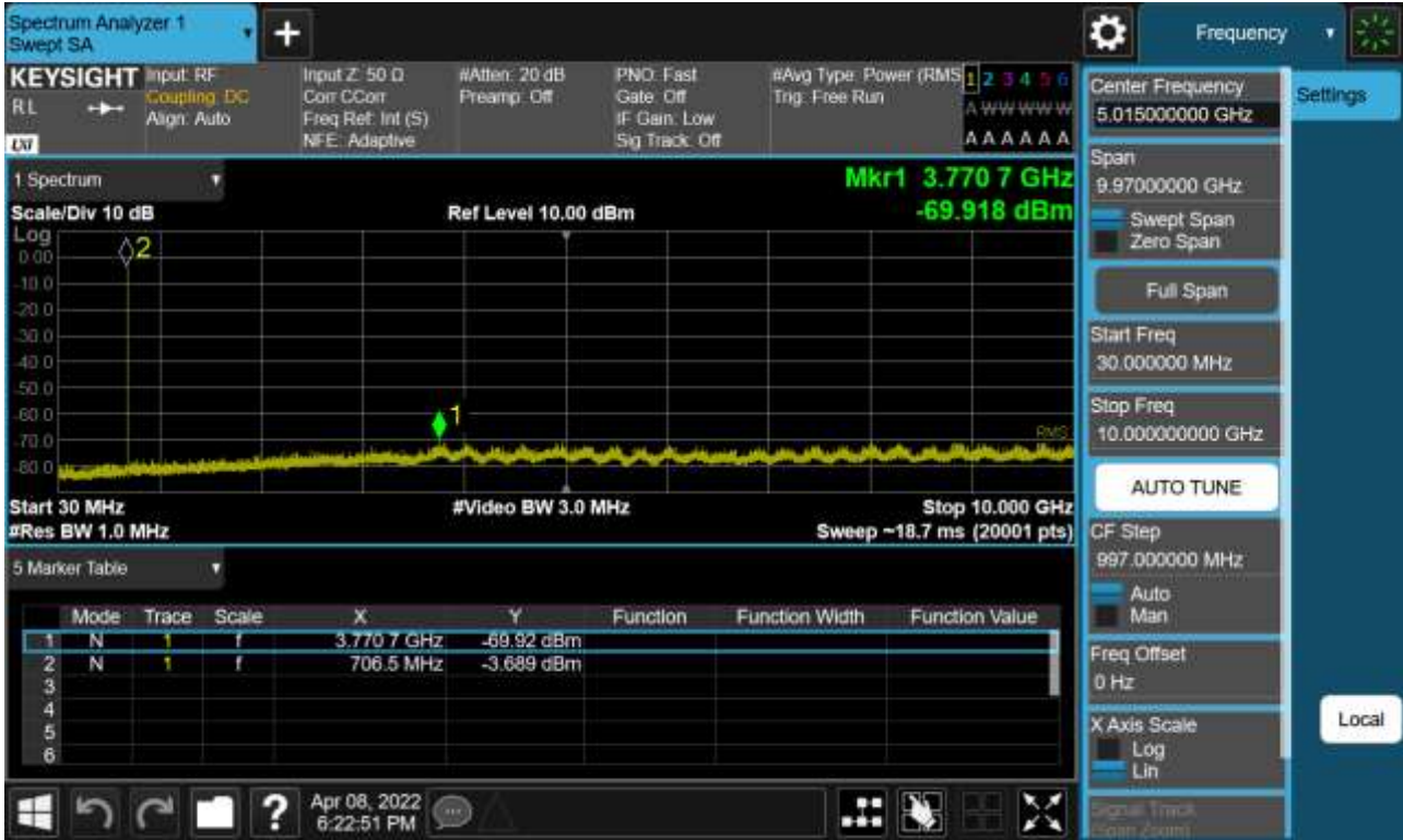
Sub6 n12. Conducted Spurious Plot _ (142200ch_10MHz_BPSK_RB 1_1)
