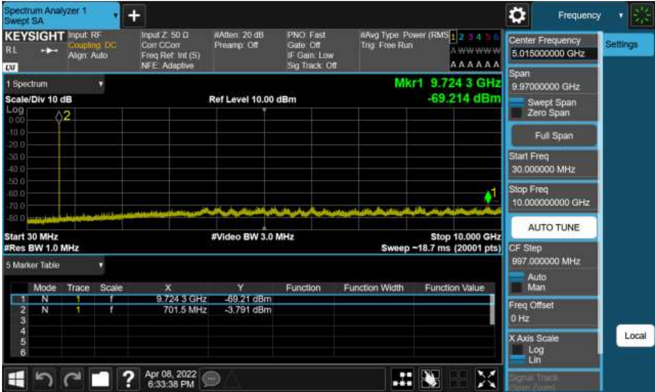
Sub6 n12. Conducted Spurious Plot _ (141700ch_15MHz_BPSK_RB 1_1)
