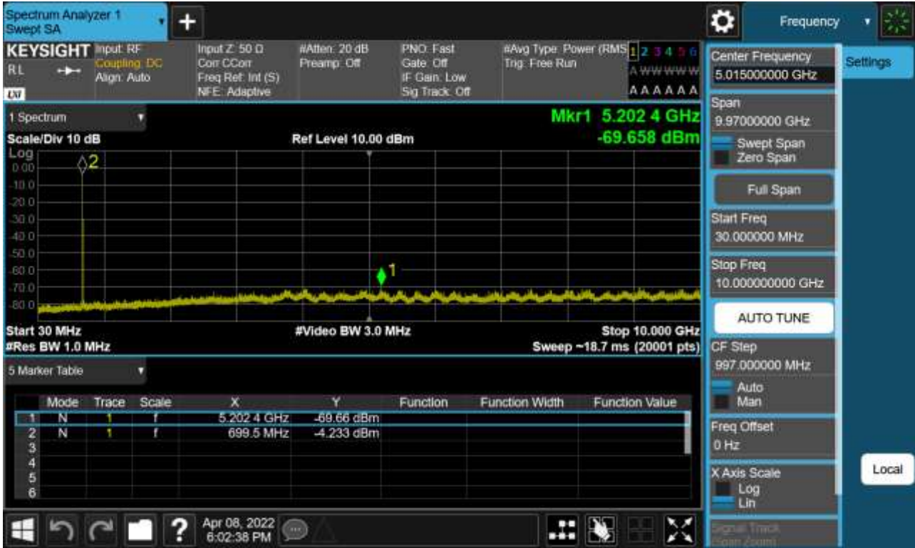
Sub6 n12. Conducted Spurious Plot _ (140300ch_5MHz_BPSK_RB 1_1)
