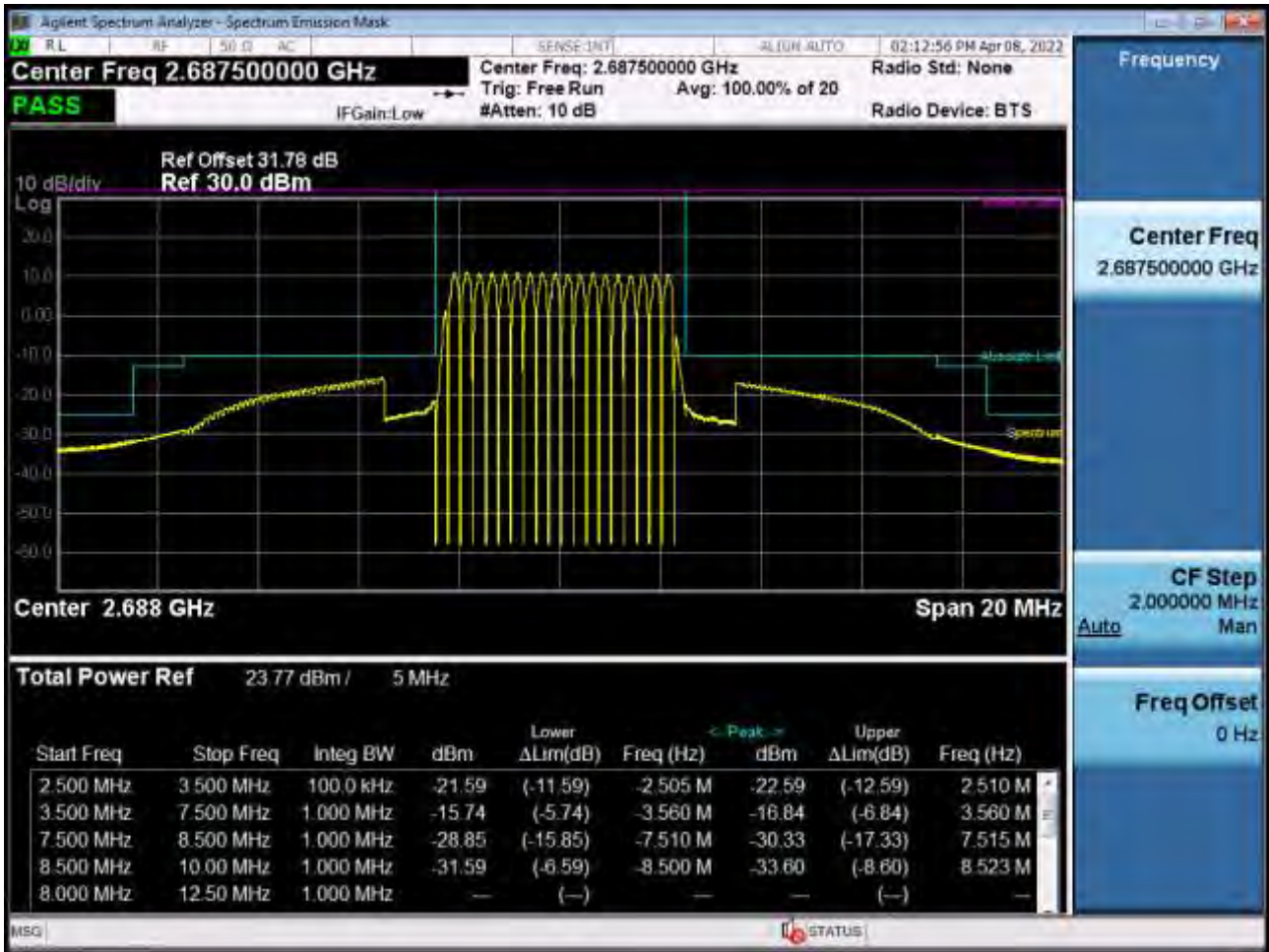
High Channel Edge Plot (5 MHz Ch.41565 QPSK_RB25_Offset 0) (POWER CLASS 3)
