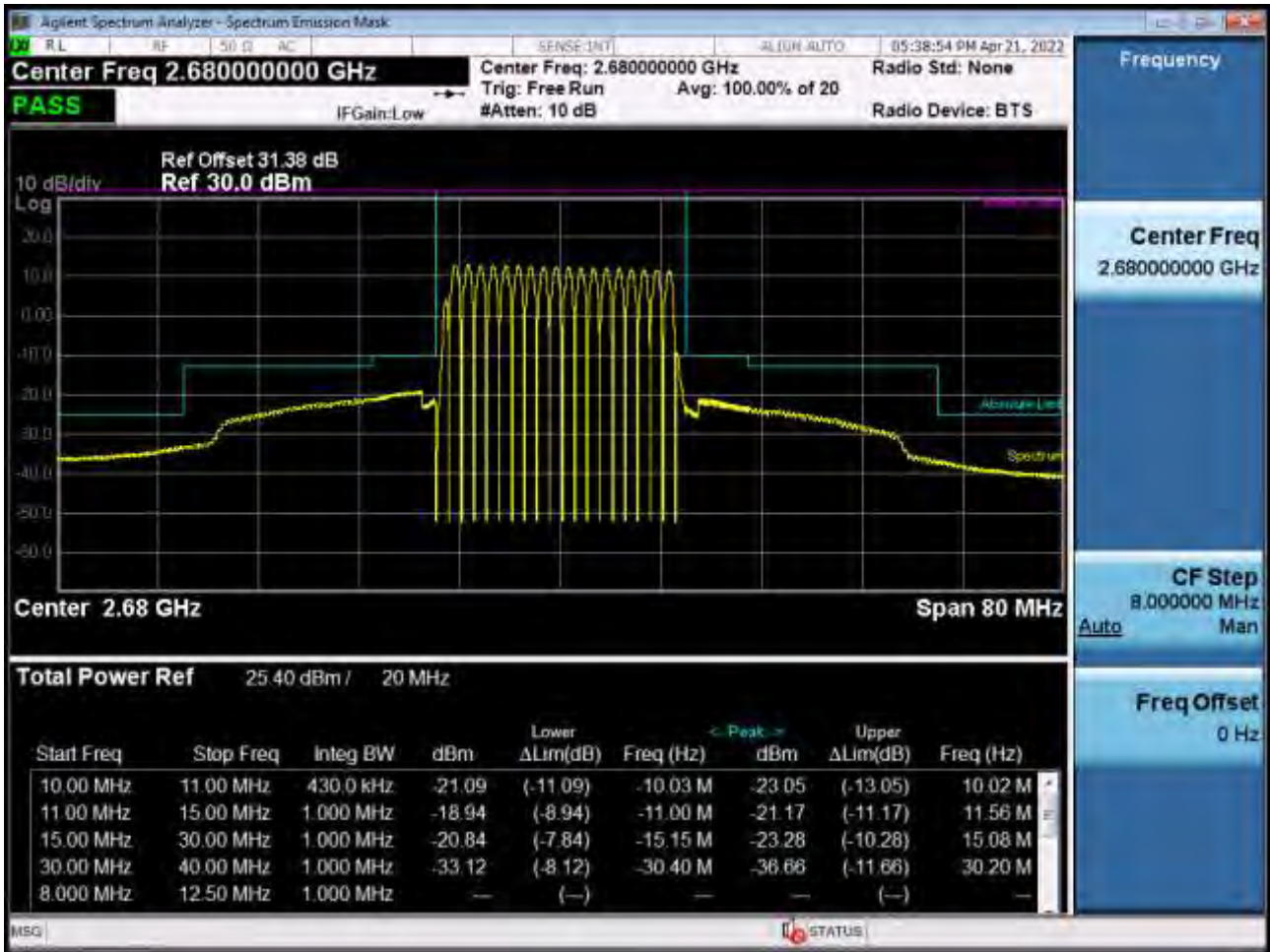
High Channel Edge Plot (20 MHz Ch.41490 QPSK_RB100_Offset 0) (POWER CLASS 2)
