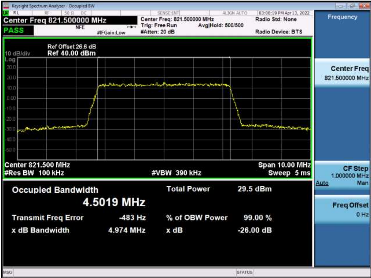
BAND 26. Occupied Bandwidth Plot (5 M BW Ch.26765 64QAM RB 25_0)
