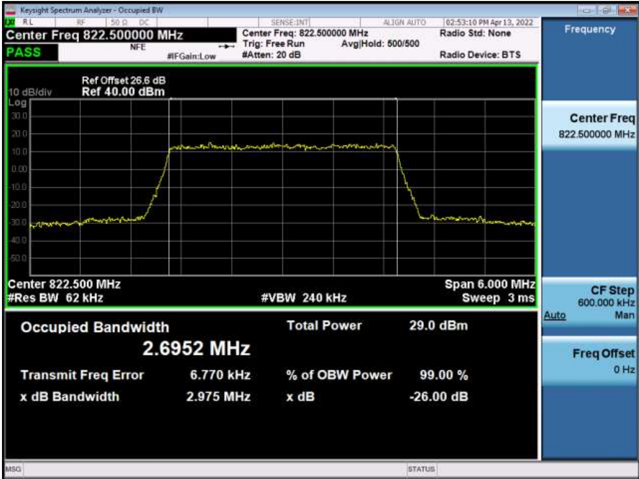
BAND 26. Occupied Bandwidth Plot (3 M BW Ch.26775 64QAM RB 15_0)
