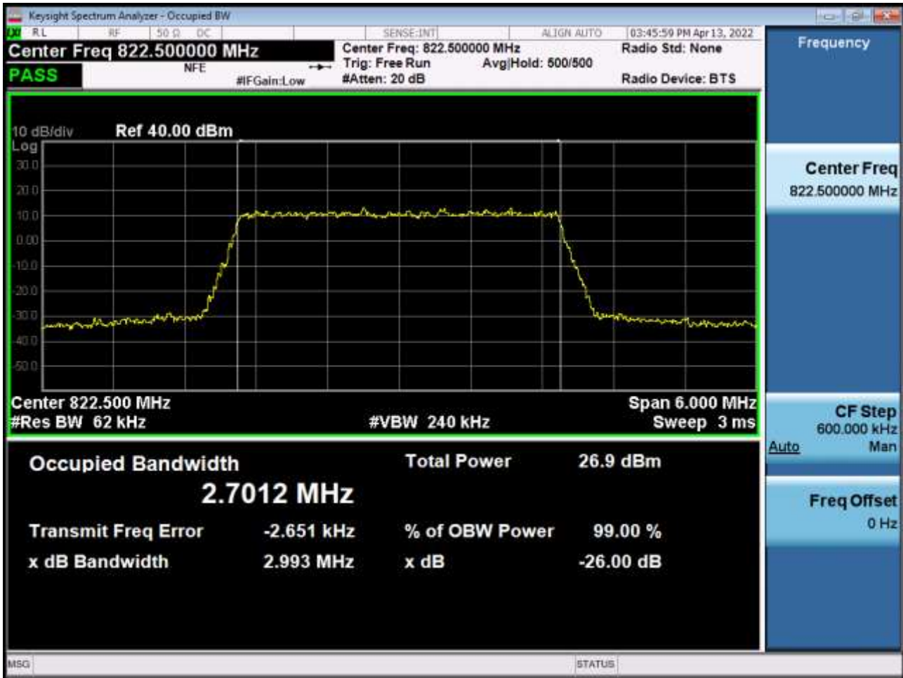
BAND 26. Occupied Bandwidth Plot (3 M BW Ch.26775 256QAM RB 15_0)
