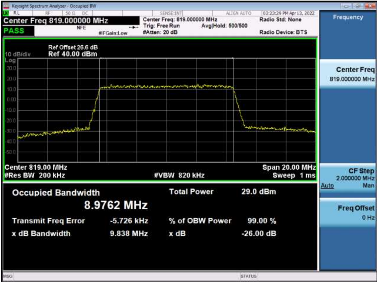
BAND 26. Occupied Bandwidth Plot (10 M BW Ch.26740 64QAM RB 50_0)
