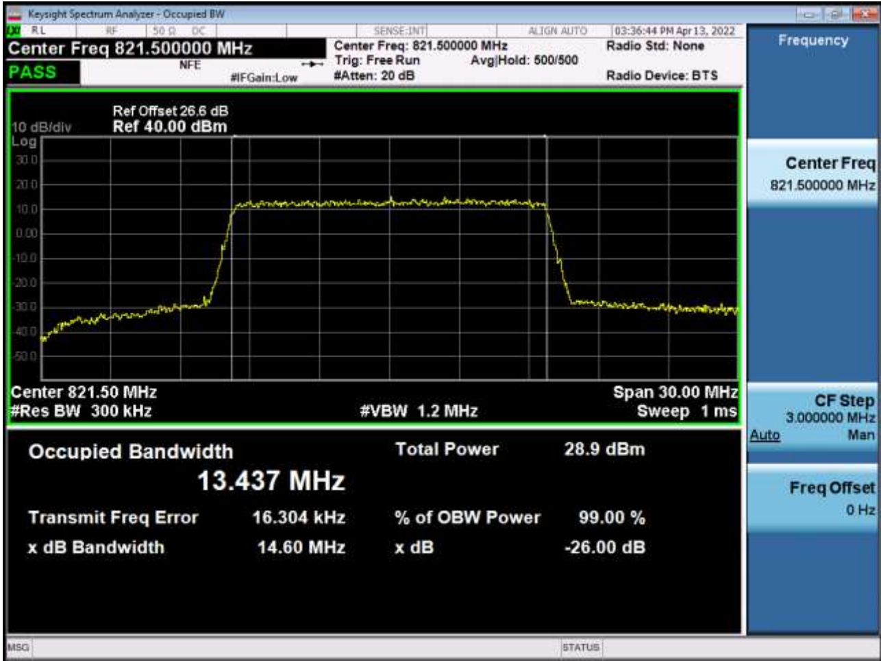
BAND 26. Occupied Bandwidth Plot (15 M BW Ch.26765 64QAM RB 75_0)
