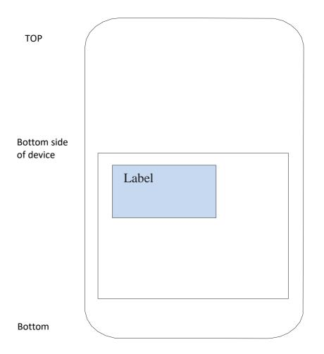
Phone: Label is placed inside of the battery compartment.
