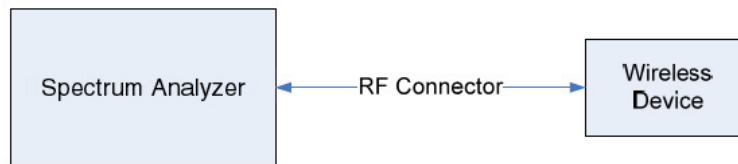
Figure 6-1. Test Instrument & Measurement Setup
