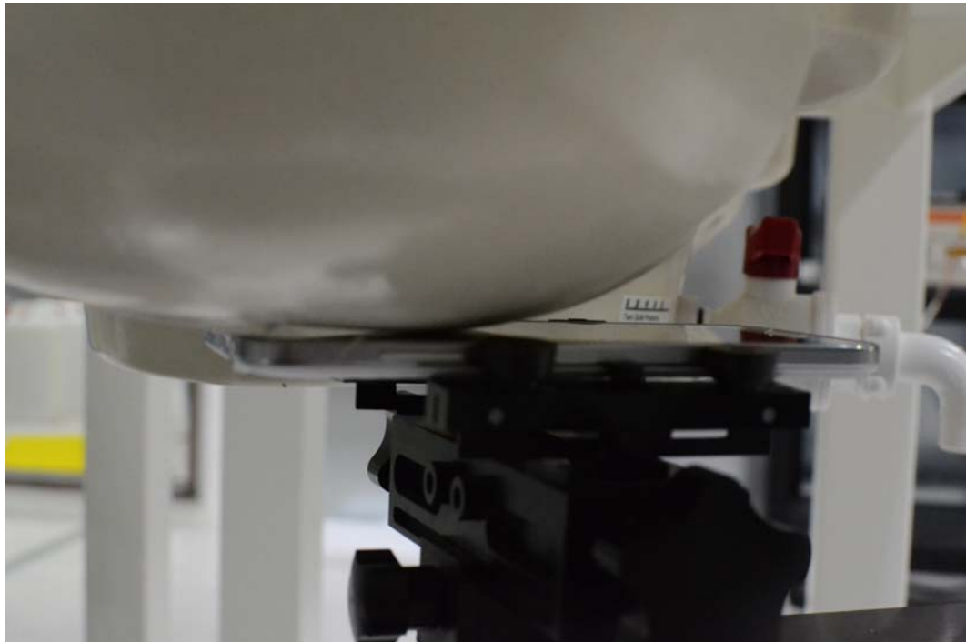
SAR Test Setup Photo 1: Right Cheek
