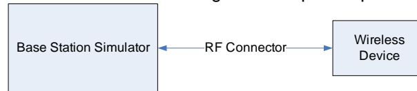
Figure 9-2 Power Measurement Setup
