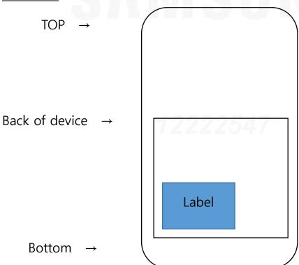
Phone: Label is placed inside of the battery compartment.
