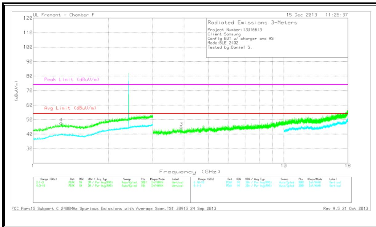
Note: Emission was scanned up to 26GHz; No emissions were detected above the noise floor which was at least 20dB below the specification limit.
