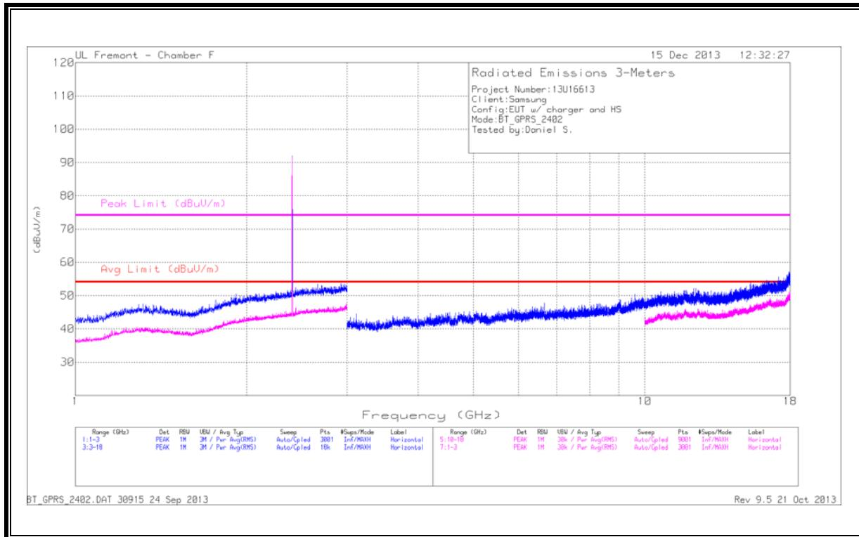
Note: Emission was scanned up to 26GHz; No emissions were detected above the noise floor which was at least 20dB below the specification limit.
