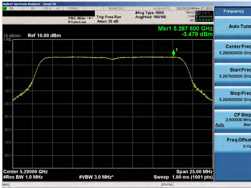
Plot 6-43. Peak Power Spectral Density Plot (20MHz BW 802.11n (UNII Band 2A) – Ch. 56)
