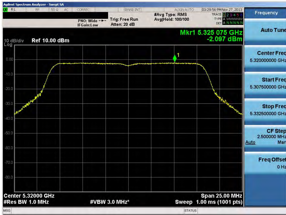
Plot 6-41. Peak Power Spectral Density Plot (802.11a (UNII Band 2A) – Ch. 64)
