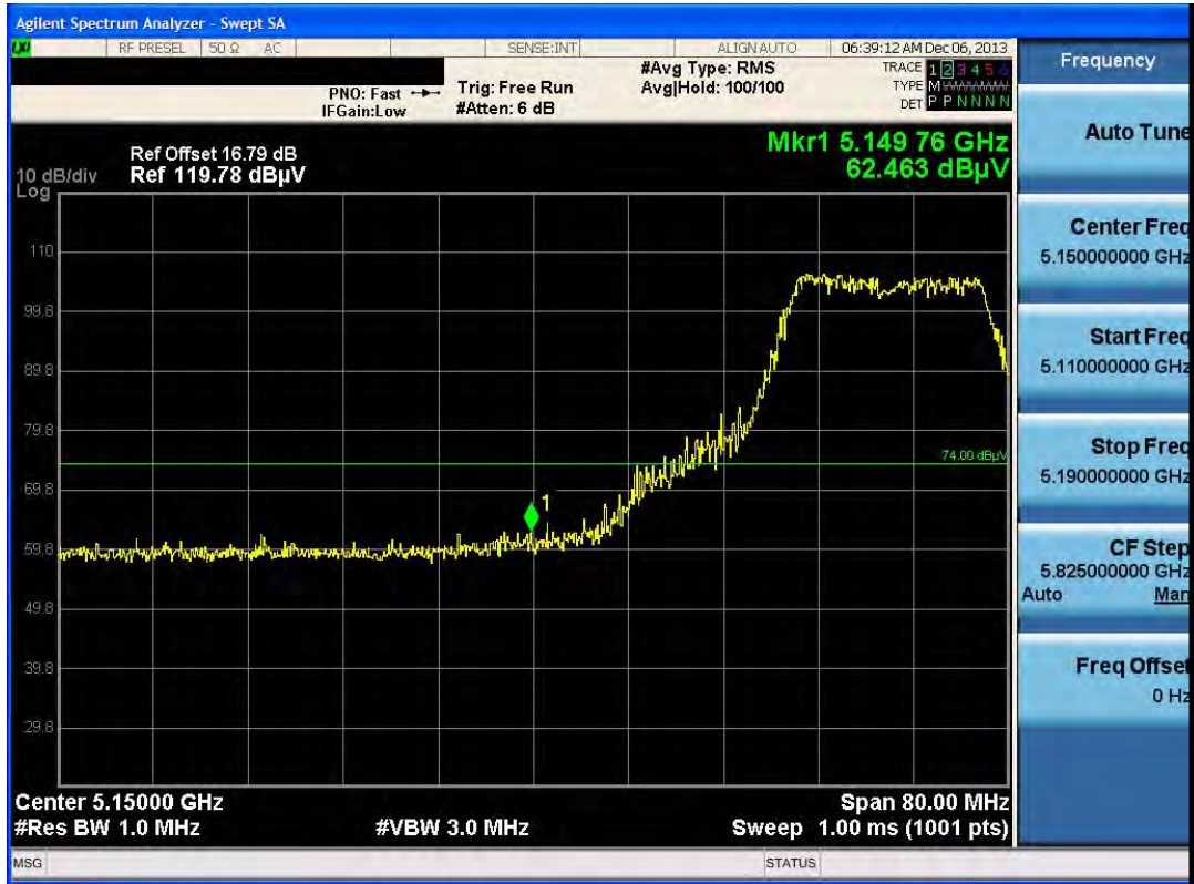
Plot 6-60. Radiated Restricted Lower Band Edge Plot (Peak – UNII Band 1)
