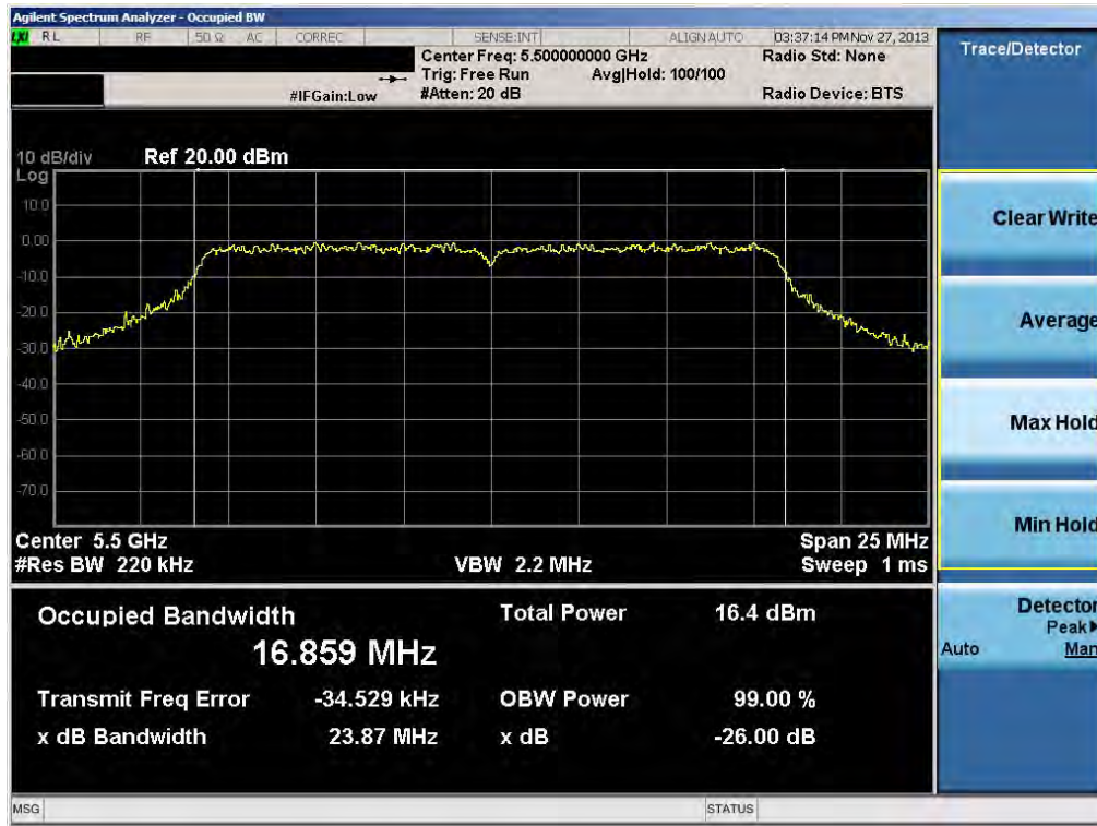
Plot 6-17. 26dB Bandwidth Plot (802.11a (UNII Band 2C) – Ch. 100)
