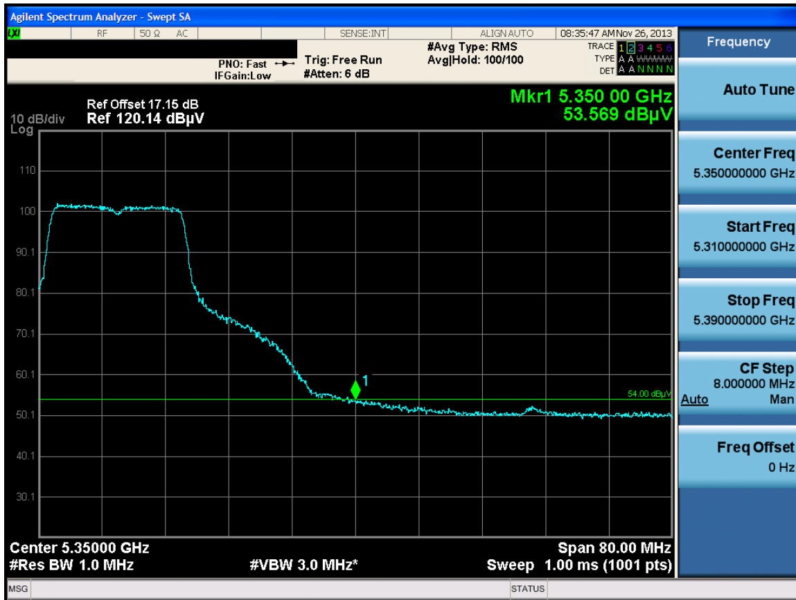
Plot 6-61. Radiated Restricted Upper Band Edge Plot (Average – UNII Band 2A)
