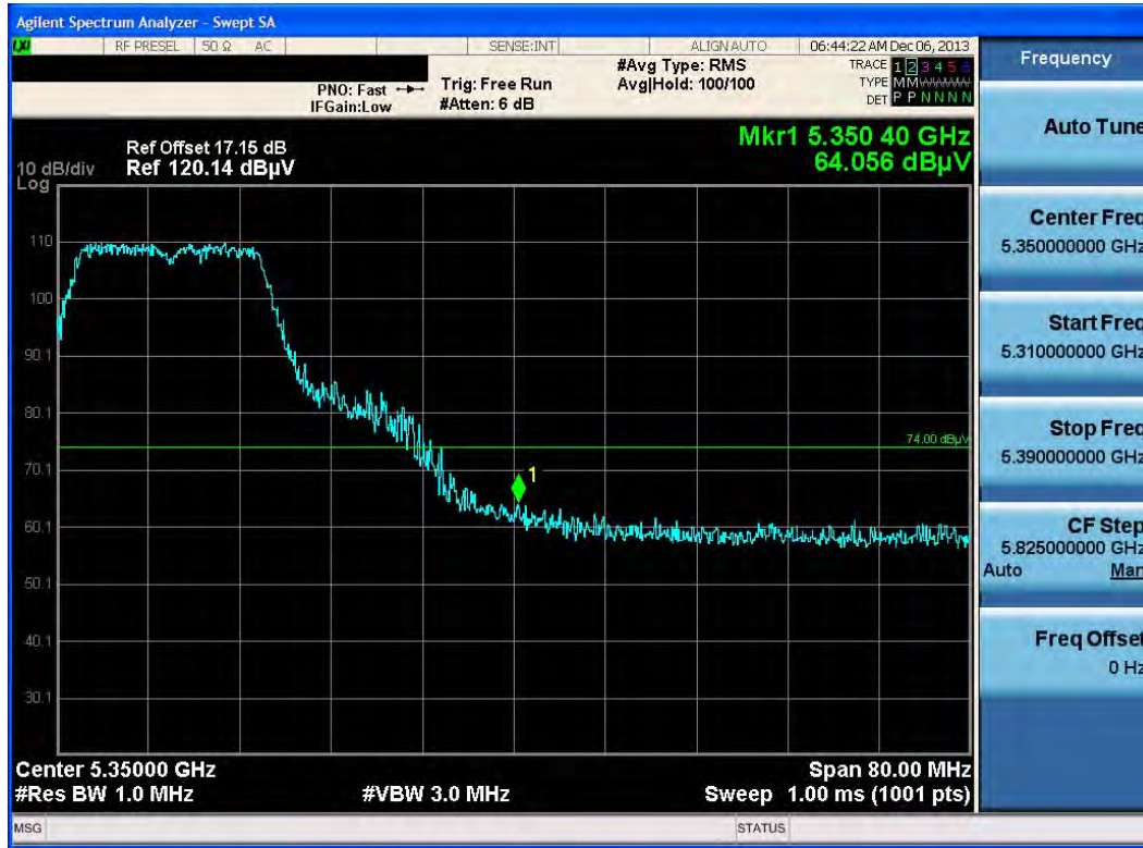
Plot 6-62. Radiated Restricted Upper Band Edge Plot (Peak – UNII Band 2A)
