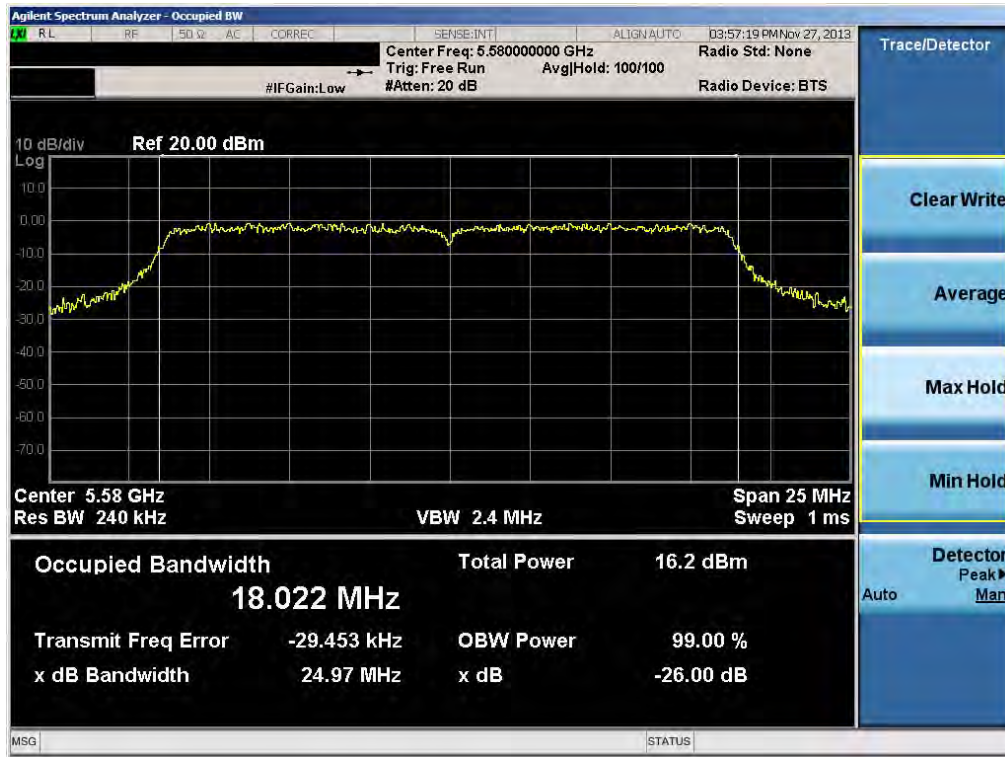
Plot 6-21. 26dB Bandwidth Plot (20MHz BW 802.11n (UNII Band 2C) – Ch. 116)
