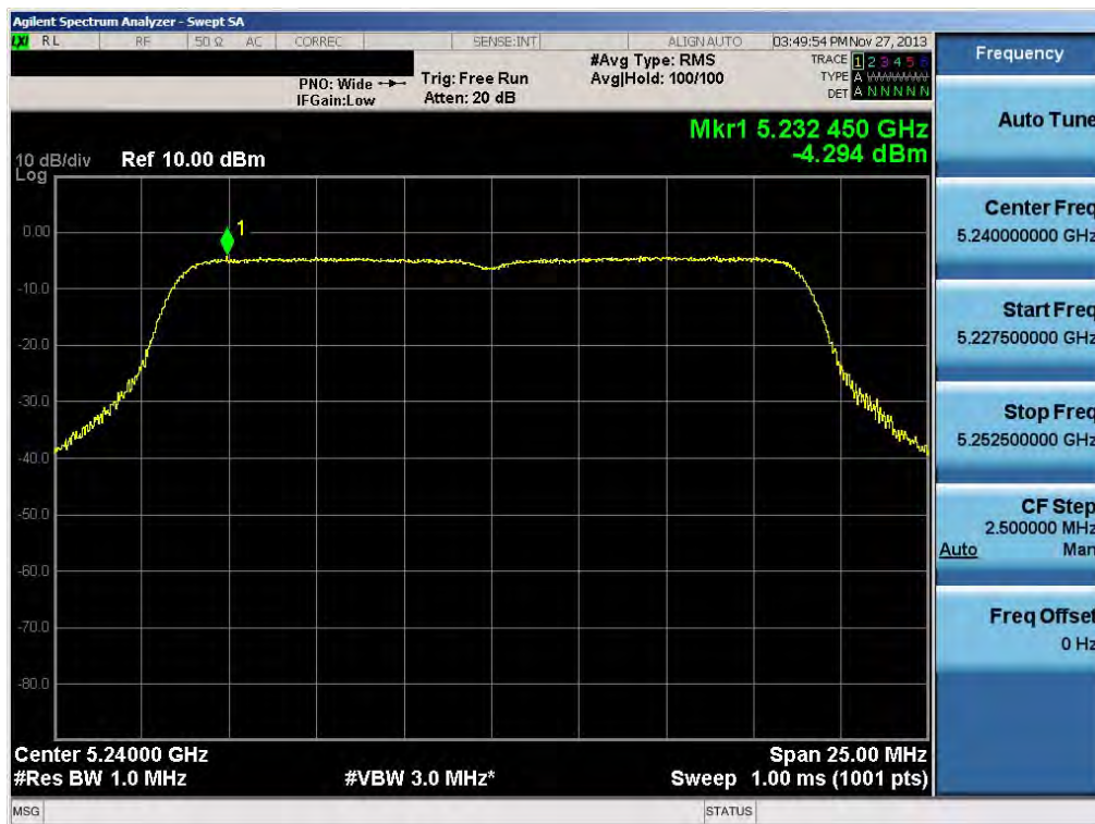
Plot 6-36. Peak Power Spectral Density Plot (20MHz BW 802.11n (UNII Band 1) – Ch. 48)
