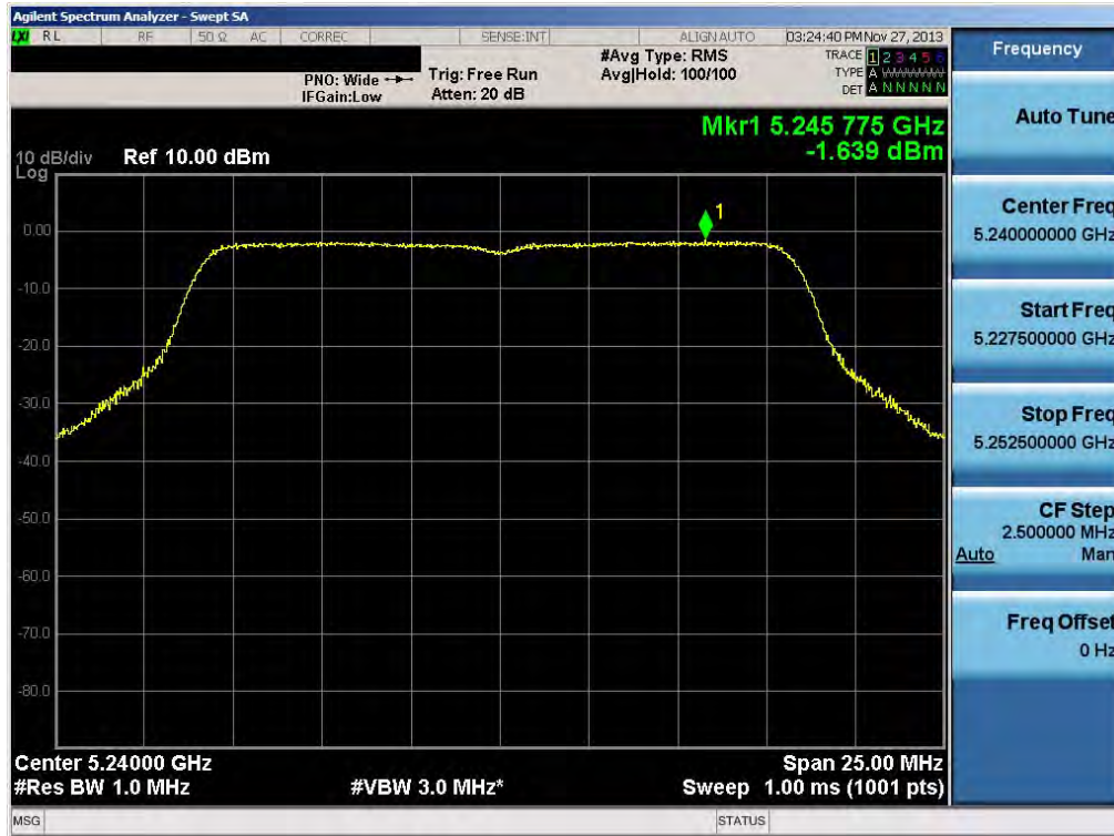
Plot 6-33. Peak Power Spectral Density Plot (802.11a (UNII Band 1) – Ch. 48)
