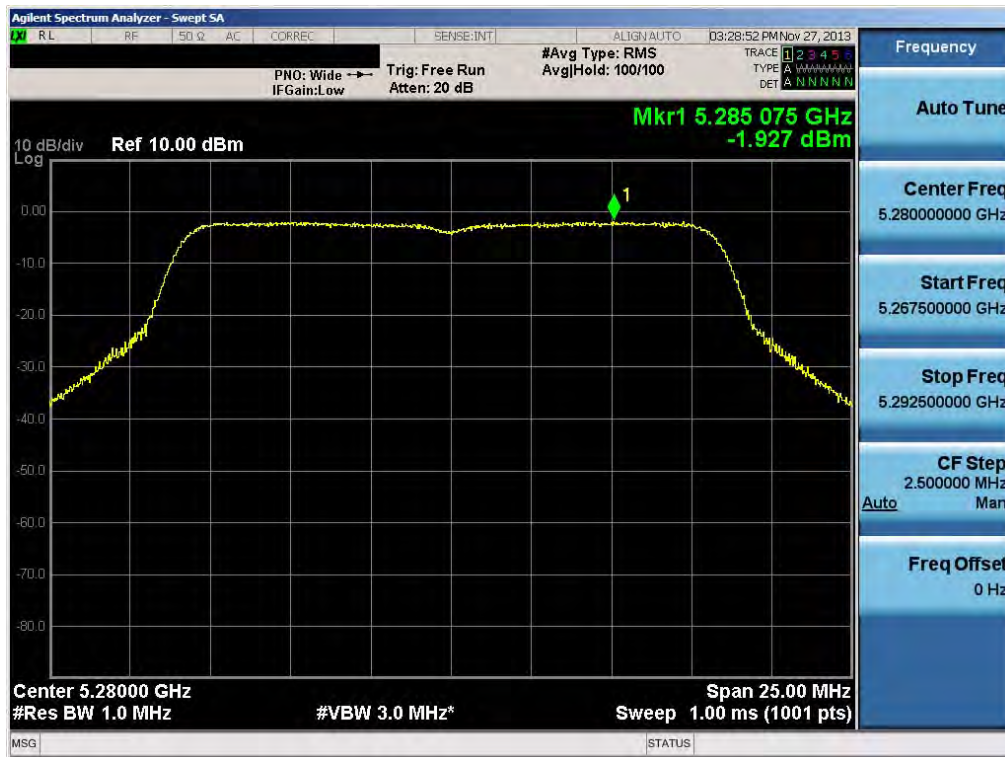
Plot 6-40. Peak Power Spectral Density Plot (802.11a (UNII Band 2A) – Ch. 56)
