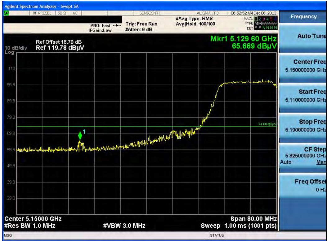
Plot 6-67. Radiated Restricted Lower Band Edge Plot (Peak – UNII Band 1)
