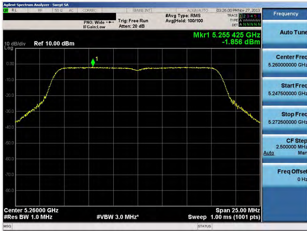
Plot 6-39. Peak Power Spectral Density Plot (802.11a (UNII Band 2A) – Ch. 52)
