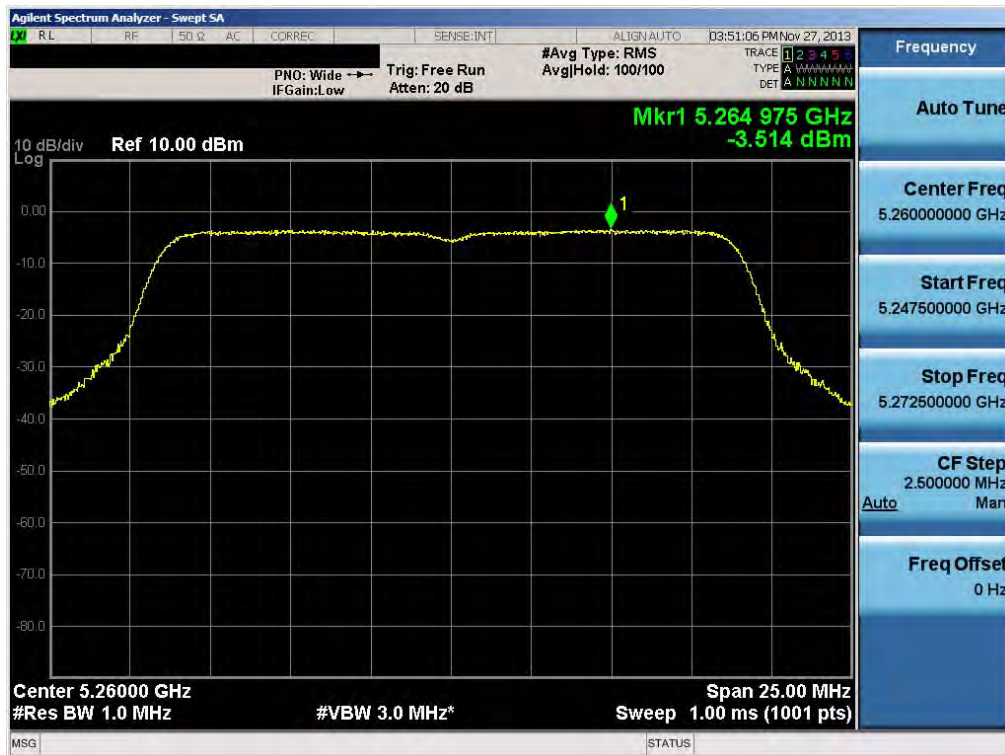
Plot 6-42. Peak Power Spectral Density Plot (20MHz BW 802.11n (UNII Band 2A) – Ch. 52)
