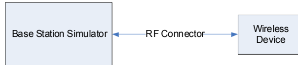
Figure 8-3 Power Measurement Setup
