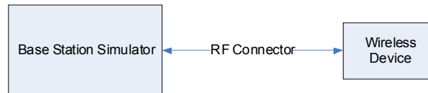
Figure 8-1 Power Measurement Setup
