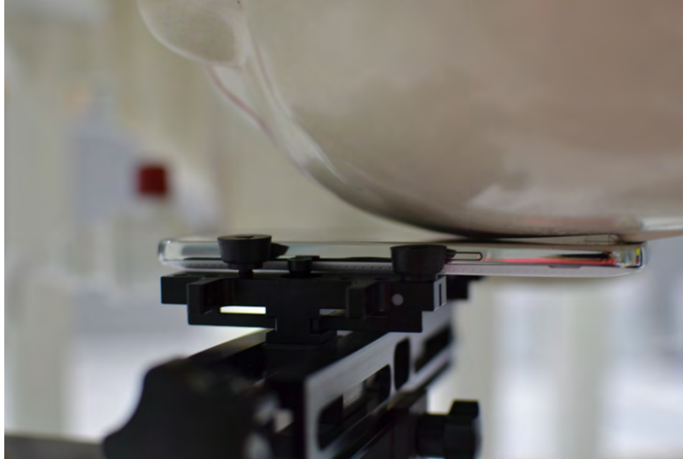
SAR Test Setup Photo 3: Left Cheek
