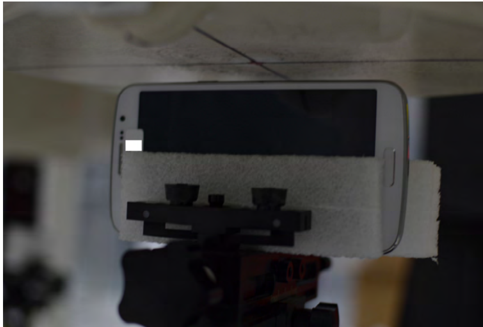
SAR Test Setup Photo 8: Right Edge at 1.0 cm
