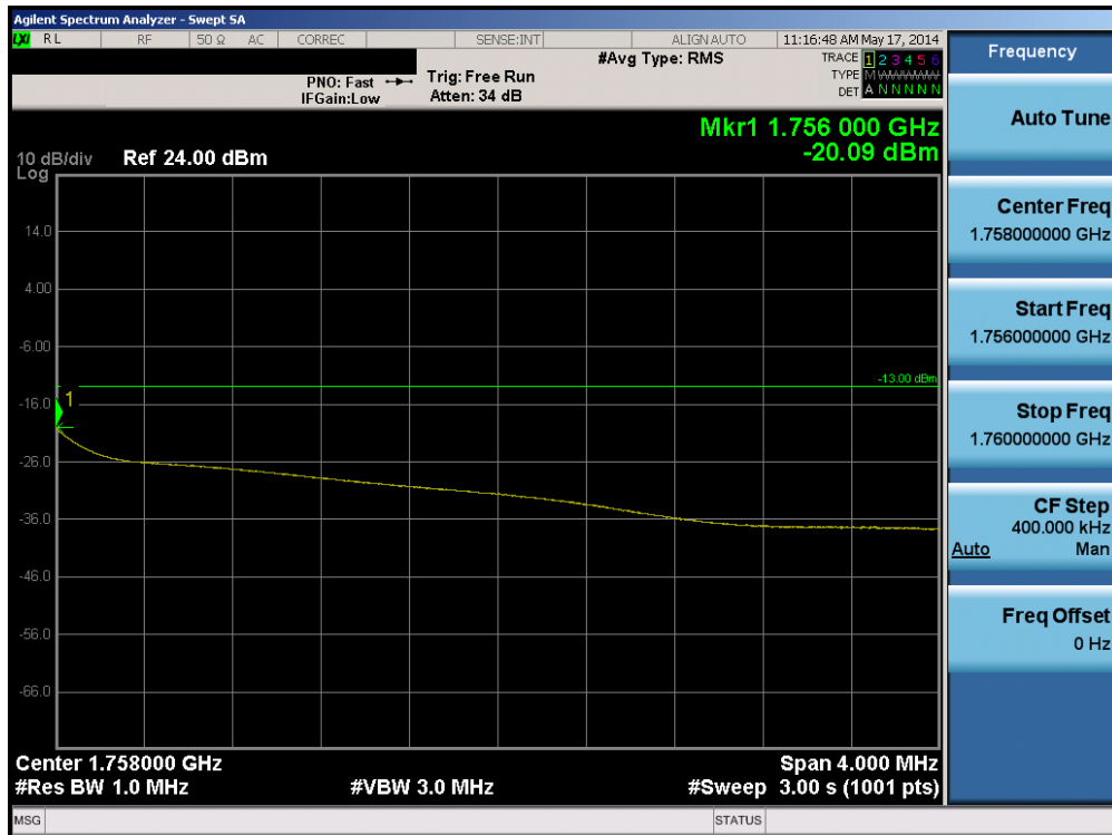
Plot 6-11. 4MHz Span Plot (AWS WCDMA Mode – Ch. 1862)
