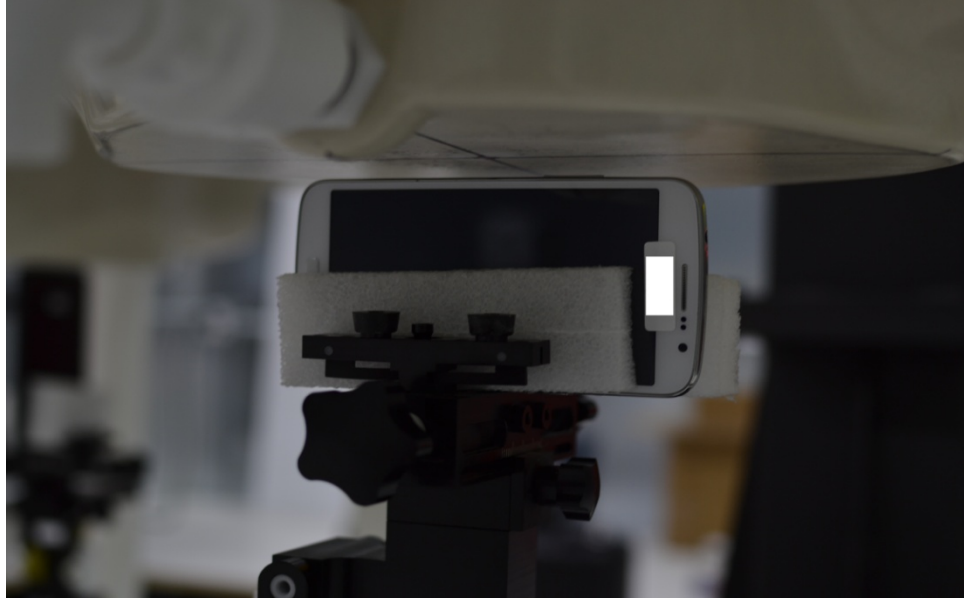
SAR Test Setup Photo 9—Left Edge at 1.0 cm
