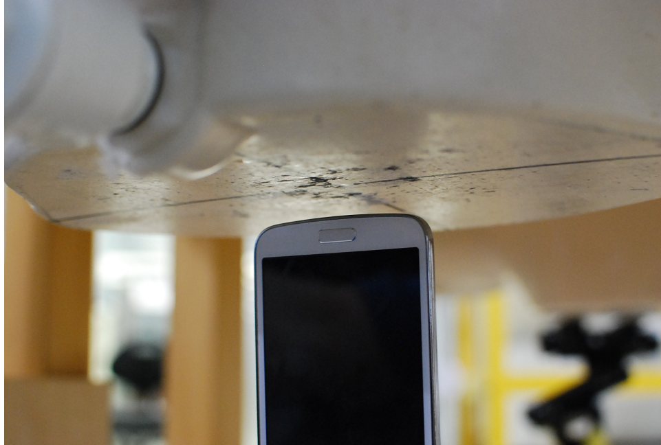
SAR Test Setup Photo 7: Bottom Edge at 1.0 cm
