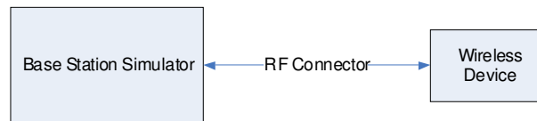
Figure 8-2 Power Measurement Setup
