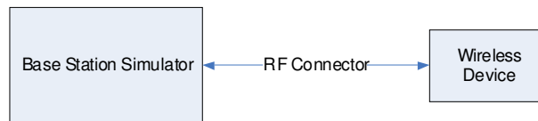
Figure 8-1 Power Measurement Setup
