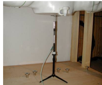
Figure 9-2 System Verification Setup Photo
