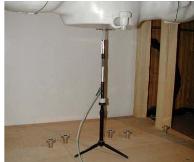
Figure 10-2 System Verification Setup Photo
