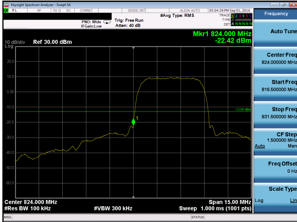
Plot 7-49. Band Edge Plot (Cellular WCDMA Mode – Ch. 4132)
