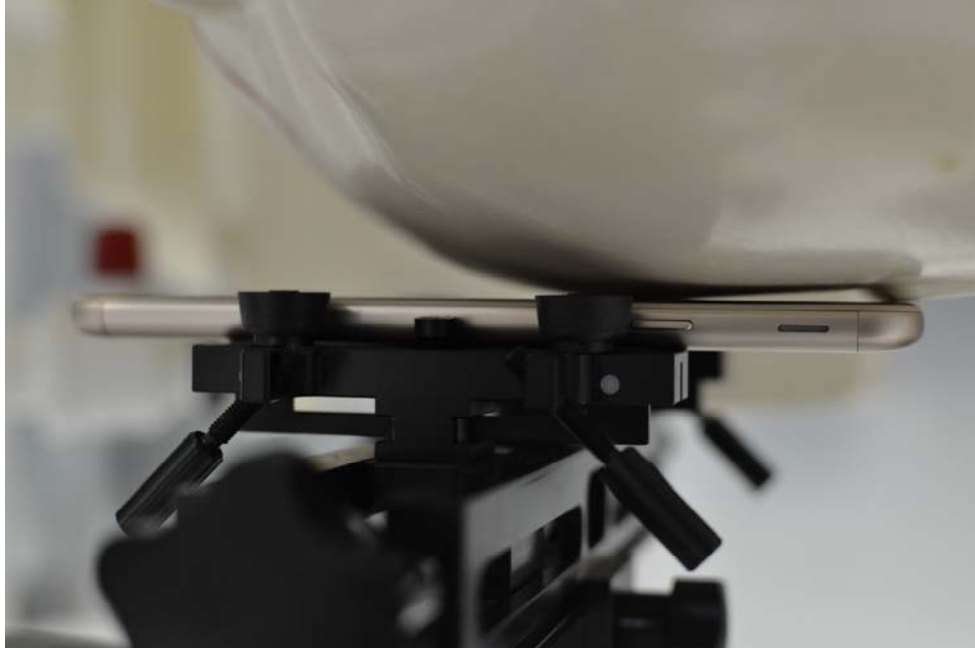
SAR Test Setup Photo 3 – Left Cheek
