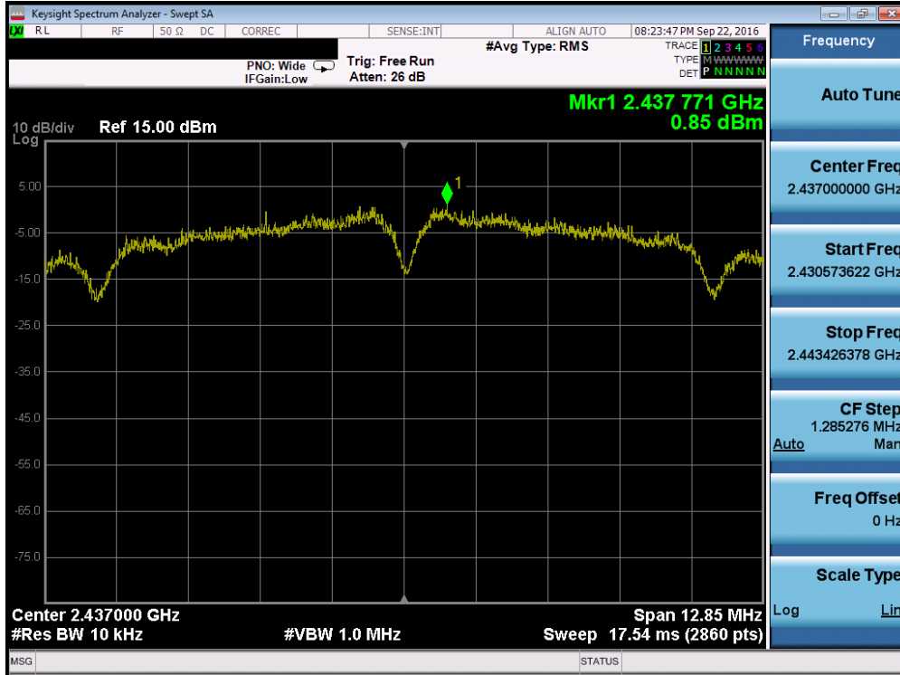
Plot 7-11. Power Spectral Density Plot (802.11b – Ch. 6)
