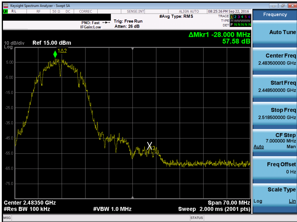
Plot 7-20. Band Edge Plot (802.11b – Ch. 11)
