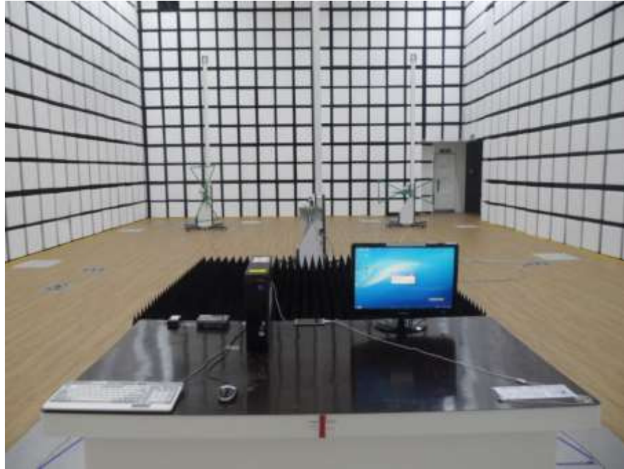
[ Radiated Disturbance for Above 1 GHz – Front ]
