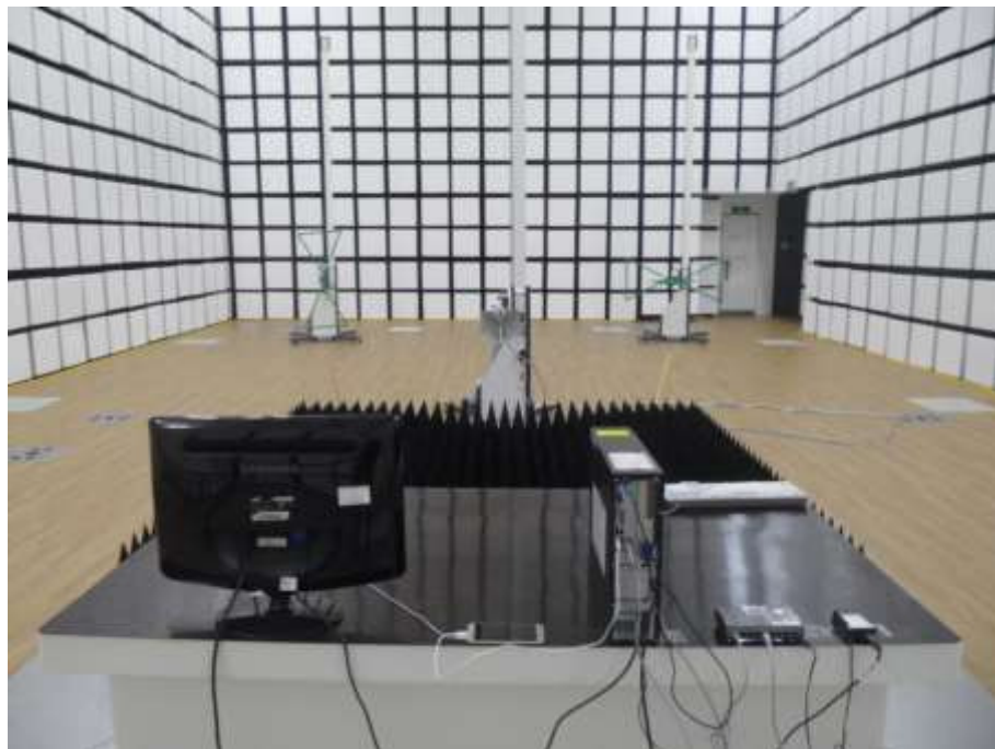
[ Radiated Disturbance for Above 1 GHz – Rear ]
