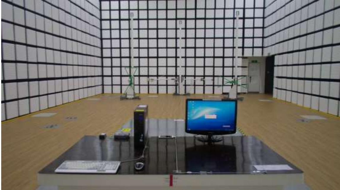
[ Radiated Disturbance for Below 1 GHz – Front ]
