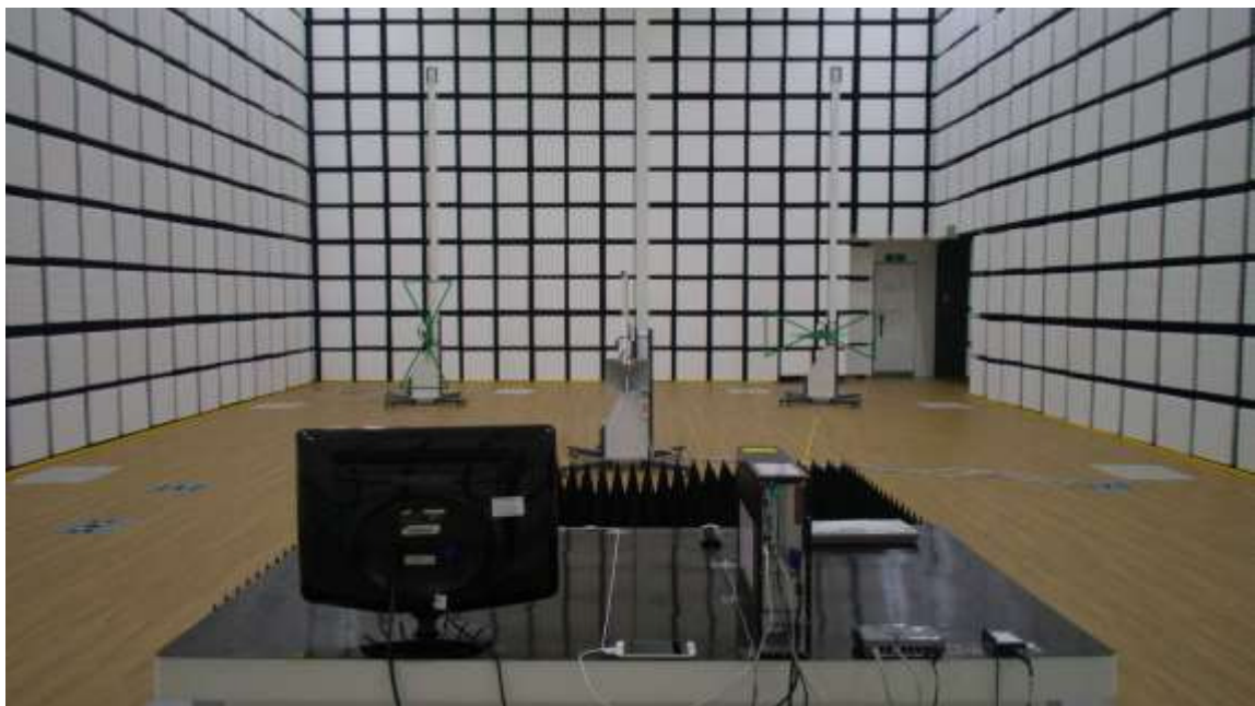
[ Radiated Disturbance for Above 1 GHz – Rear ]
