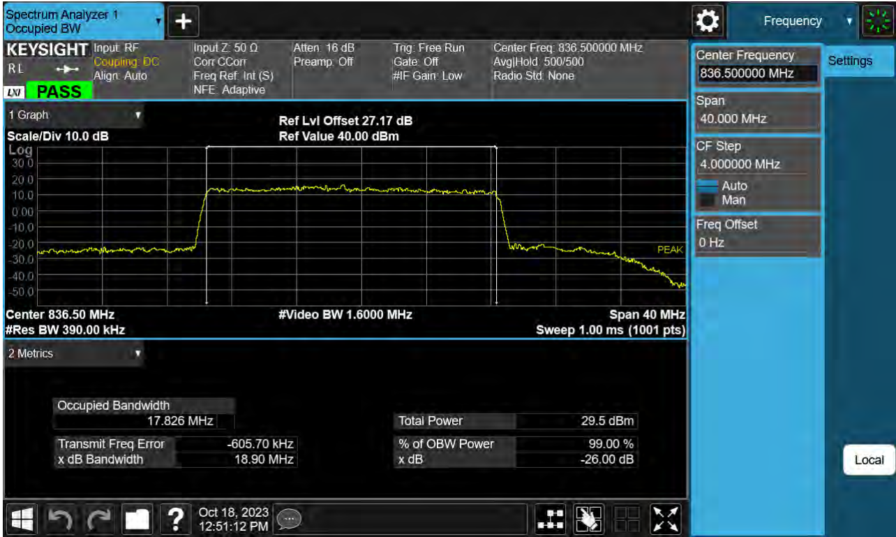
Sub6 n26. Occupied Bandwidth Plot (20 M BW Ch.167300 16QAM RB 100_0)
