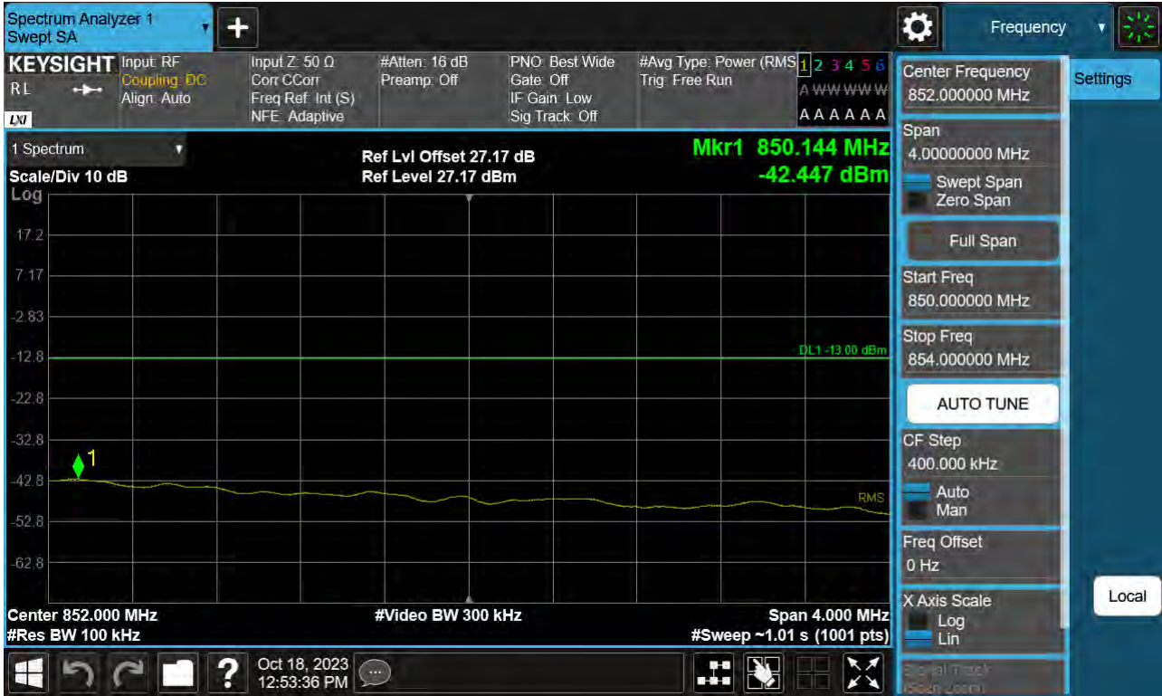
Sub6 n26. Upper Extended Band Edge Plot (20 M BW Ch.167800 BPSK_RB 100_0)
