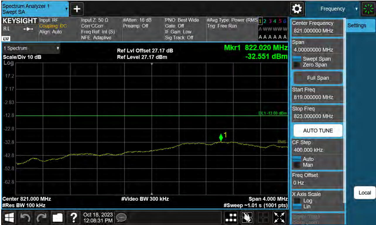
Sub6 n26. Lower Extended Band Edge Plot (5 M BW Ch.165300 BPSK_RB 25_0)
