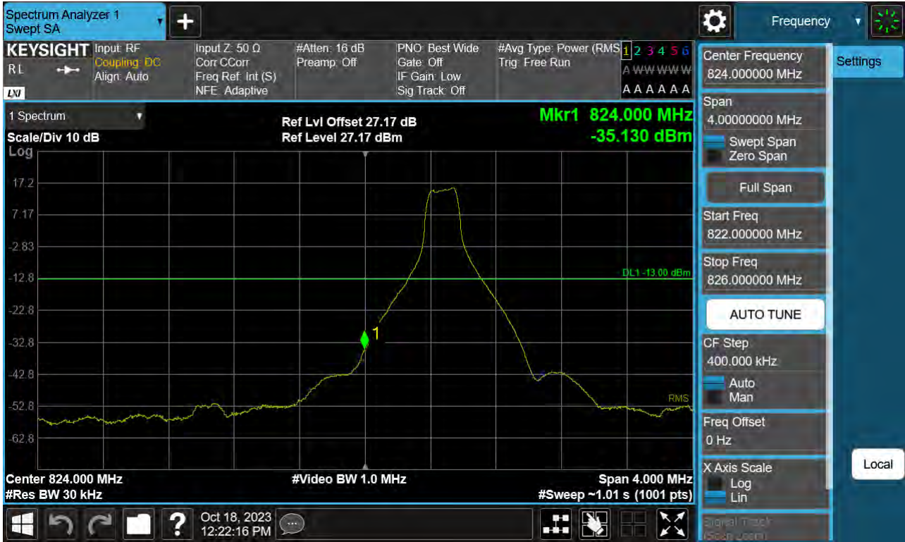
Sub6 n26. Lower Band Edge Plot (15 M BW Ch.166300 BPSK_RB 1_Offset 0)
