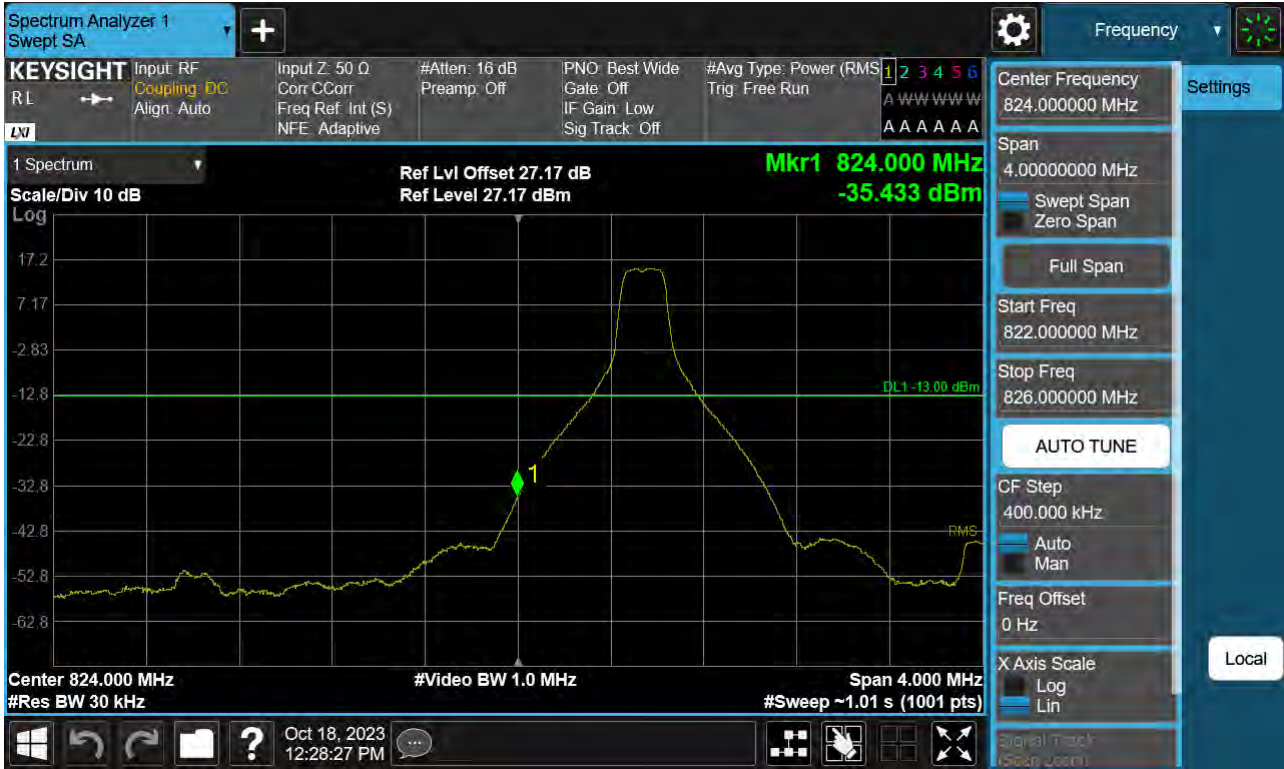
Sub6 n26. Lower Band Edge Plot (20 M BW Ch.166800 BPSK_RB 1_Offset 0)
