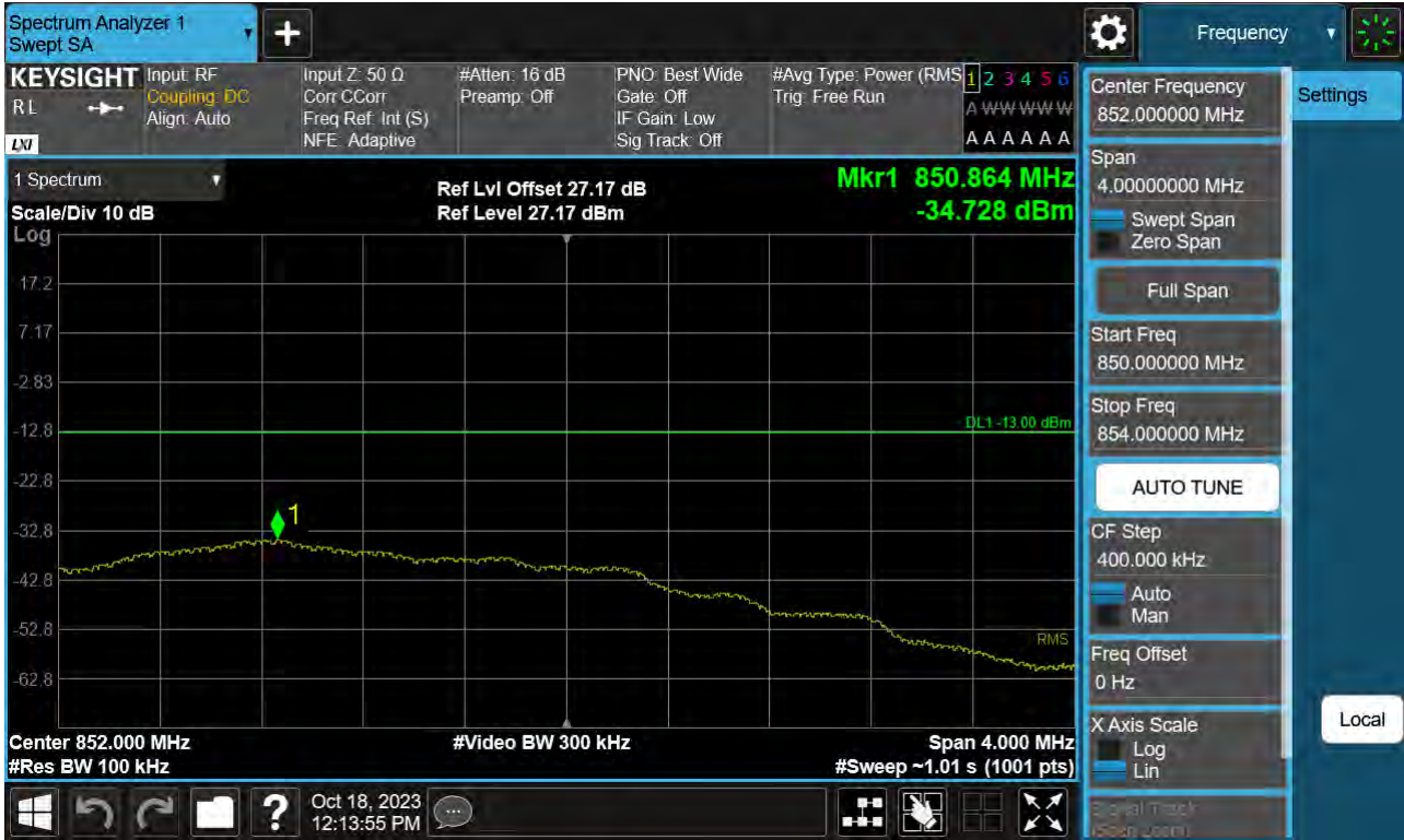
Sub6 n26. Upper Extended Band Edge Plot (5 M BW Ch.169300 BPSK_RB 25_0)
