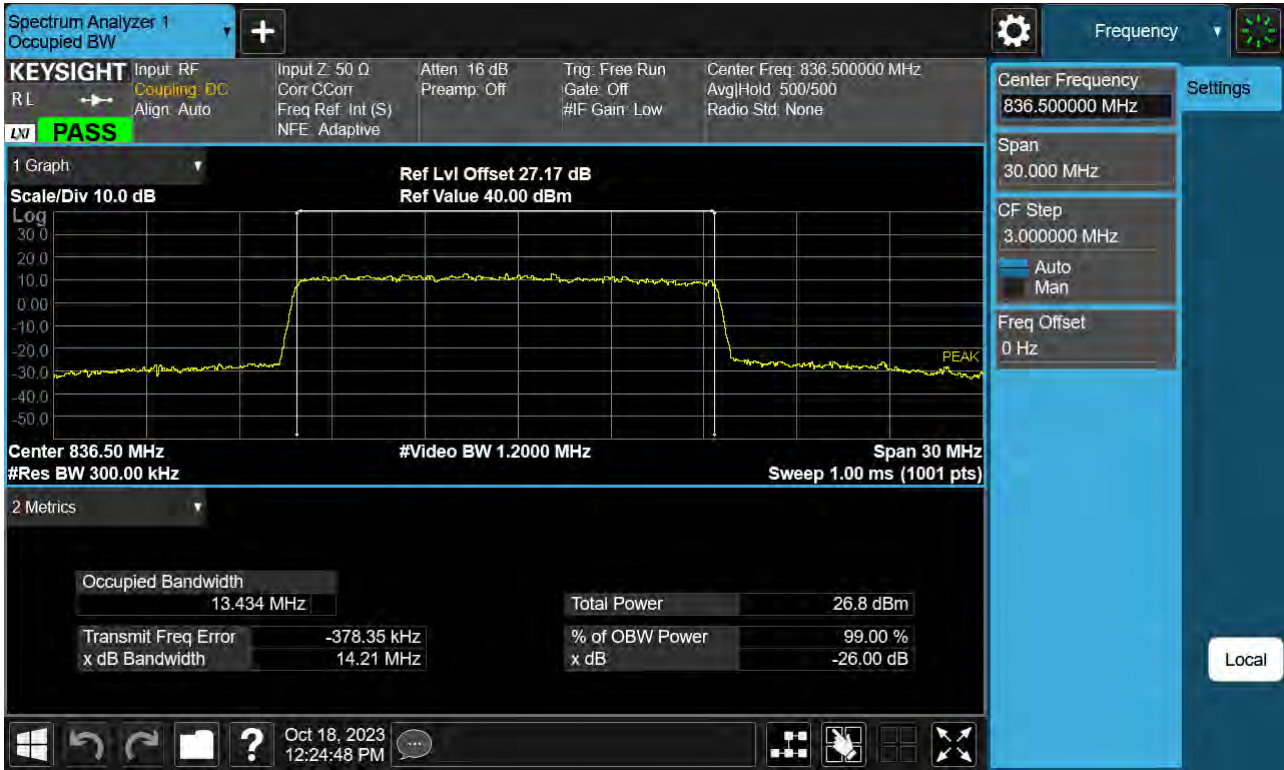
Sub6 n26. Occupied Bandwidth Plot (15 M BW Ch.167300 256QAM RB 75_0)
