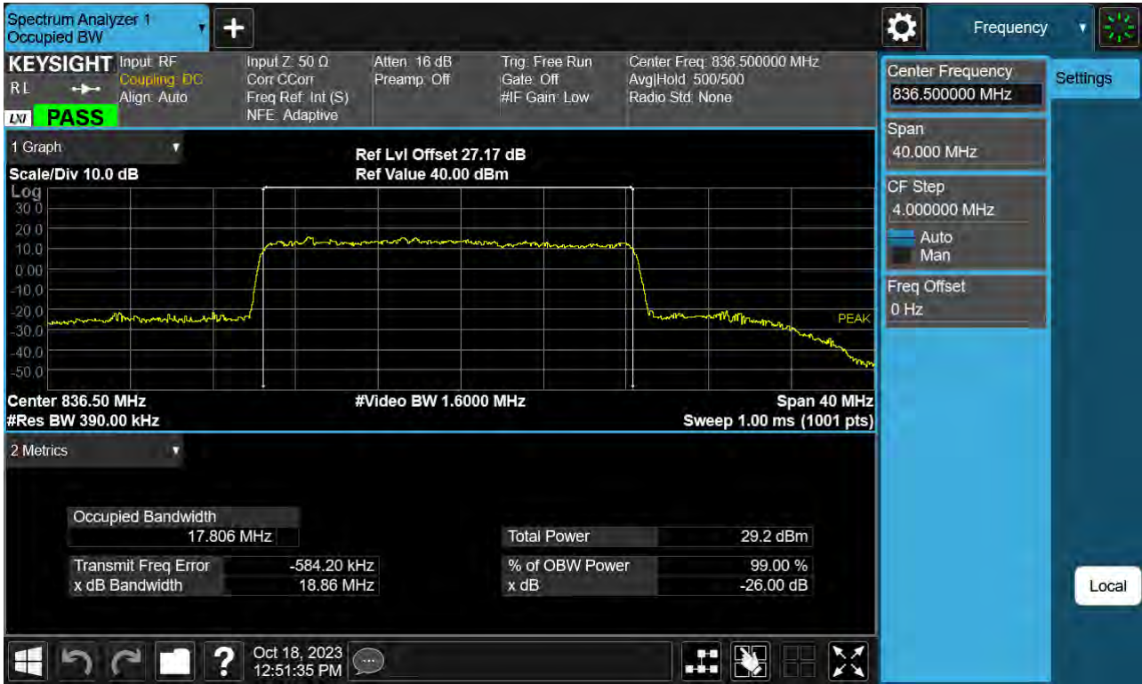
Sub6 n26. Occupied Bandwidth Plot (20 M BW Ch.167300 64QAM RB 100_0)
