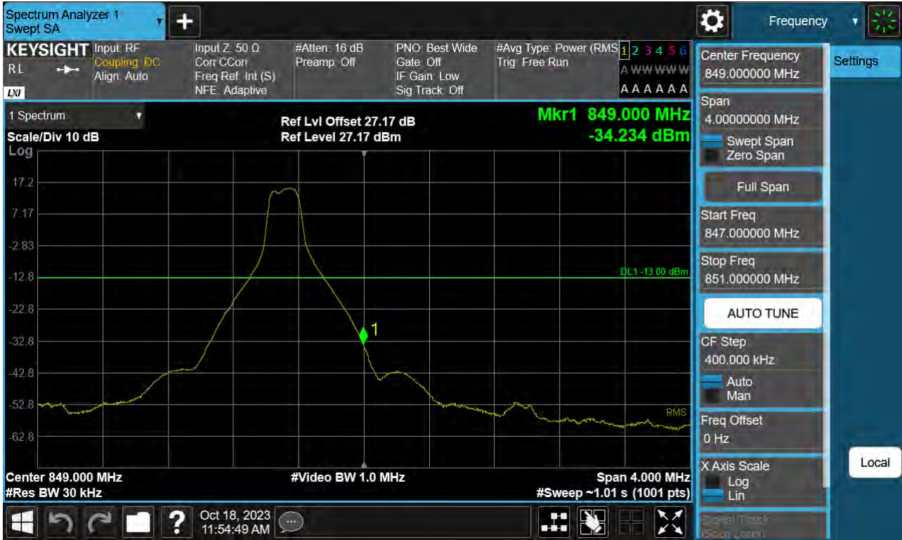
Sub6 n5. Upper Band Edge Plot (15 M BW Ch.168300 BPSK_RB1_Offset 78)
