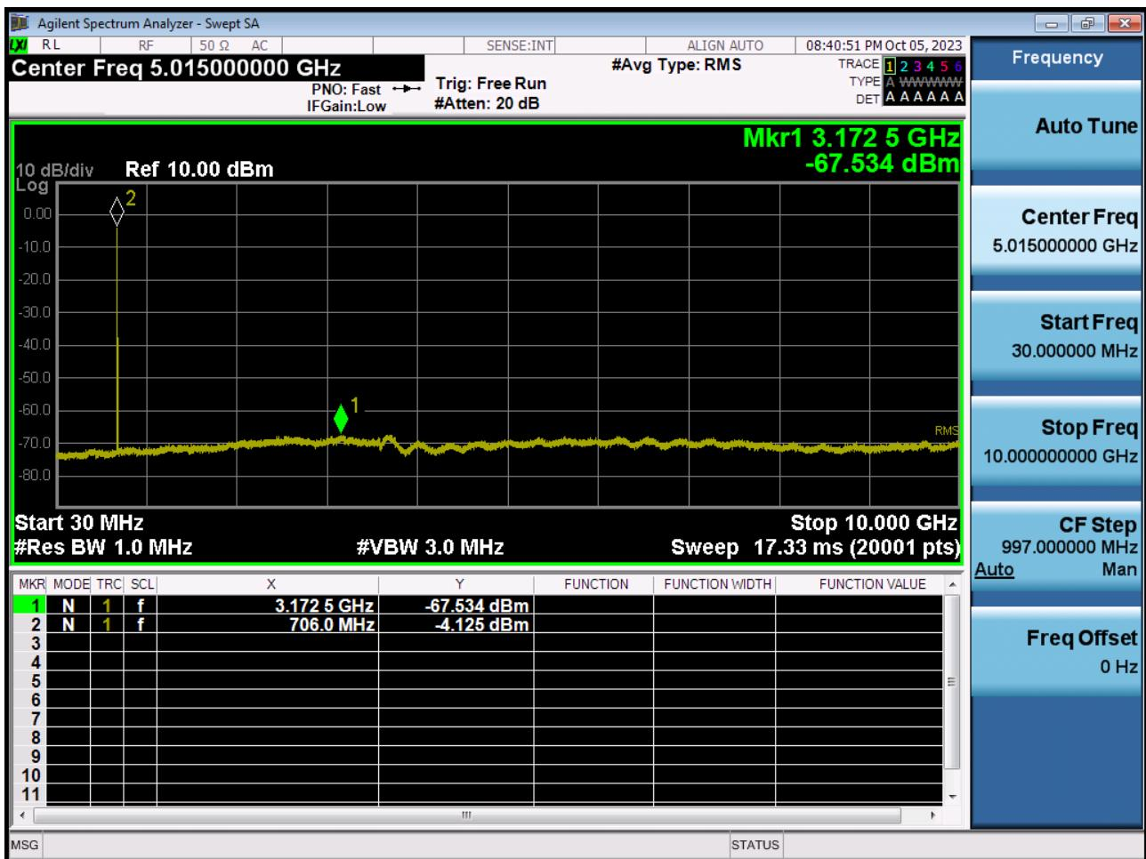
BAND 12/17. Conducted Spurious Plot \_ (23155ch\_5 MHz\_QPSK\_RB 1\_0)
