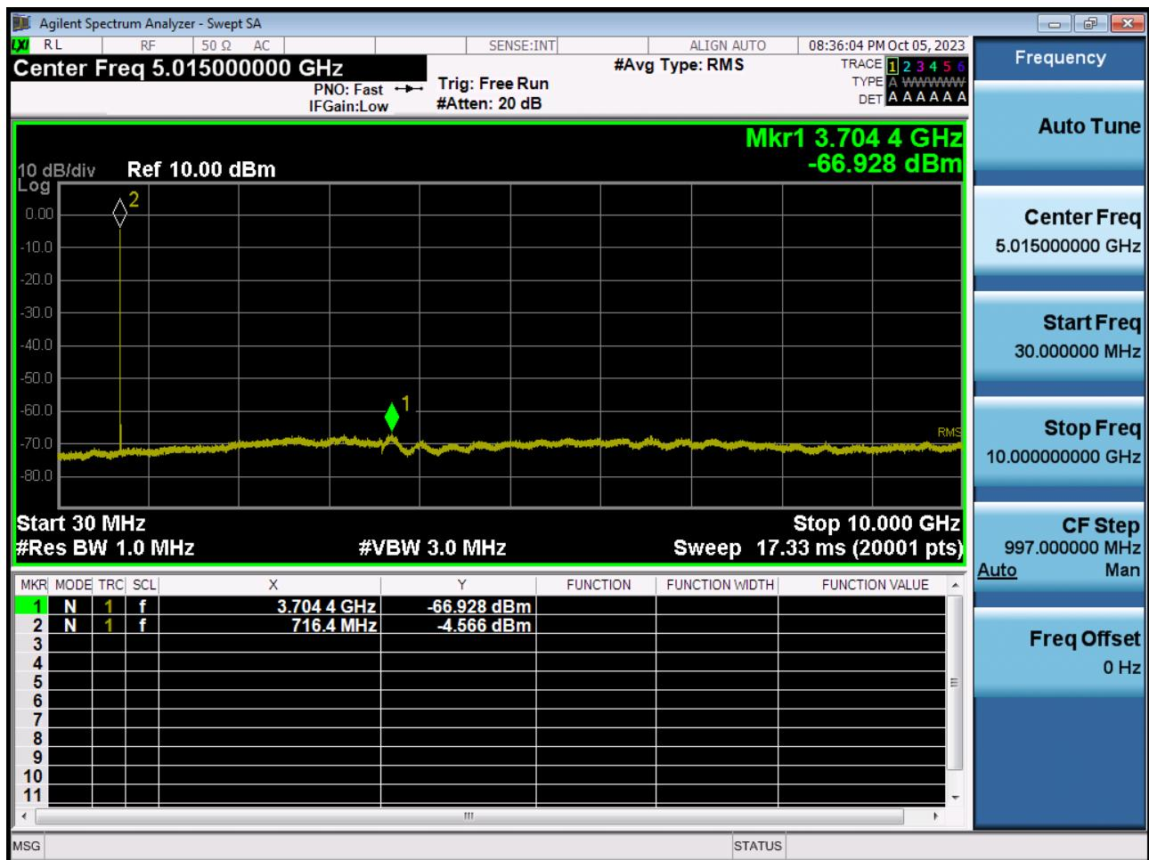
BAND 12/17. Conducted Spurious Plot \_ (23035ch\_5 MHz\_QPSK\_RB 1\_0)
