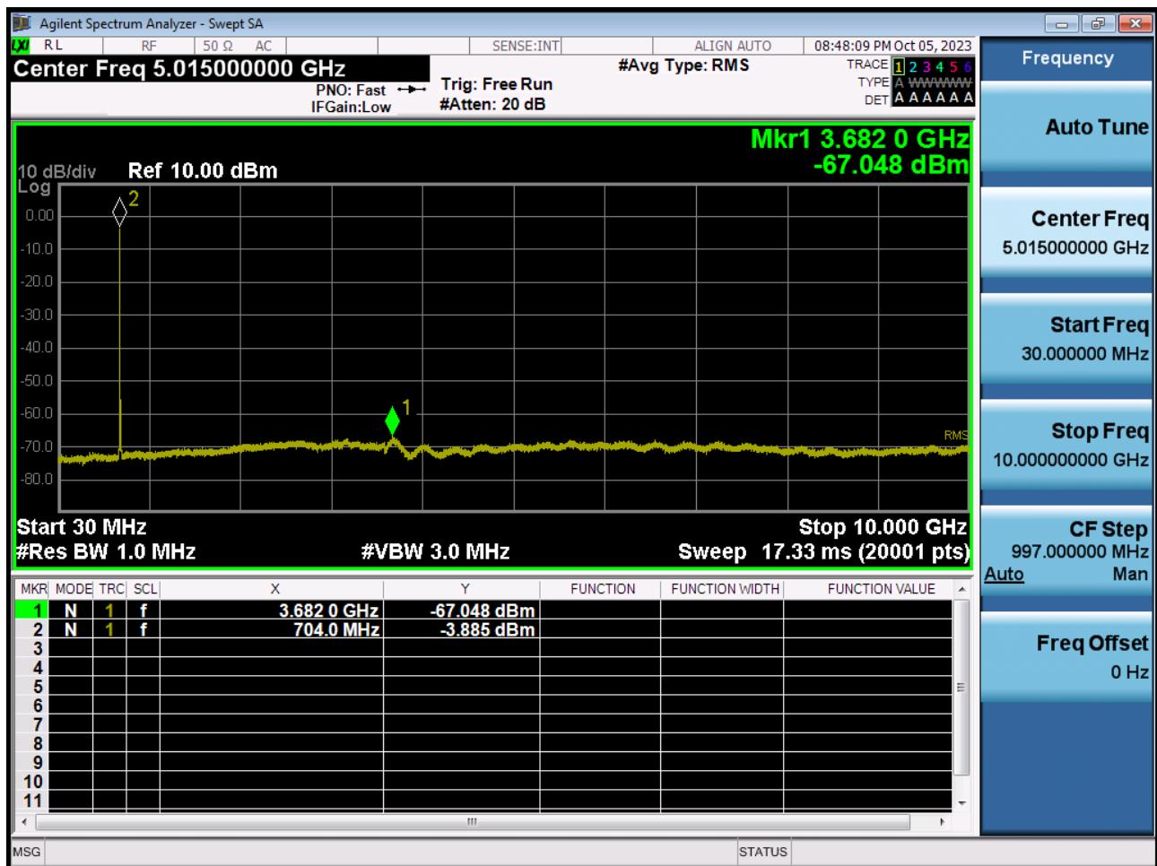
BAND 12/17. Conducted Spurious Plot \_ (23130ch\_10 MHz\_QPSK\_RB 1\_0)
