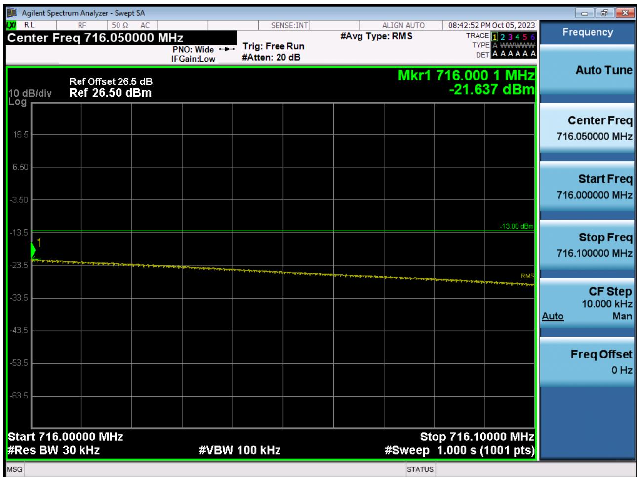
BAND 12/17. Upper Band Edge Plot (5 M BW Ch.23155 QPSK\_RB1\_Offset 24)\_2
