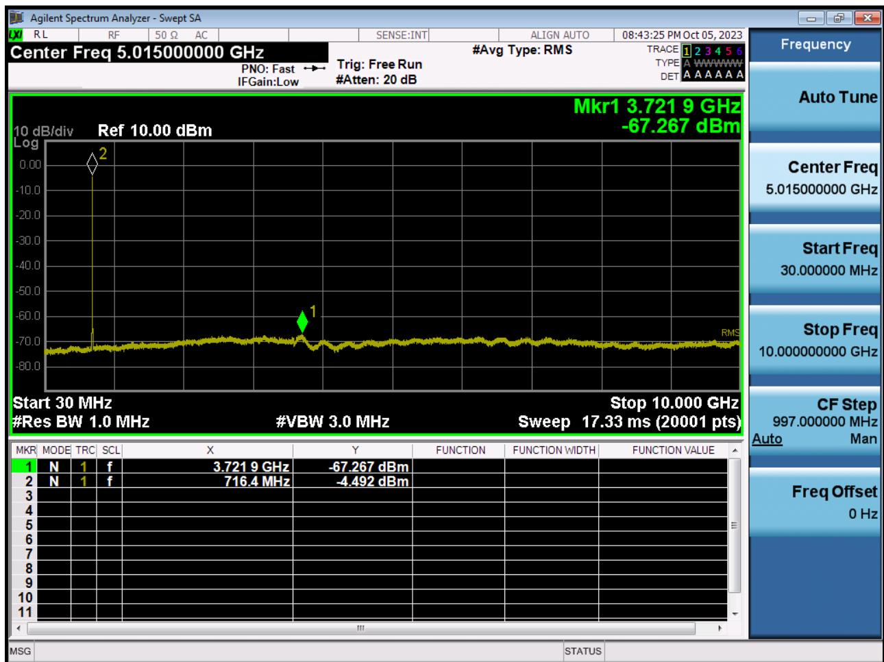
BAND 12/17. Conducted Spurious Plot \_ (23060ch\_10 MHz\_QPSK\_RB 1\_0)
