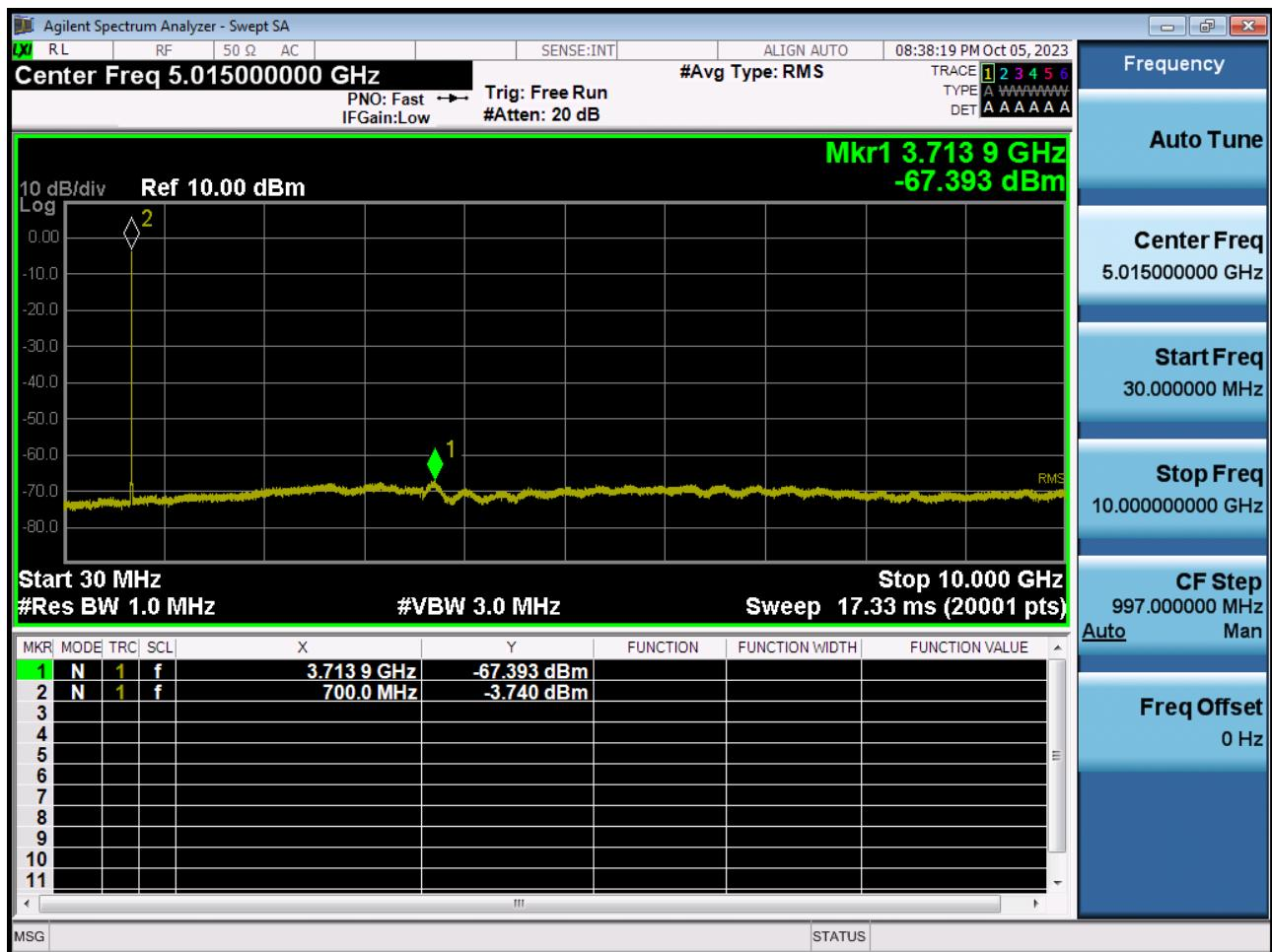
BAND 12/17. Conducted Spurious Plot \_ (23095ch\_5 MHz\_QPSK\_RB 1\_0)
