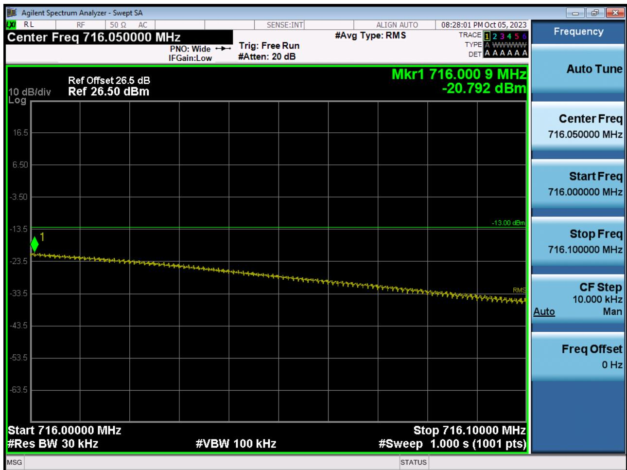
BAND 12. Upper Band Edge Plot (1.4 M BW Ch.23173 QPSK\_RB1\_Offset 5)\_2
