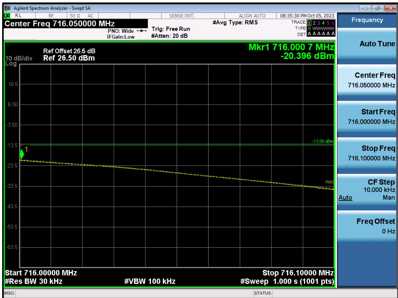
BAND 12. Upper Band Edge Plot (3 M BW Ch.23165 QPSK\_RB1\_Offset 14)-2
