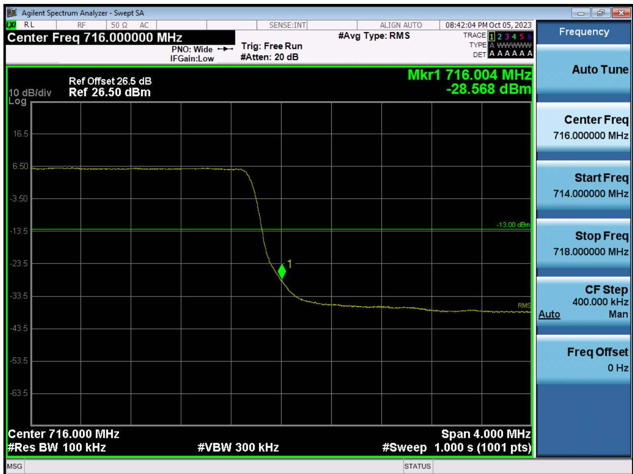
BAND 12/17. Upper Extended Band Edge Plot (5 M BW Ch.23155 QPSK\_RB25\_0)
