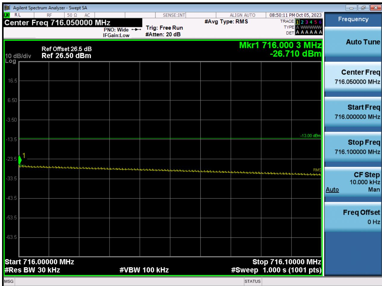
BAND 12/17. Upper Band Edge Plot (10 M BW Ch.23130 QPSK\_RB1\_Offset 49)\_2
