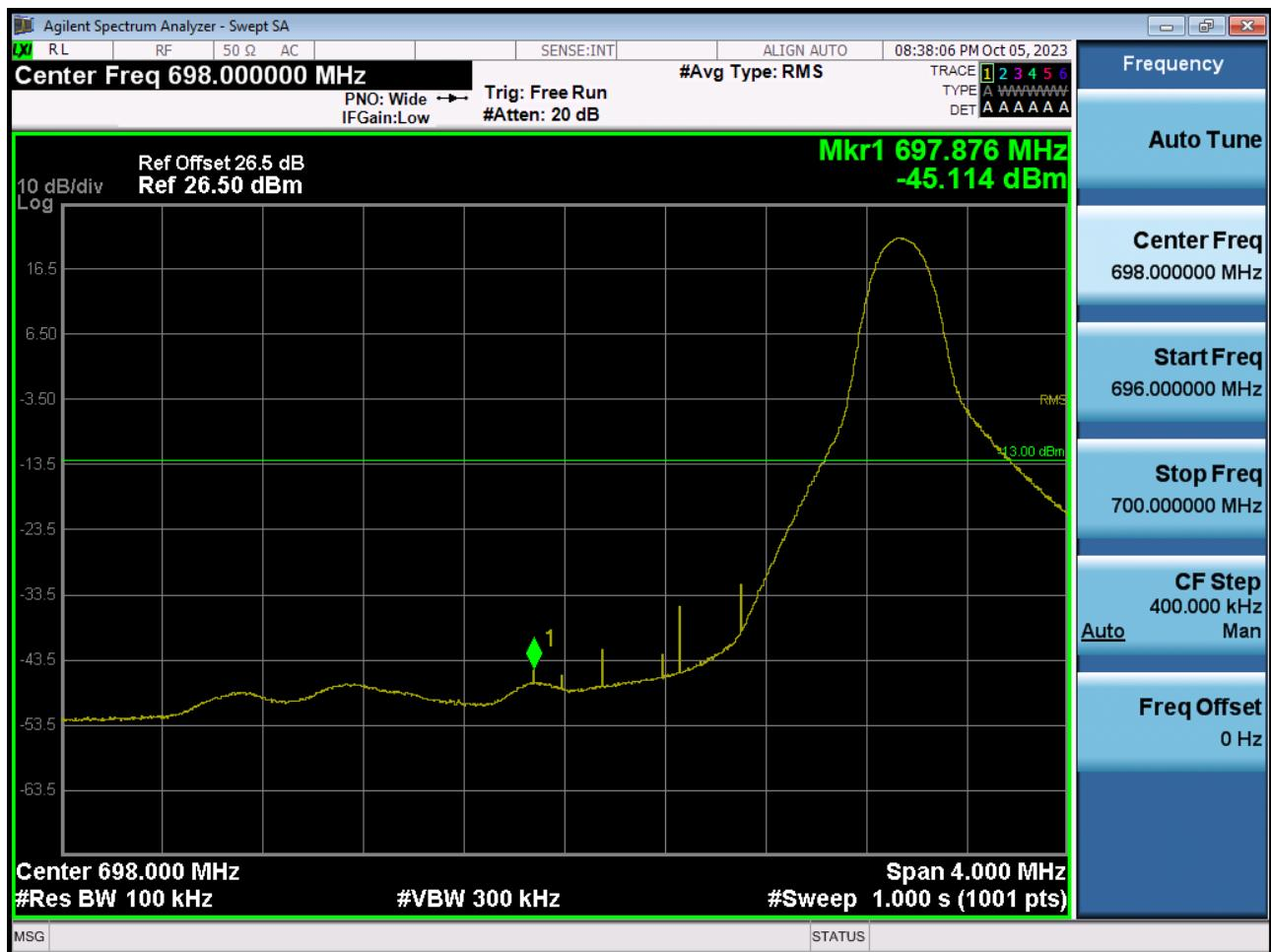
BAND 12/17. Lower Band Edge Plot (5 M BW Ch.23035 QPSK\_RB25\_Offset 0)
