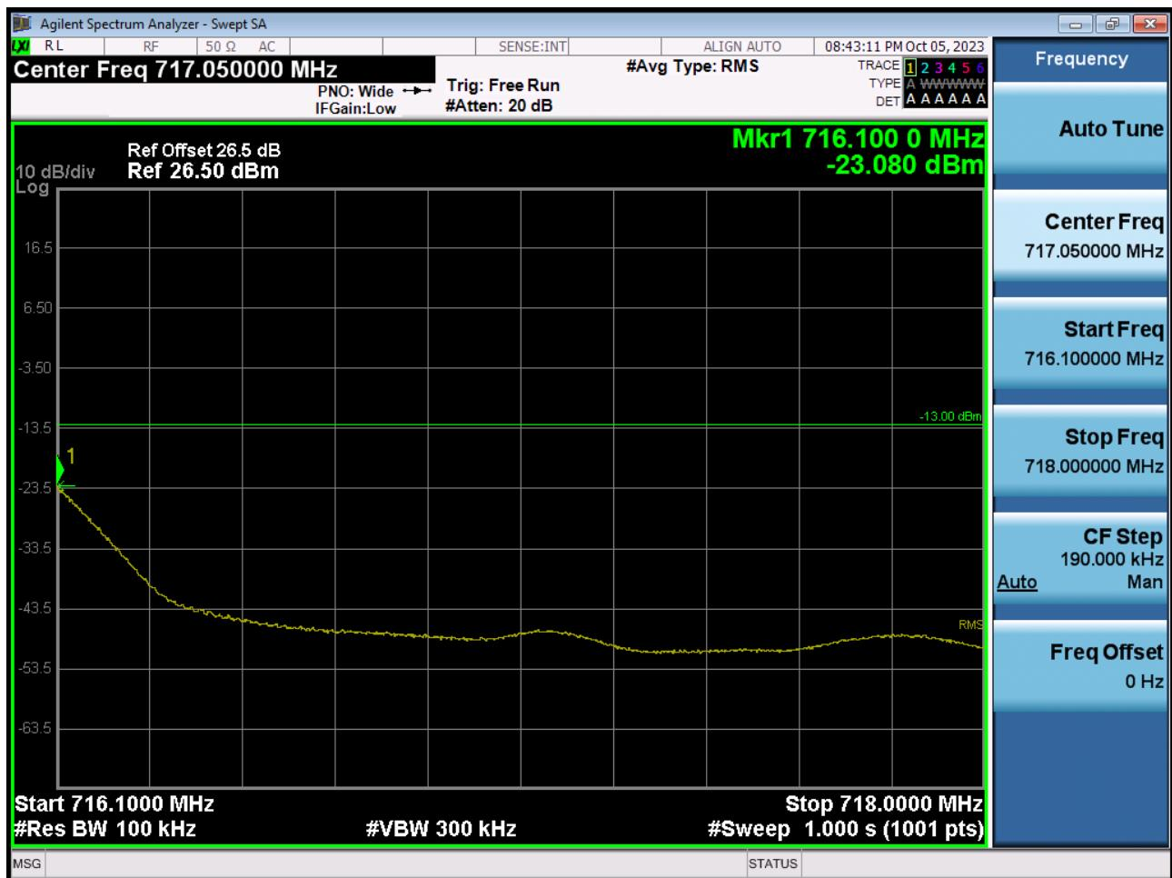
BAND 12/17. Upper Band Edge Plot (5 M BW Ch.23155 QPSK\_RB25\_Offset 0)
