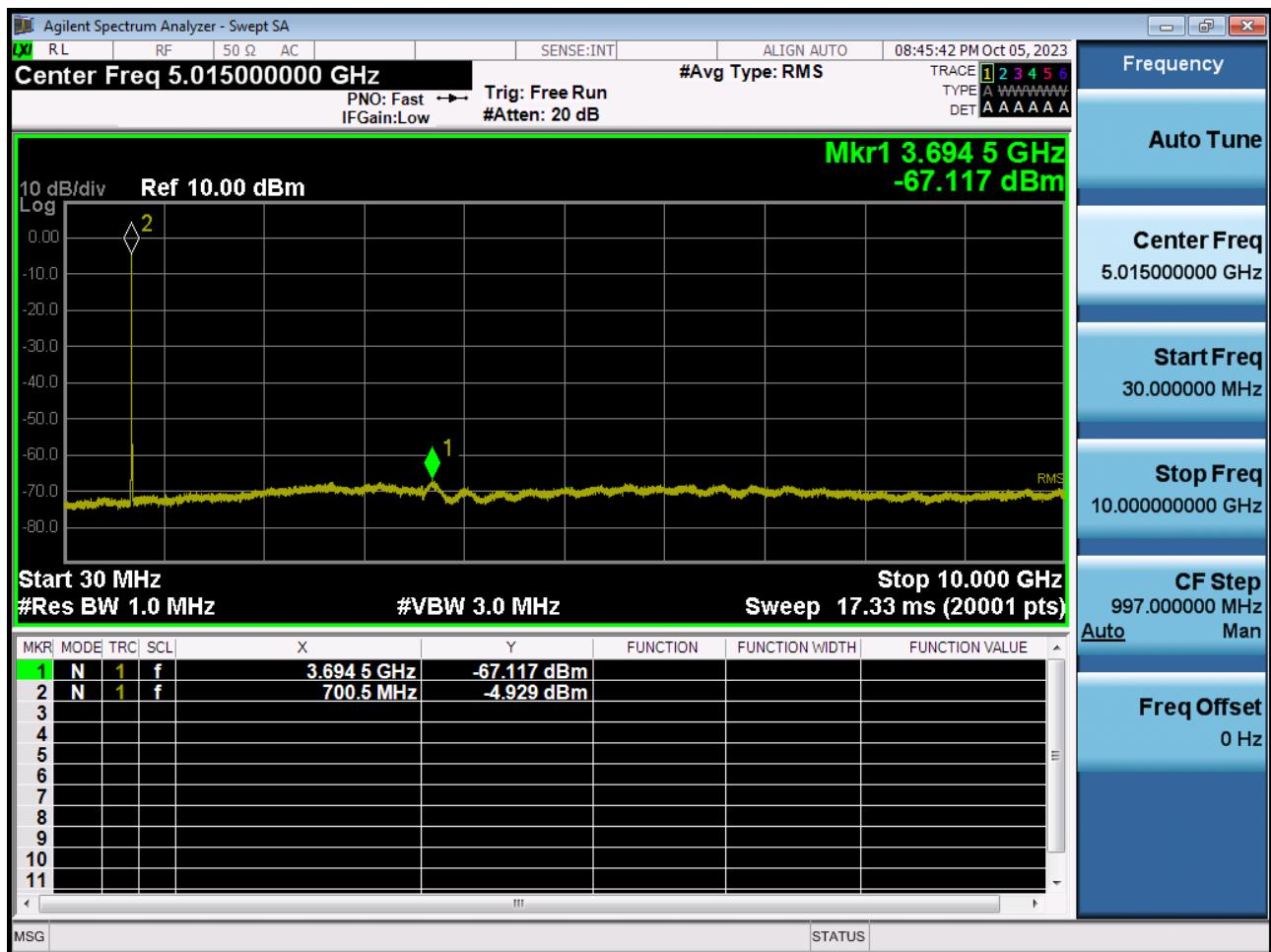
BAND 12/17. Conducted Spurious Plot \_ (23095ch\_10 MHz\_QPSK\_RB 1\_0)
