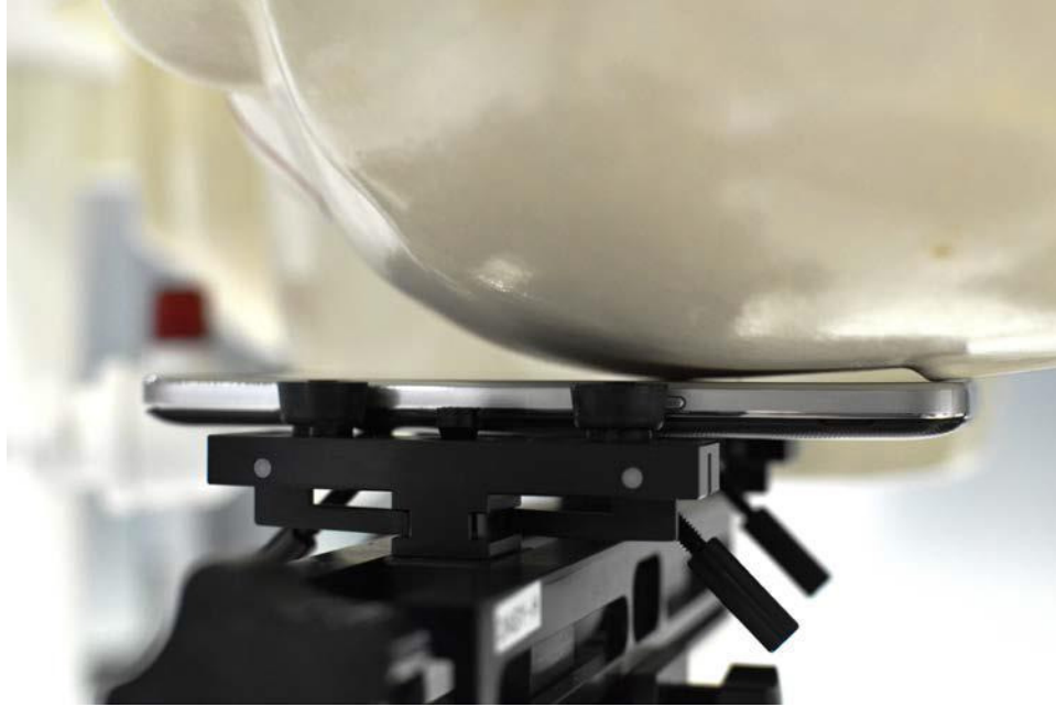
SAR Test Setup Photo 3 – Left Cheek
