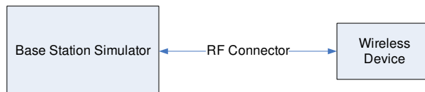
Figure 9-2 Power Measurement Setup
