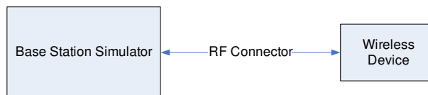
Figure 9-1 Power Measurement Setup
