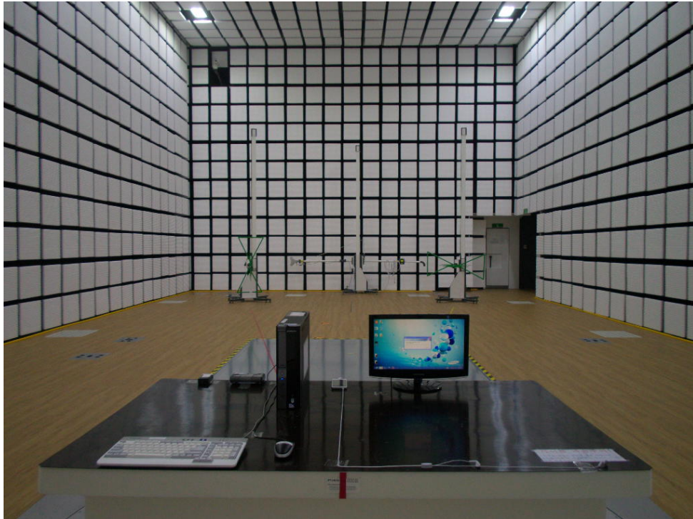
[ Radiated Disturbance for Below 1 GHz – Front ]
