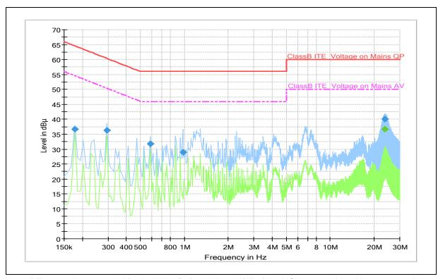
Note 1) Two graphs measured for both Live(L1) and Neutral(N) of the LISN are combined into one graph.
