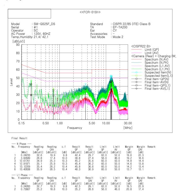
Note 1) Two graphs measured for both Live(L1) and Neutral(N) of the LISN are combined into one graph Note 2) Level (QP and/or CAV) = Meter Reading (QP and/or CAV) + Corr. (LISN Insertion Loss + Cable Loss) Margin (QP and/or CAV) = Limit – Level (QP and/or CAV) QP = Quasi-Peak, CAV = CISPR-Average, Corr. = Correction Factor.
