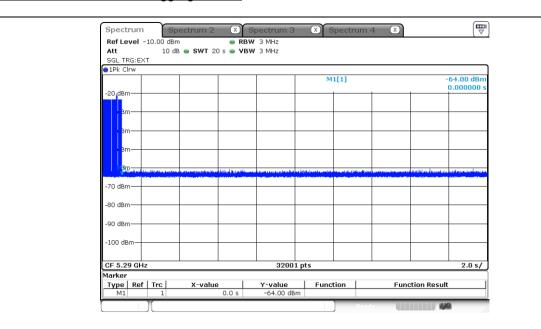
Channel move time = Not detected Closing time = Not detected
