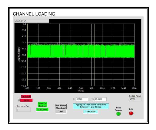
The level of traffic loading on the channel by the EUT is 31.94%
