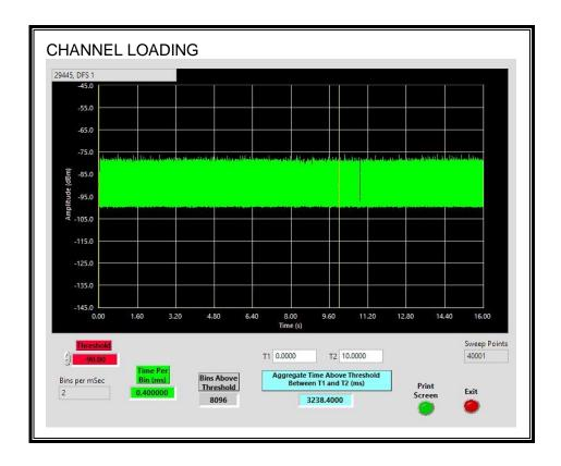
The level of traffic loading on the channel by the EUT is 32.38%
