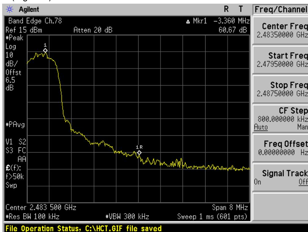
Test Plots with hopping (GFSK)
