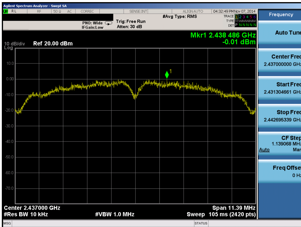
Plot 6-11. Power Spectral Density Plot (802.11b – Ch. 6)
