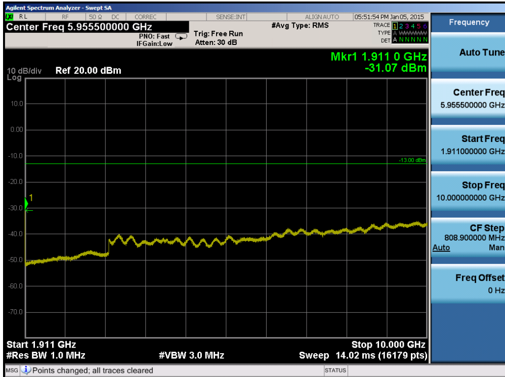
Plot 6-44. Conducted Spurious Plot (Band 2 – 10.0MHz QPSK – RB Size 1, RB Offset 0 – High Channel)
