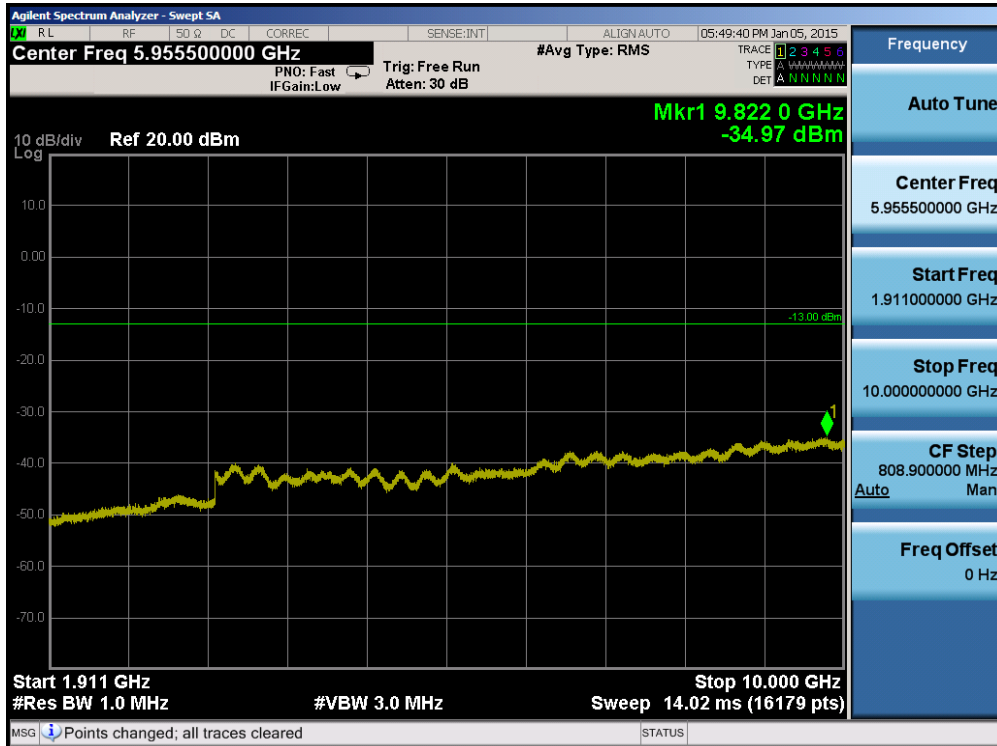
Plot 6-38. Conducted Spurious Plot (Band 2 – 10.0MHz QPSK – RB Size 1, RB Offset 0 – Low Channel)
