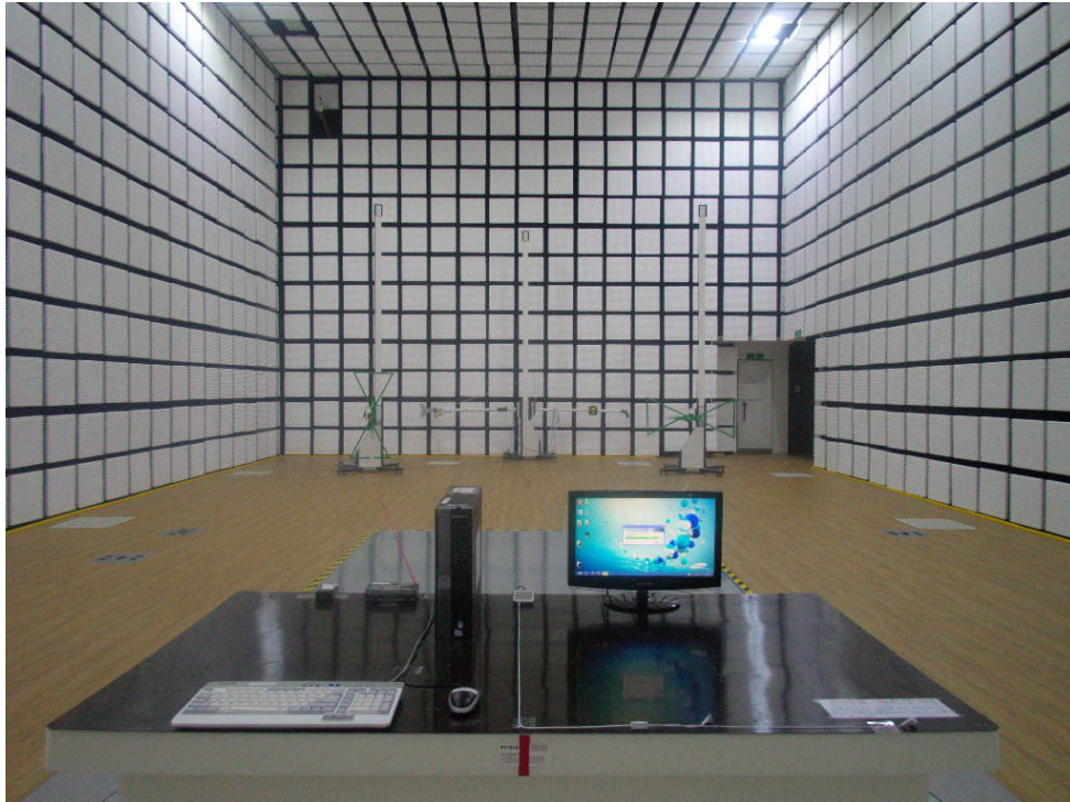
[ Radiated Disturbance for Below 1 GHz – Front ]
