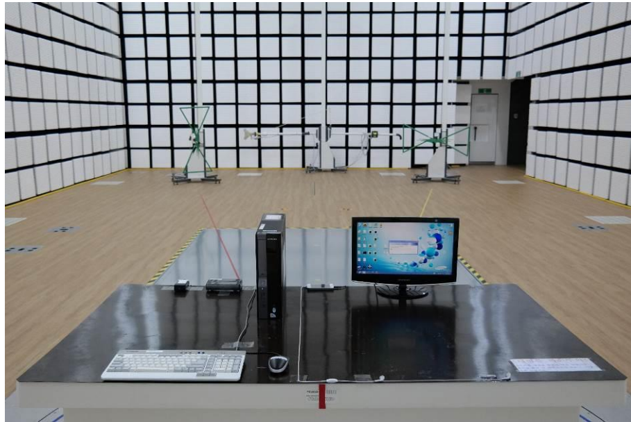
[ Radiated Disturbance for Below 1 GHz – Front ]
