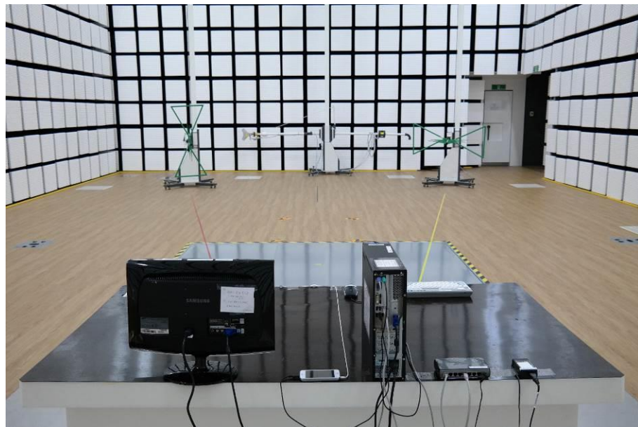
[ Radiated Disturbance for Below 1 GHz – Rear ]
