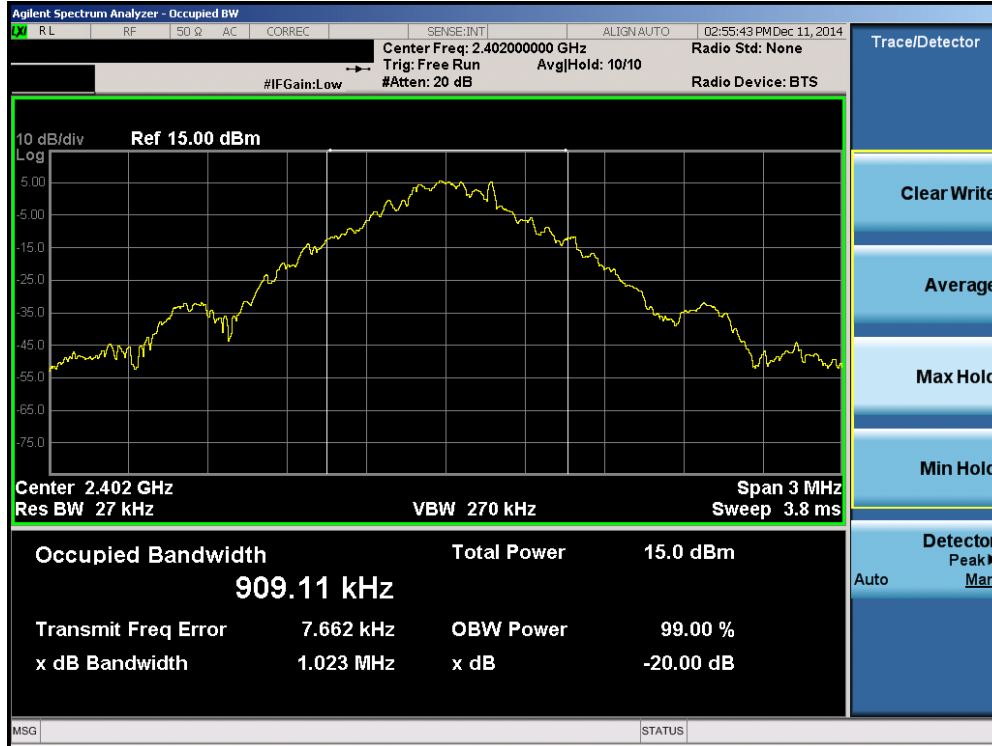
Plot 6-1. 20dB Bandwidth Plot (Bluetooth, 1Mbps – Ch. 0)
