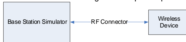
Figure 8-2 Power Measurement Setup
