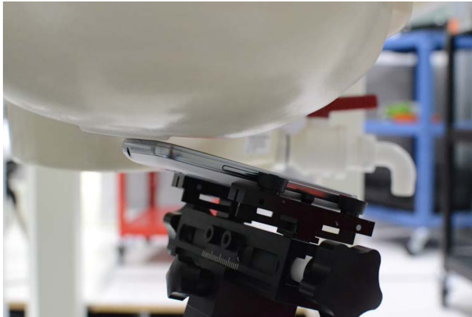
SAR Test Setup Photo 2: Right Tilt
