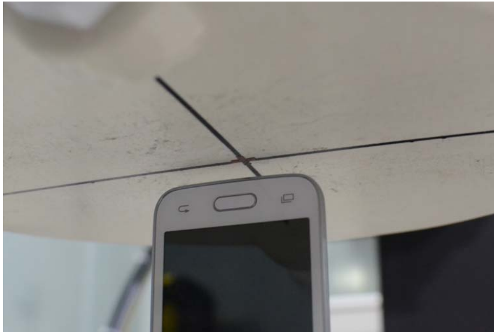
SAR Test Setup Photo 10: Bottom Edge at 10 mm
