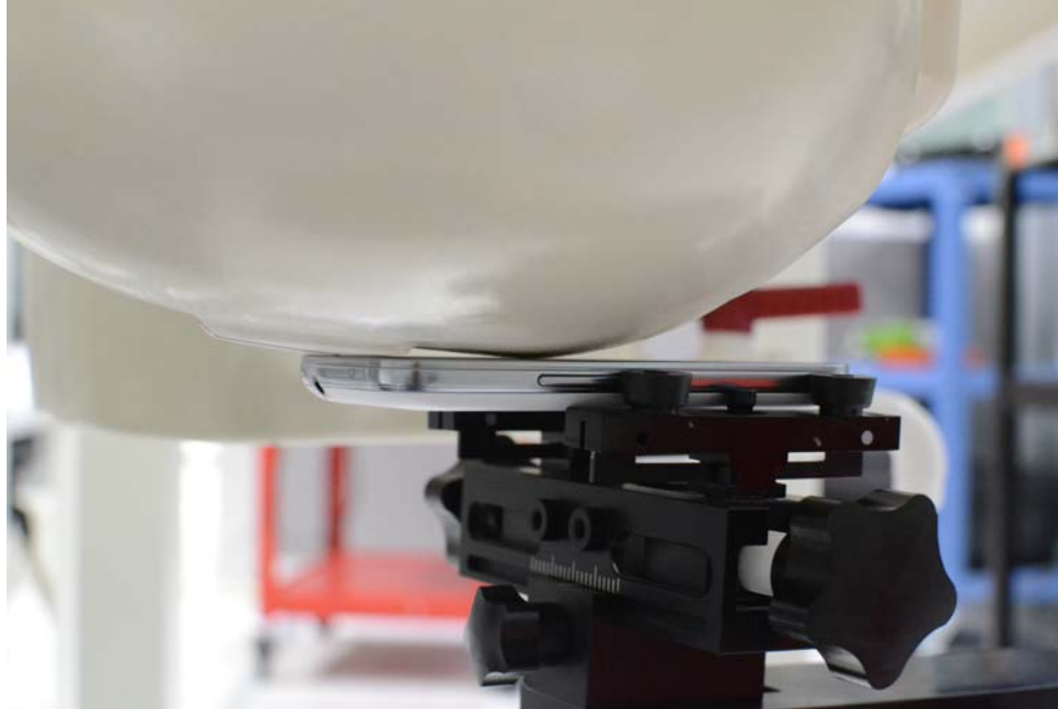
SAR Test Setup Photo 1: Right Cheek
