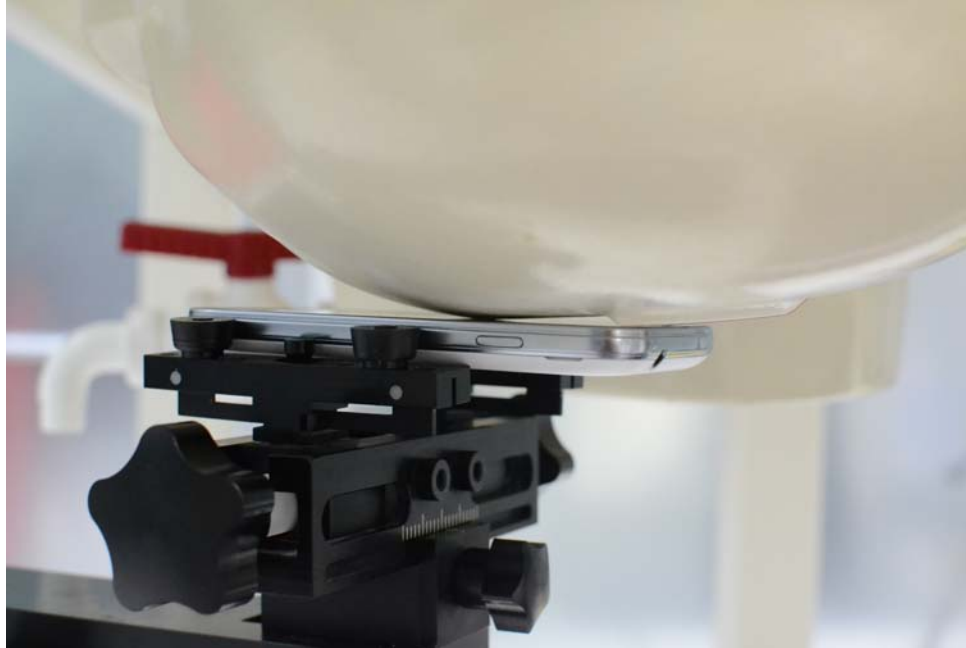
SAR Test Setup Photo 3: Left Cheek
