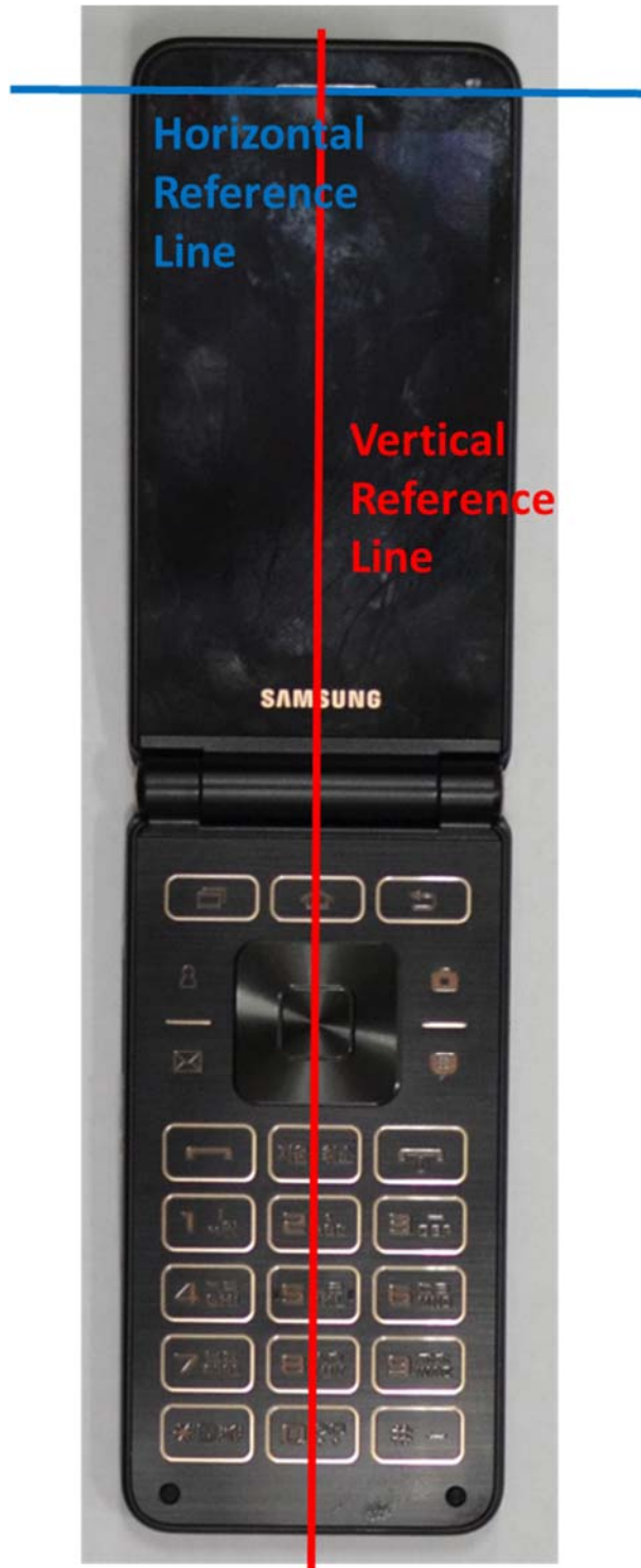
SAR Test Setup Photo 10 – Vertical and Horizontal Reference Lines
