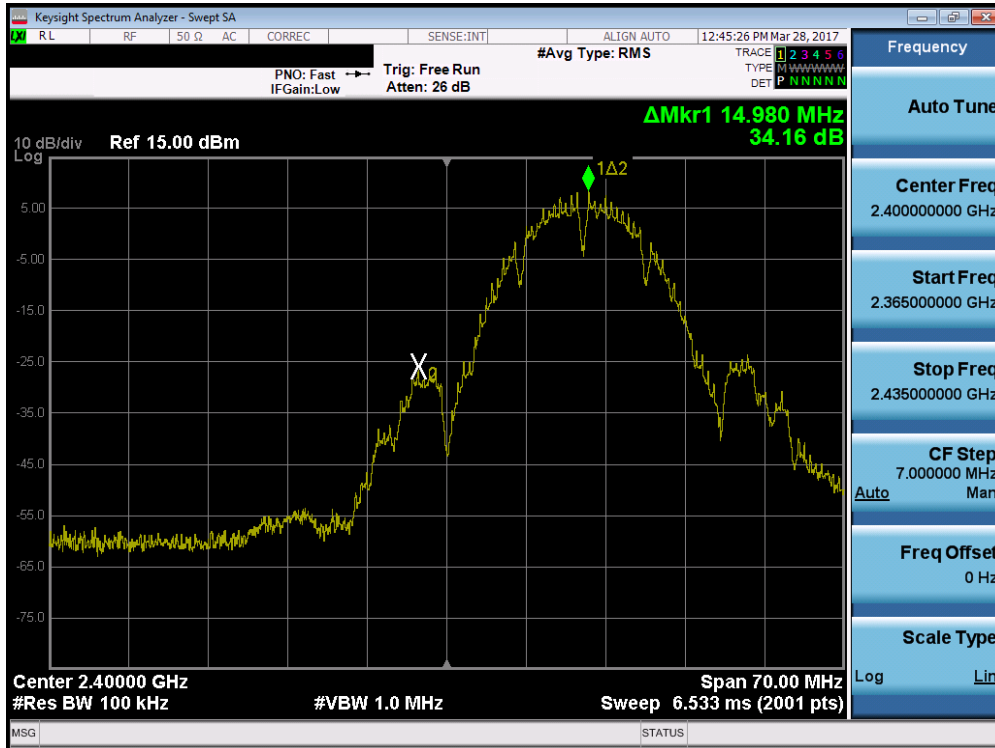
Plot 7-19. Band Edge Plot (802.11b – Ch. 1)
