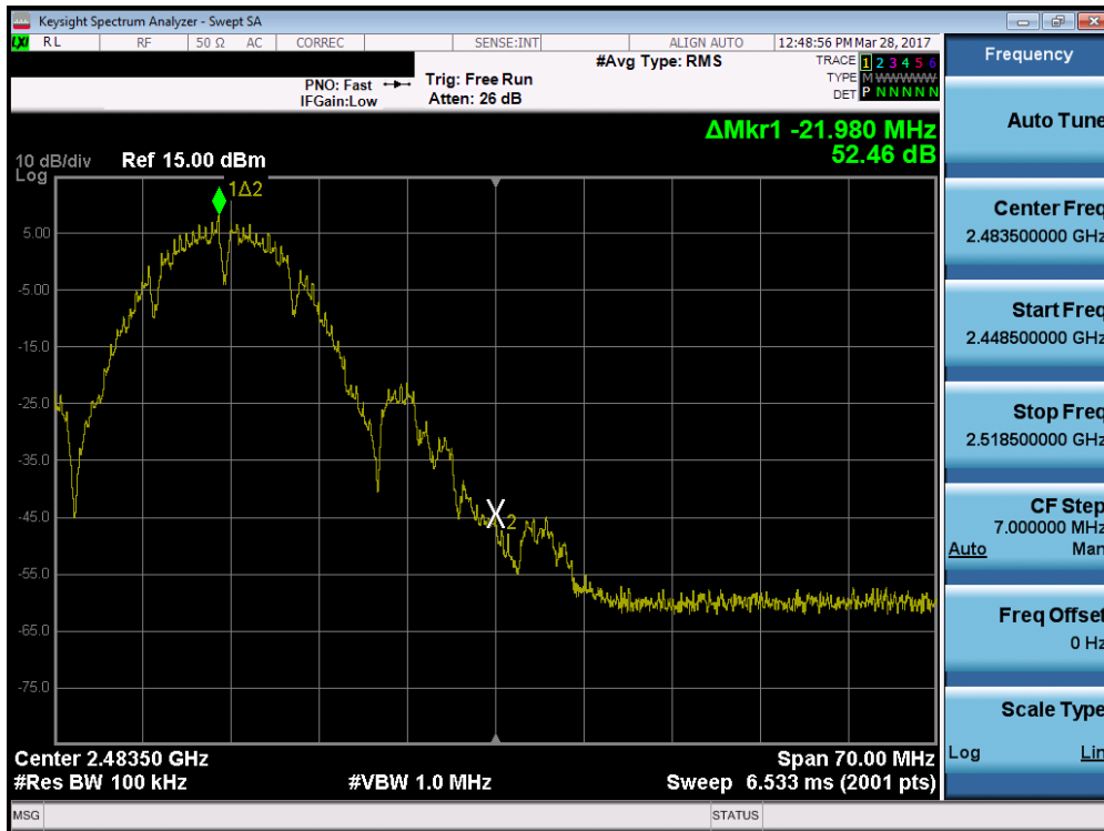
Plot 7-20. Band Edge Plot (802.11b – Ch. 11)
