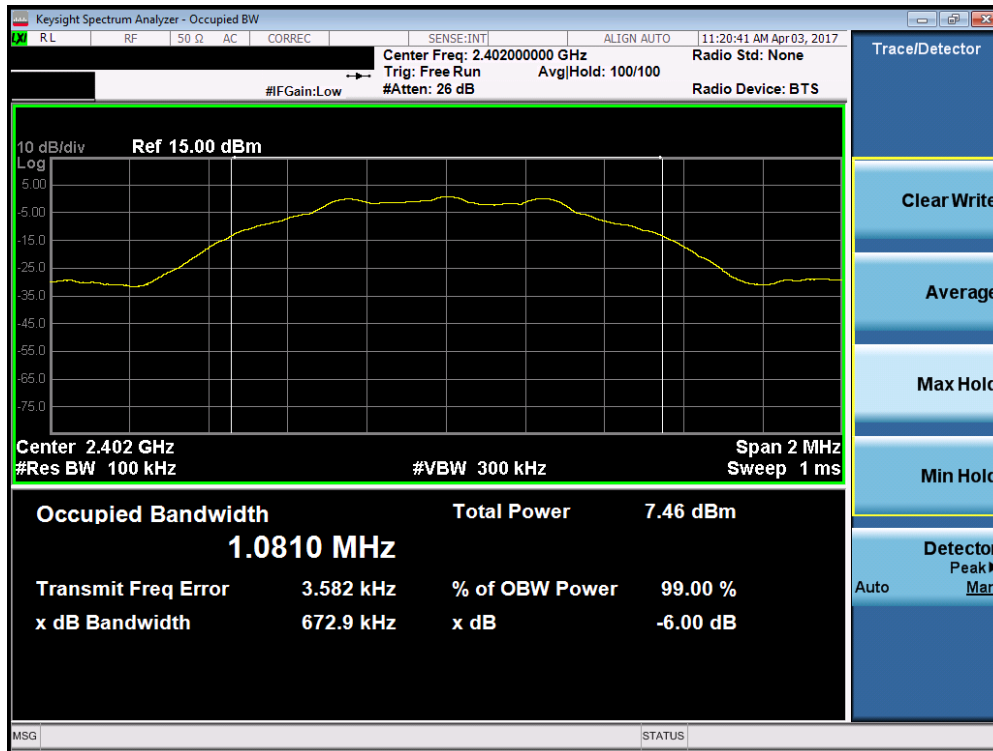
Plot 7-1. 6dB Bandwidth Plot (Bluetooth (LE) – Ch. 0)
