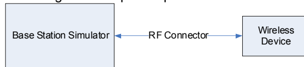
Figure 9-2 Power Measurement Setup
